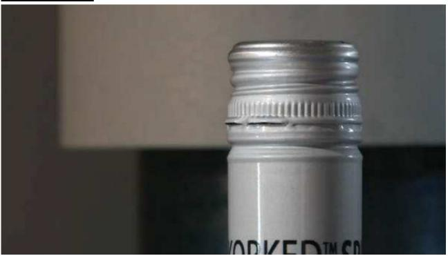
The aluminium between screw cap's bridges tends to deform or flanging in consequence of the following causes:
