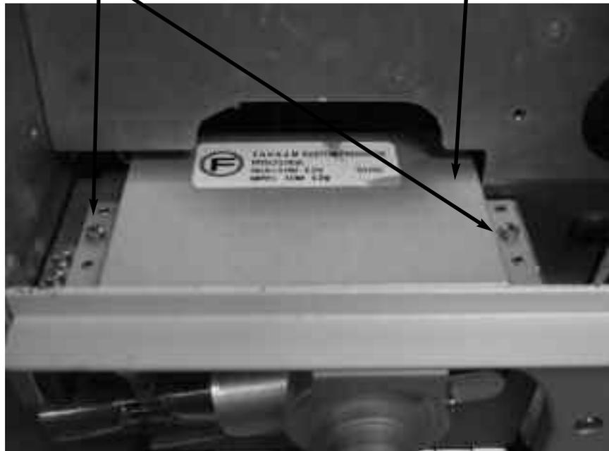
**Figure 4-22 Heater Assembly HTR2100A**
