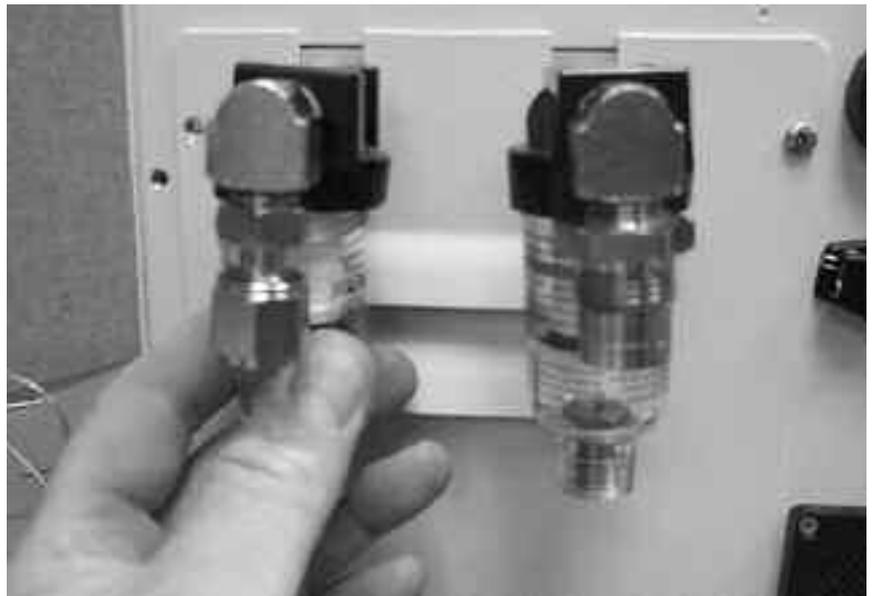
**Figure 2-1 Inlet Water Trap Filter Replacement**
