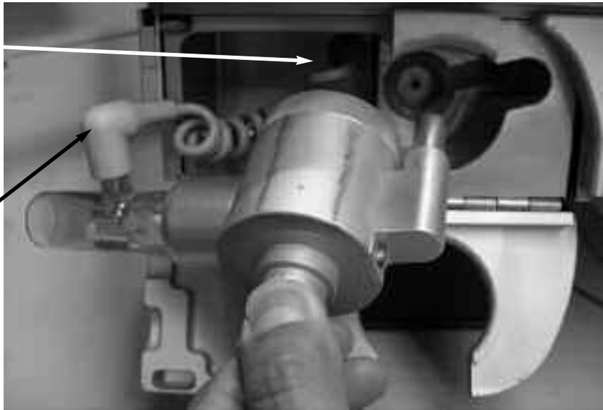
**Figure 4-1 Exhalation Valve and Exhalation Flow Sensor**
