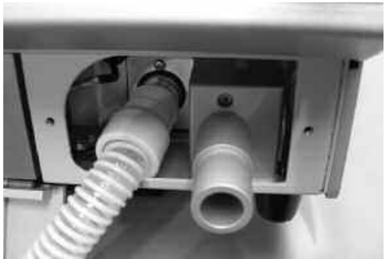
**Figure 4-19 Use circuit to loosen Oxygen Sensor**
