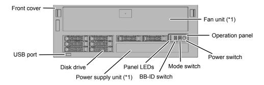
\*1: You can see the fan unit and the power unit by removing the front cover.
