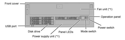
\*1: You can see the fan unit and the power supply unit by removing the front cover.
