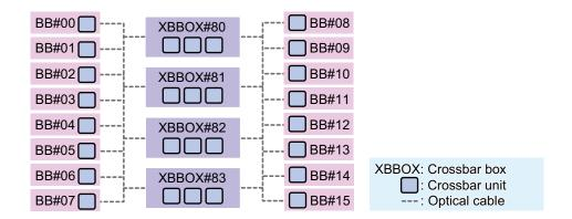
Each number shown after BB# or XBBOX# is an ID (BB-ID) used for identification. Building block numbering begins with 00, and crossbar box numbering begins with 80. For the connection procedure, see the *Fujitsu M10/SPARC M10 Systems Installation Guide*.
