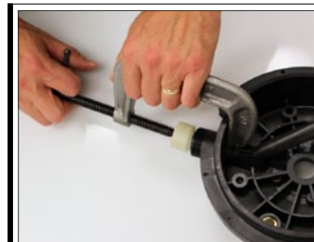
Fig. 16a | Use Bulkhead Inserter tool to install new bulkhead insert.
