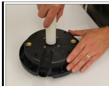
Fig. 27b | On a flat surface, use the Seal Seat Driver tool (wide end) to install the seat into the motor base plate counter bore with the smooth shiny surface facing up.
