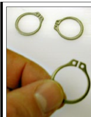
Fig. 3b | Retaining rings have a smooth rounded edge on one side, sharp on the other.
