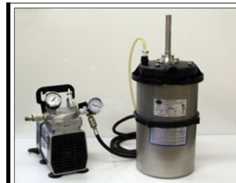
Fig. 35b | Draw motor base plate assembly into S/S housing using 20 in. Hg of Vacuum.
