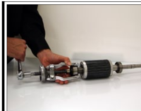
Fig. 17a | Use bearing puller to remove damaged bearings.
