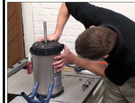
Fig. 21b | Lower motor/motor base plate assembly into S/S housing and be sure it is even/square on the housing.
