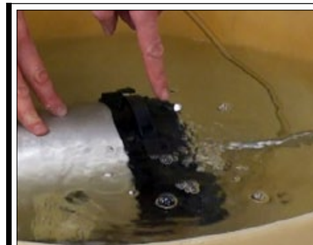
Fig. 37b | Water dunk tank works well for testing leakage, you can also use a soapy water solution.
