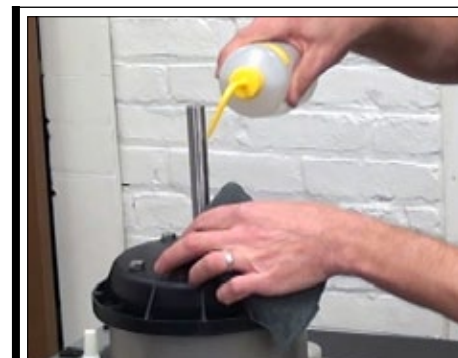
Fig. 34b | Clean motor shaft with denatured alcohol.
