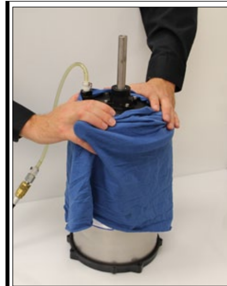
Fig. 3a | When removing motor base plate with air pressure, wrap a rag around the assembly to catch excess oil.
