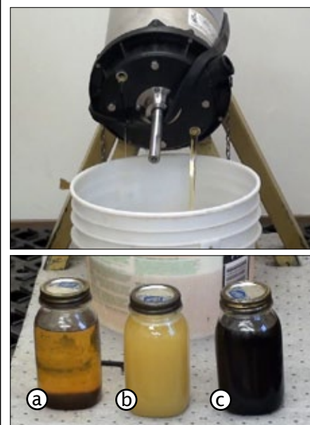
Fig. 1c | [Top] Remove oil plugs and drain oil, note condition of oil. [Bottom] Condition of oil: (a) Clean Oil (b) Milky Oil (c) Dark Oil
