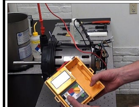
Fig. 8b | Megger and Hi-Pot tests will verify correct wiring and operation. (Megger test shown)
