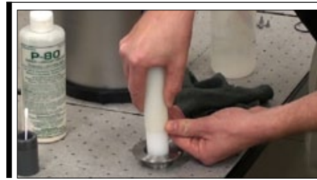
Fig. 14b | Insert into bore of hub with seal surface facing out, push into place with Seal Seat Drive (P/N SS-10)
