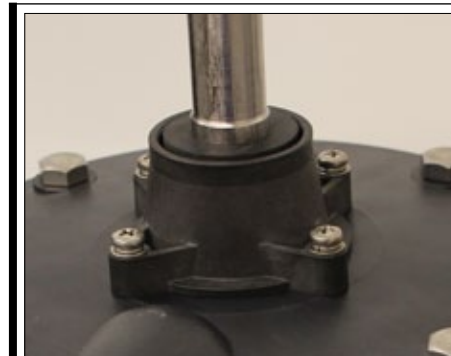
Fig. 26b | Rubber slinger disc is flush to the top of the hub when installed
