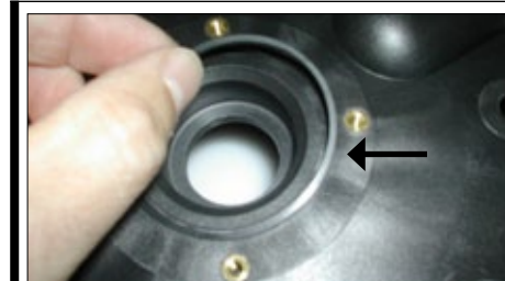
Fig. 15b | Place square ring into groove of motor base plate.
