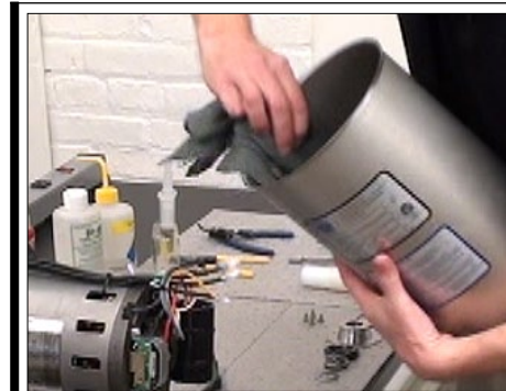
Fig. 32b | Wipe clean the S/S housing before installing motor/motor base plate assembly.
