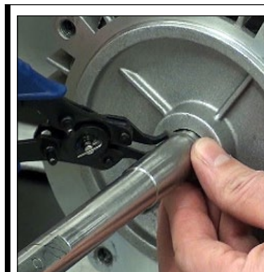
Fig. 2b | Install retaining ring to motor shaft so it locks into groove.
