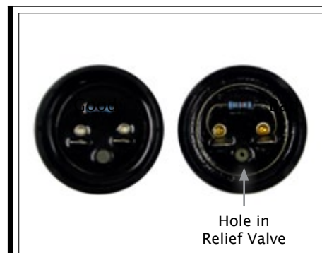
Fig. 10a | Capacitors, hole in relief valve means it's bad and needs to be replaced.
