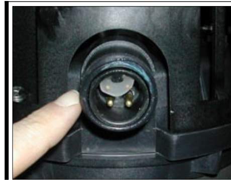
Fig. 41b | Place dielectric compound or silicone grease in the bulkhead connector to prevent water penetration which will lead to nuisance tripping.
