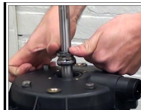
Fig. 12b | When seal reaches shoulder of shaft, place thumb tips on outer edge
