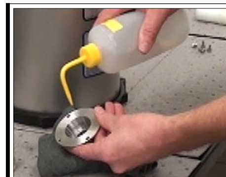
Fig. 13b | Clean inside of S/S Hub (P/N 42-0052 with denatured alcohol)
