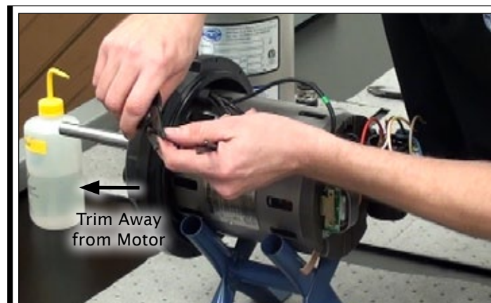
Fig. 30b | When trimming bulkhead wires be sure to trim away from the top of the motor so the scrap doesn't fall in the windings.
