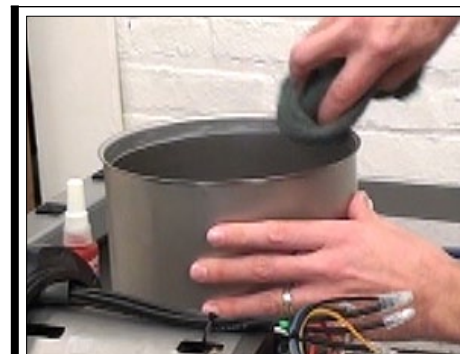
Fig. 10b | Wipe seal lubricant around the top of the S/S housing to help with seating the motor/motor base plate assembly.
