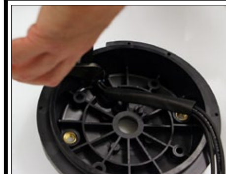
Fig. 14a | Remove old bulkhead insert. Cut away part of lip if necessary.
