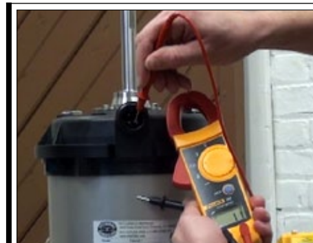
Fig. 38b | Check for continuity between S/S housing and ground pin on bulkhead to confirm that S/S housing and ground clip are touching.
