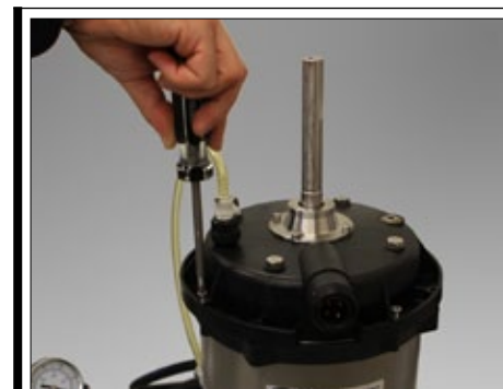
Fig. 36b | Insert self tapping screws into motor base plate and lift can ring. Thread by hand and tighten screws.
