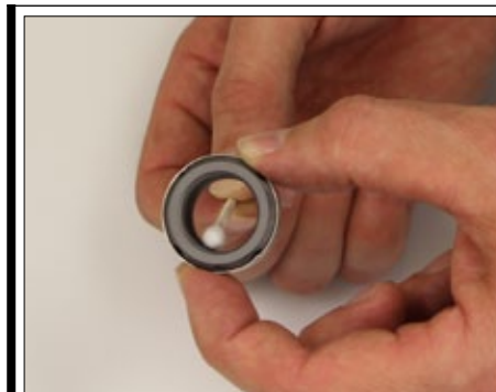
Fig. 23b | Apply seal lubricant to inside of rotary portion of the seal with cotton swab.
