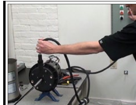
Fig. 9b | Bump start the motor to verify wiring and operation.
