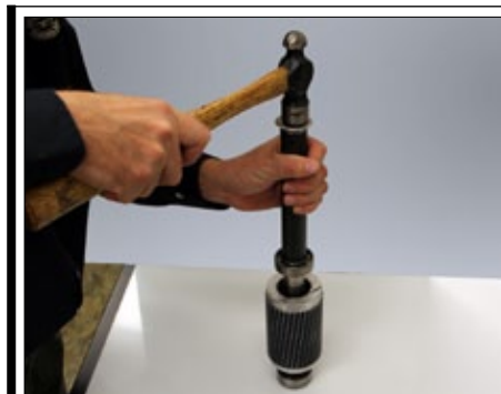
Fig. 18a | Tap new bearings into place with the Bearing Driver tool.
