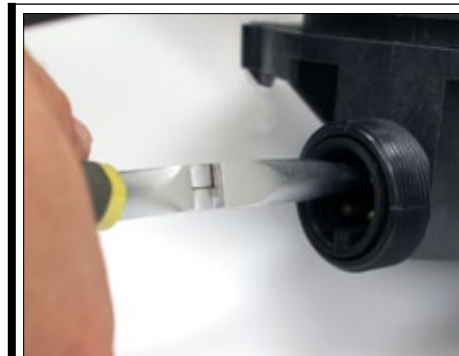
Fig. 15a | Use needle nose pliers to grab pin and remove insert.
