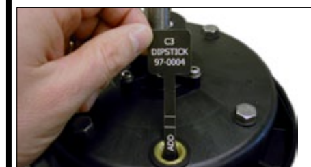
Fig. 39b | (Top) Pour Otterbine oil into one of the oil plug openings on the power unit using a funnel. (Bottom) Fill until oil level is between the lines of the C3 Oil Dipstick.
