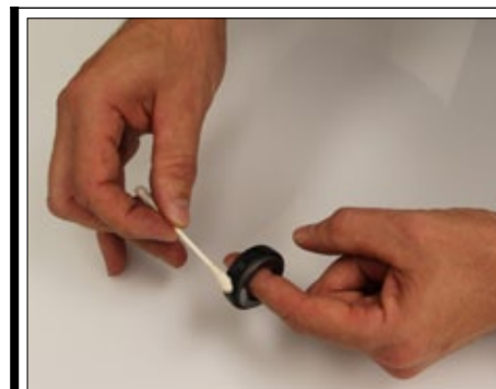
Fig. 17b | Apply seal lubricant to the outer rubber surface of the Silicon Carbide Seal Seat.
