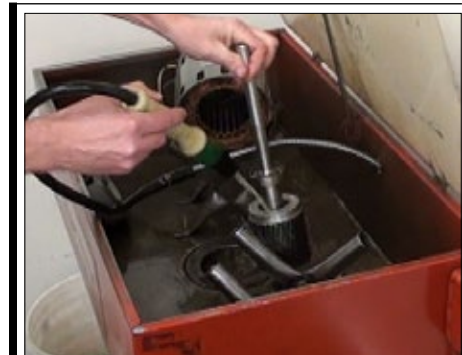
Fig. 7a | If water was present in oil, you might be able to reuse motor. Separate motor rotor and stator and wash both in mineral spirits; allow to dry overnight before retesting.
