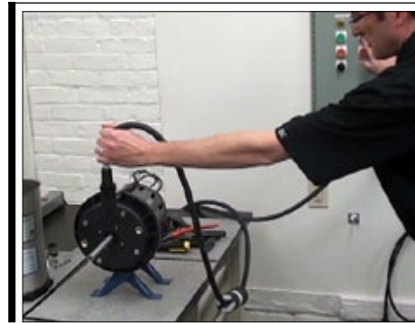
Fig. 31b | Bump start the motor to verify wiring and operation.
