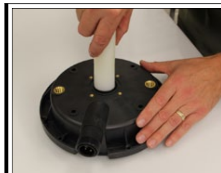
Fig. 18b | On a flat surface, use the Seal Seat Driver tool (wide end) to install the seat into the motor base plate counter bore with the smooth shiny surface facing up.
