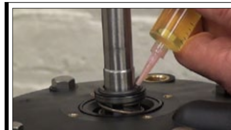
Fig. 16b | Apply two drops of Otterbine oil onto the face of the seal seat.
