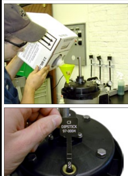
Fig. 2c | [Top] Pour Otterbine oil into one of the oil plug openings on the power unit using a funnel. [Bottom] Fill until oil level is between the lines of the C3 Oil Dipstick.
