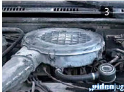
Fig : Cleaning of air filter housing
