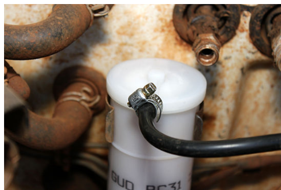
Fig: Photographs of Replacing Fuel Filter
