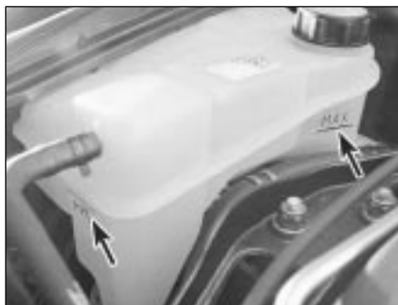
3.10 The cooling system expansion tank is located on the right-hand side of the engine compartment. The coolant level must be between the tank "MAX" and "MIN" level lines (arrowed) when the engine is cold
