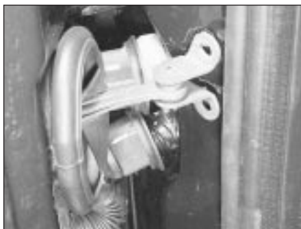
15.2B Front door check strap removed
