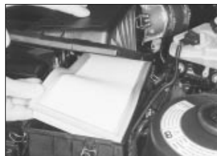
29.2 . . . lift the element out of the housing, and wipe out its interior before fitting the new element
