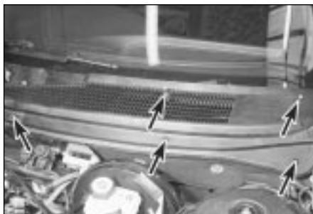
27.3 Remove screws (arrowed) to release cowl grille panel . . .
