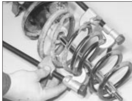
12.1E . . . and coil spring
