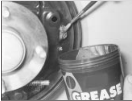
6.2N Clean the backplate, and apply small amounts of high-melting-point brake grease to the brake shoe contact points. Be careful not to get grease on any friction surfaces
