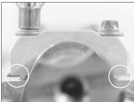
13.21A Keep caps square to cylinder head at all times when tightening down
