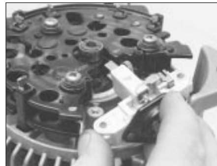
13.4 . . . then remove regulator/brush holder assembly (secured by two screws)
