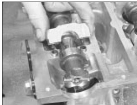
13.5A Note locating dowels when removing camshaft bearing caps
