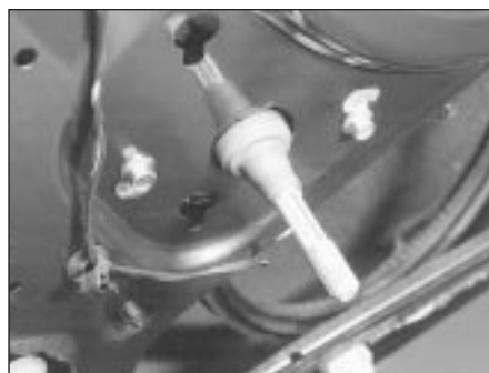
13.2D Manual winder mounting bolts (rear door)
