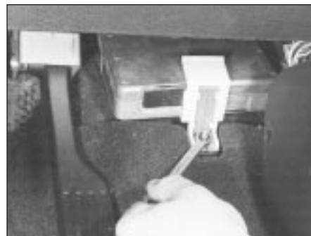
4.37 Unscrew retaining bolt and withdraw ECU's mounting bracket . . .
