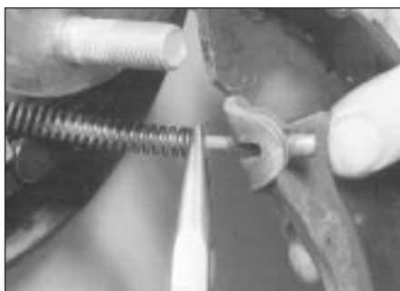
6.2K Pull the handbrake cable spring back from the operating lever on the rear of the trailing shoe. Unhook the cable end from the cut-out in the lever, and remove the shoe
