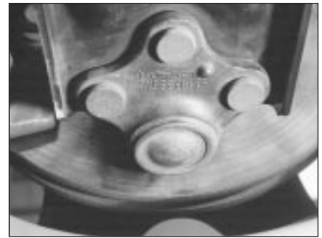
8.0 Original riveted front suspension lower arm balljoint
