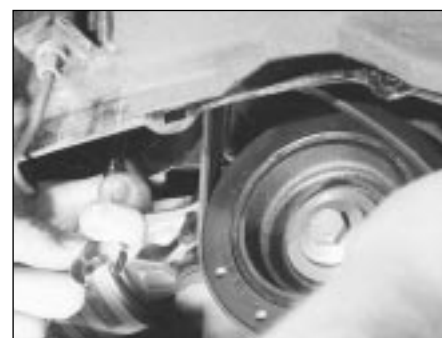
11.9 Rotate the tensioner pulley clockwise to release its pressure on the drivebelt, then slip the drivebelt off the crankshaft pulley
