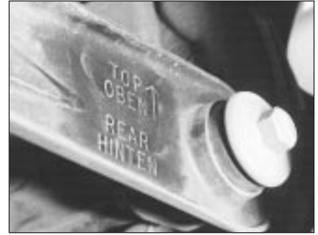
14.11 "TOP" marking on the rear lower arm
