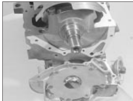
16.12 Use new gasket when refitting oil pump
