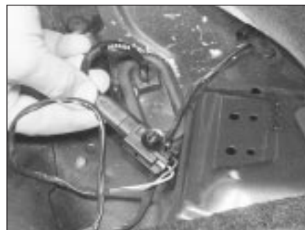
21.12 Rear ABS sensor wiring multi-plug located beneath the rear seat
