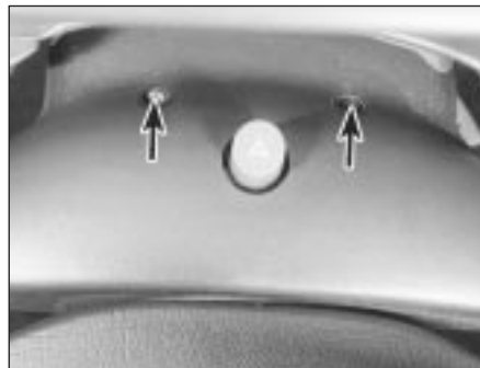
28.4D Upper shroud retaining screws (arrowed)
