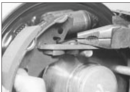
6.2H Unhook the upper return spring from the shoes . . .
