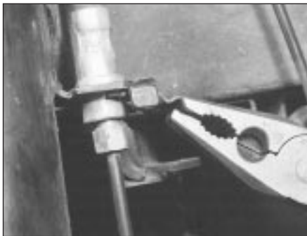
14.6B Pulling out a brake pipe mounting clip
