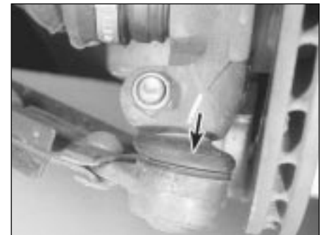
19.2B Check the condition of the lower arm balljoint dust cover (arrowed)
