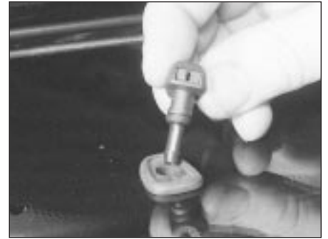
22.12A Remove the nozzle from the tailgate glass . . .
