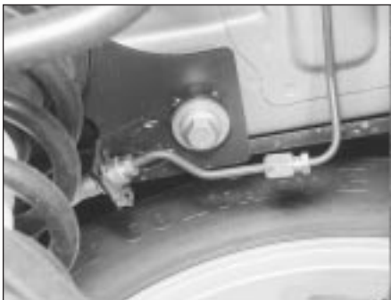
26.7A Rear suspension crossmember rear mounting bolt
