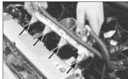
16.19B . . . and withdraw fuel rail with injectors and pressure regulator - renew nose seals (arrowed) whenever rail is disturbed
