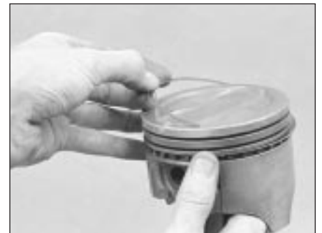
16.7A Installing the spacer/expander in the oil control ring groove
