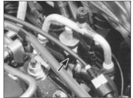
12.33 Unplug pressure-regulating switch electrical connector (arrowed)
