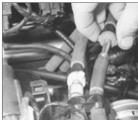
4.7 Note colour-coding of unions when disconnecting fuel feed and return lines
