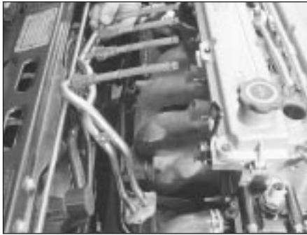
7.23 Removing pulse-air piping - take care not to bend or distort it
