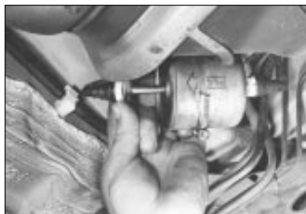
33.5 Squeeze together fuel filter pipe union locking lugs, then pull pipes off filter stubs - ensure pipes are correctly reconnected
