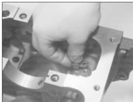
11.1E . . . unbolt blanking plugs (where fitted) to clean out oilways . . .
