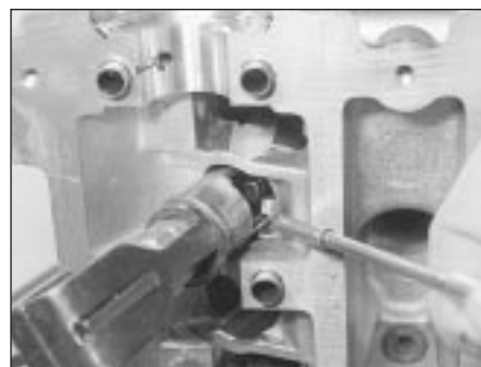
6.3C . . . so that both valve split collets can be removed from the valve's stem - small magnetic pick-up tool prevents loss of small metal components on removal and refitting
