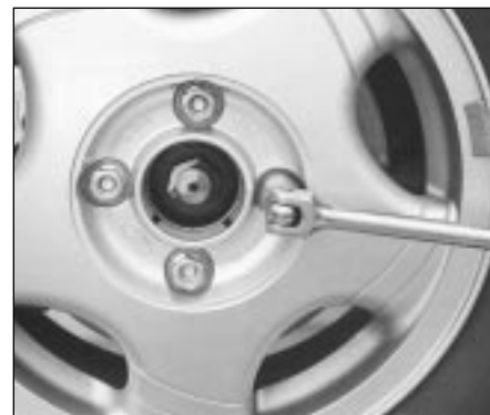
Slacken roadwheel nuts in diagonal sequence
