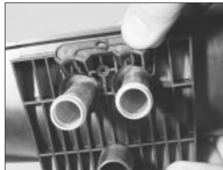
9.14 Remove clamp (one screw) to separate matrix from heater unit's bottom cover
