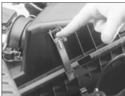
29.1B . . . noting the long clip normally hidden by the battery . . .
