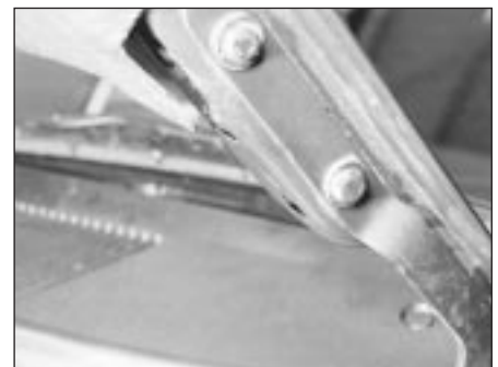
8.7 Mark around the bonnet hinges with a soft pencil before removal
