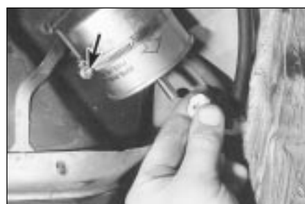
33.7B . . . secure pipe unions as described - do not overtighten clamp screw (arrowed)
