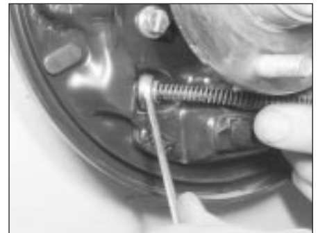
27.8 Using a ring spanner to compress the retaining lugs securing the outer cable to the backplate
