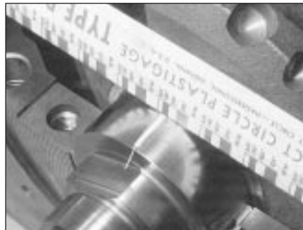
17.10 Compare the width of the crushed Plastigage to the scale on the envelope to determine the main bearing oil clearance (always take the measurement at the widest point of the Plastigage). Be sure to use the correct scale; Imperial and metric scales are included
