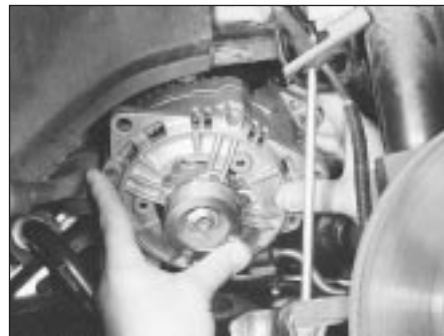
12.6 Alternator must be withdrawn through right-hand front wheel arch
