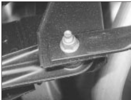
23.2 Front lower arm-to-crossmember securing bolt
