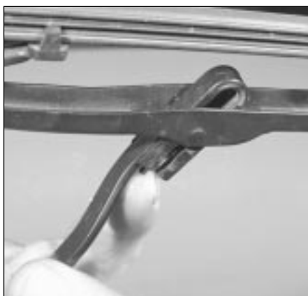
6.6 Releasing the catch to remove a windscreen wiper blade
