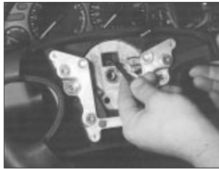
27.7 Feeding the horn and air bag wiring through the hole in the steering wheel hub
