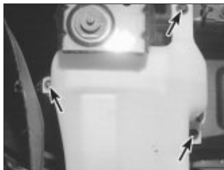
22.2 Washer reservoir mounting bolts (arrowed)
