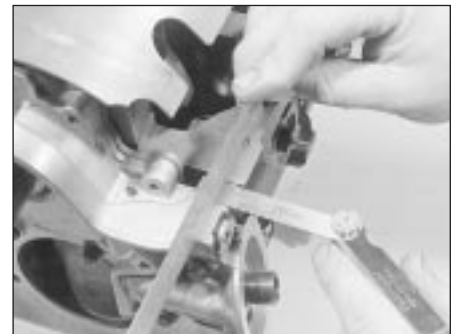
16.13 Check the oil pump is positioned correctly
