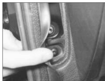
33.18B ... and pull away the weatherstrip to reveal the facia mounting bolts
