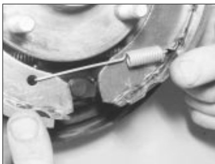
6.2E Release the trailing (rear) brake shoe from the anchor, then move the bottom ends of both shoes towards each other
