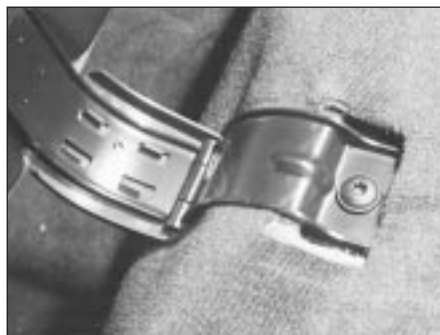
27.6 Rear seat cushion hinge bolt
