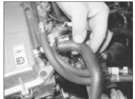
5.4 Disconnecting crankcase breather hose from cylinder head cover union
