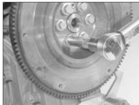
21.11 Note method used to lock flywheel/driveplate while (new) bolts are tightened
