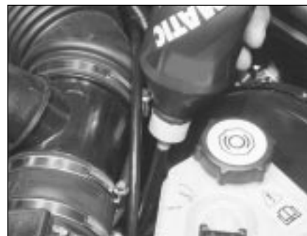
7.6B Adding automatic transmission fluid through the dipstick tube
