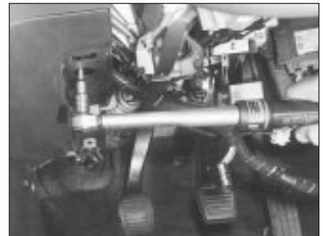
28.13 Tightening the steering column mounting bolts
