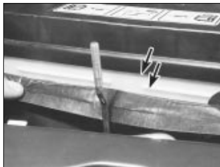
3.18 On non-sealed batteries, keep the electrolyte level of all the cells in the battery between the maximum and minimum levels (arrowed) - ie, 10 mm above the plates. Use only distilled water, and never overfill
