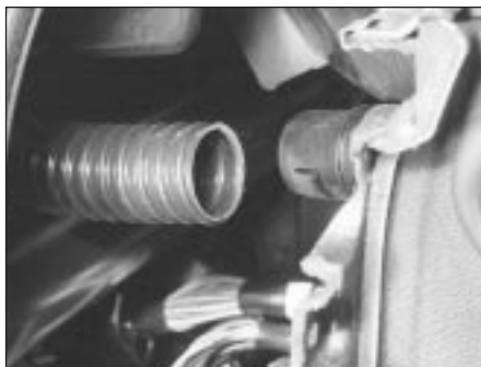
33.22 Disconnecting the fresh air hoses
