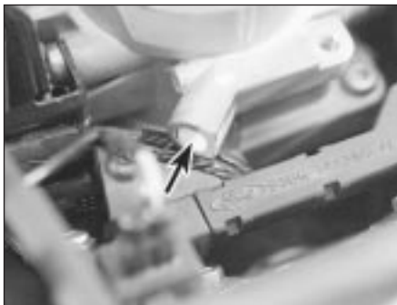
3.45 Throttle housing air bypass screw is sealed on production with a white tamperproof plug (arrowed)
