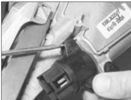
4.4A Release the retaining tab . . .
