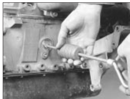
11.4 The core plugs should be removed with a puller - if they're driven into the block, they may be impossible to retrieve
