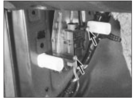
13.3 Fuel cut-off switch retaining screws (arrowed)
