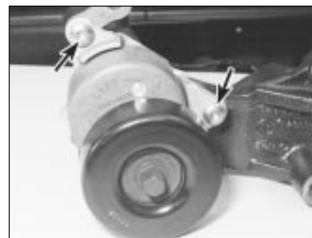
11.6 The auxiliary drivebelt is tensioned by an automatic tensioner; Torx screws (arrowed) secure it to alternator mounting bracket
