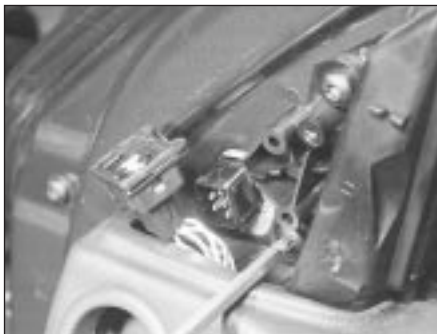
16.5A Unscrew the screws ...
