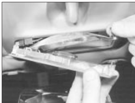
6.5 Lifting the reflector from the interior light
