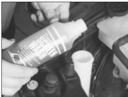
3.17 Topping-up the windscreen washer reservoir
