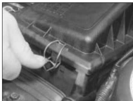
29.1A Release the wire clips to detach the cover from the air cleaner assembly . . .
