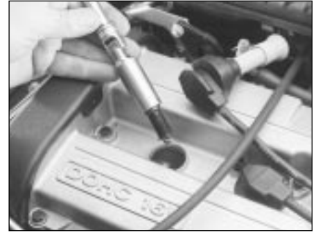
31.16 Spark plugs have tapered seats - do not overtighten them on refitting, or you will not be able to get them out again without risking damage to the plugs and cylinder head
