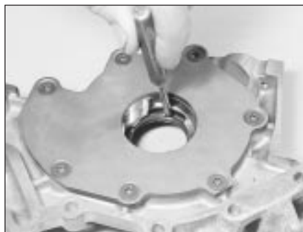
20.2 Driving out crankshaft right-hand oil seal
