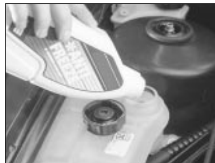
3.13 Remove the cap to add coolant only when the engine is cold - top-up to the "MAX" level line using the specified coolant mixture
