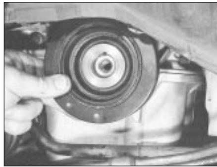
8.4B Ensure pulley is located on crankshaft Woodruff key on reassembly
