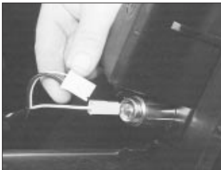
30.8 Disconnecting the cigar lighter wiring
