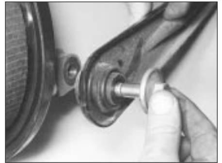
11.9B . . . and remove the rear lower arm from the knuckle
