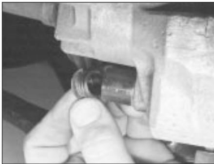
2.3B Pry the plastic covers from the ends of the two guide pins
