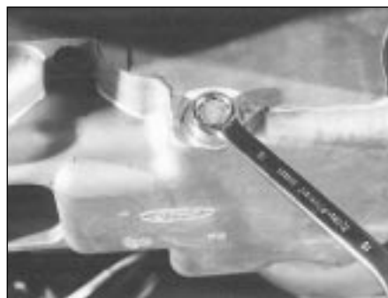
15.7 Use the correct-size spanner or socket to remove the oil drain plug and avoid rounding it off
