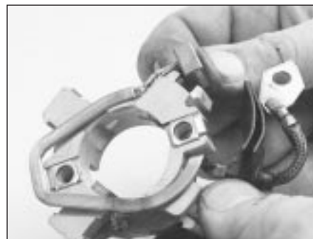
17.2I ... note how the bus bar is engaged on the brushbox before removing it
