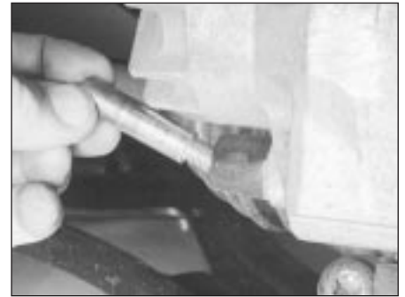
2.3D . . . and remove the guide bolts securing the caliper to the carrier bracket
