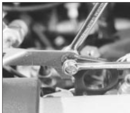
4.9B . . . unbolt the power steering high-pressure pipe . . .
