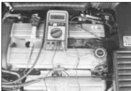
31.22 Measure the resistance of the spark plug leads - if any exceeds the specified maximum value, renew all the leads
