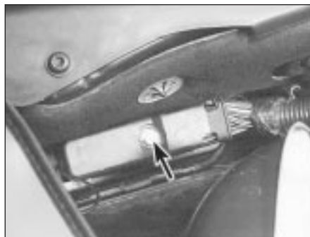
4.36B . . . unscrew bolt (arrowed) to release ECU's electrical connector
