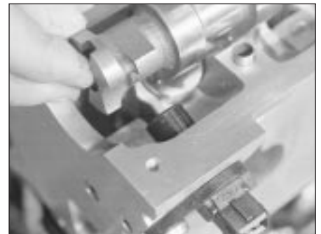
13.5B Inlet camshaft has lobe for camshaft position sensor
