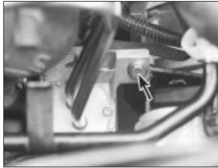
7.31 Remove mounting bolt (arrowed) to remove complete pulse-air assembly - again, take care not to bend or distort piping
