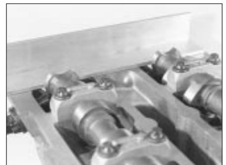
13.21C Fit camshaft aligning tool to set TDC position . . .
