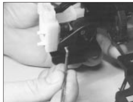
14.10 Pulling out the handle connecting rods
