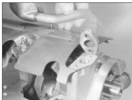
16.16 Use new gasket when refitting oil pick-up pipe to pump
