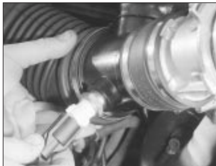
4.7 Unplugging intake air temperature sensor's electrical connector
