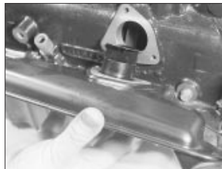
11.1C . . . unbolt crankcase ventilation system oil separator . . .
