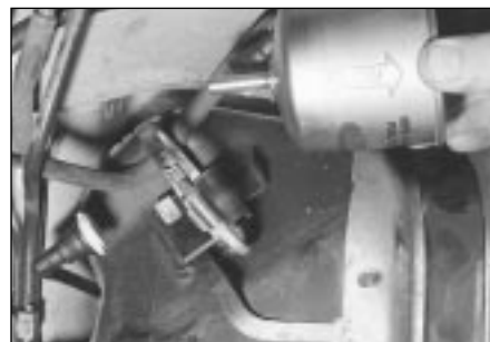
33.7A When installing the new filter, ensure the arrow showing direction of fuel flow points towards the engine . . .
