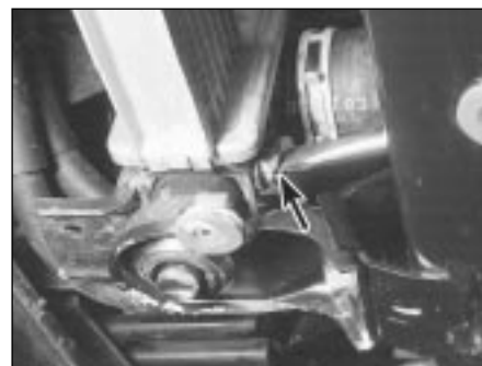
28.3B . . . to unscrew the radiator drain plug (arrowed) and empty the cooling system. Try to protect yourself from coolant splashing into your eyes or onto your skin, catching as much of it as possible in the drain tray
