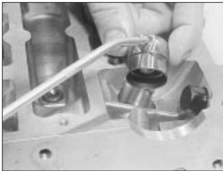
13.17 Oil liberally when refitting hydraulic tappets
