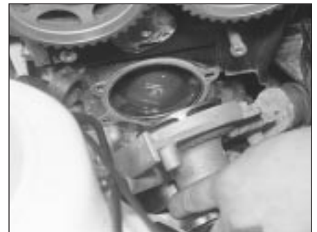
8.10 . . . to remove water pump - always renew gasket and clean all mating surfaces carefully
