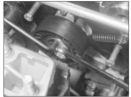
10.20 . . . then use Allen key to position tensioner so that timing belt can be refitted
