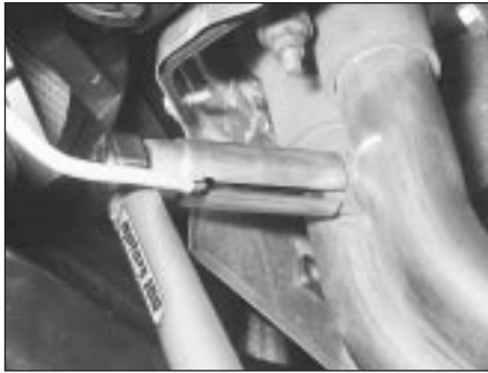
4.64 . . . slotted socket will be required to tighten sensor with a torque wrench
