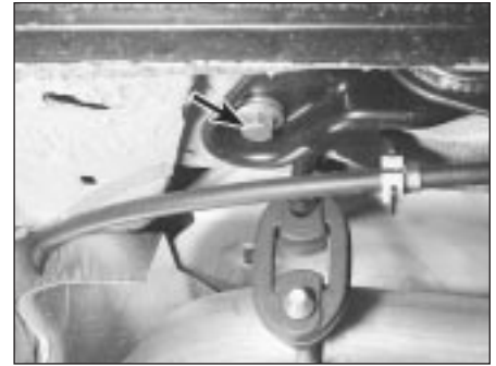
25.8B Tie-bar bracket rear bolt (arrowed) on the underbody
