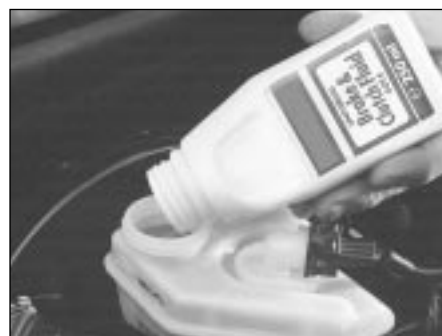
3.22 Topping-up the brake fluid reservoir
