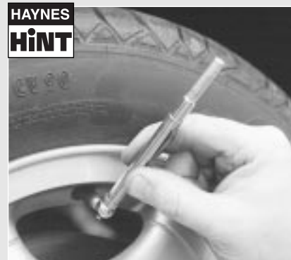
4.2B A tyre tread depth indicator should be used to monitor tyre wear - they are available at accessory shops and service stations, and cost very little
