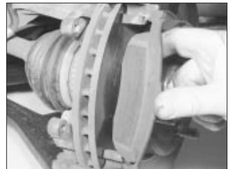
2.3G Remove the outer pad from the caliper frame. Brush all dust and dirt from the caliper, pads and disc, but do not inhale it, as it may be harmful to health. Scrape any corrosion from the disc.
