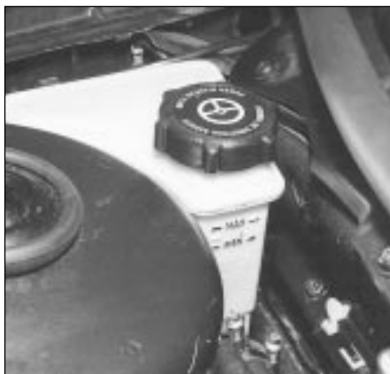
5.4 Power steering fluid reservoir, showing "MAX" and "MIN" marks
