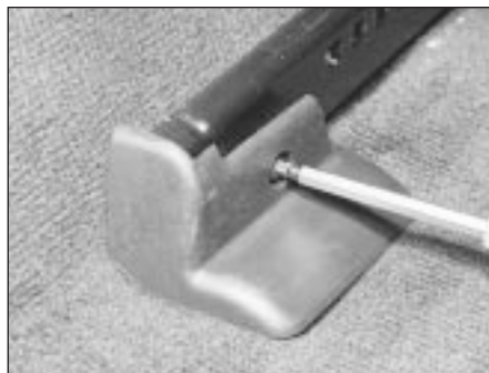
27.2A Unscrew the Torx-headed screws . . .
