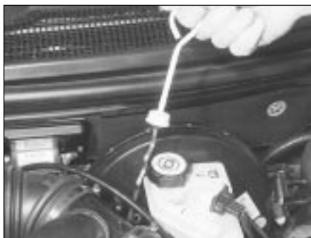
7.4 Removing the automatic transmission dipstick from its tube
