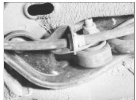
15.4 Tie-bar bracket on the underbody
