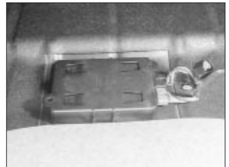
1.6B Adaptive damping computer module located in the luggage compartment
