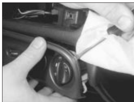
4.10 Prising out the light switch
