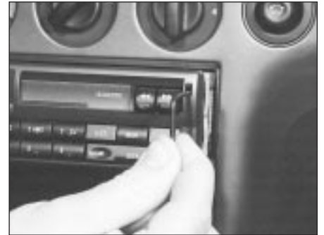
23.6 Using the special U-shaped rods to remove the radio
