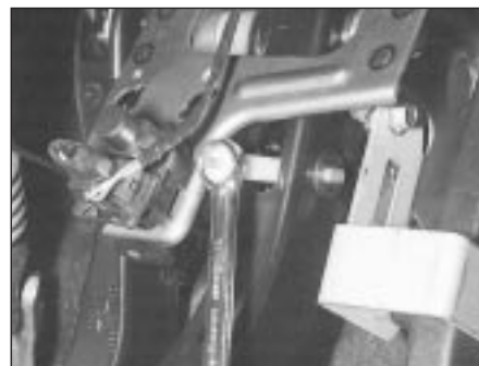
12.4A Unscrew the nut securing the pedal trunnion to the pushrod . . .
