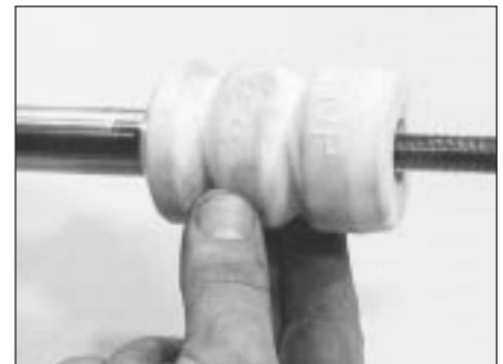
5.5D Removing the bump stop
