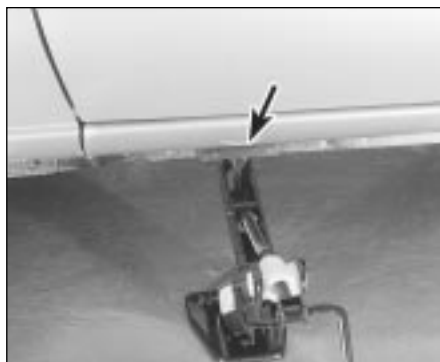
With jack base on firm ground, locate jack head in jacking point - indentations (arrowed) in sill identify jacking points
