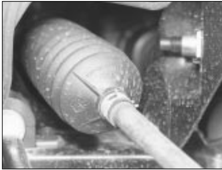
19.2C Check the condition of the steering rack gaiters
