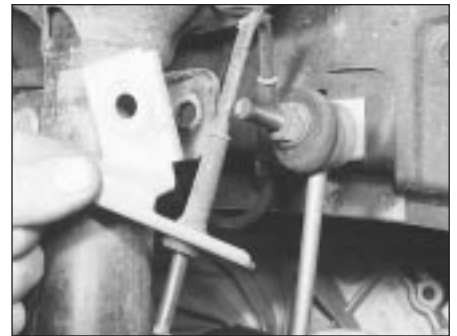
6.2B . . . and disconnect the anti-roll bar link and (on ABS models) the sensor wiring support bracket
