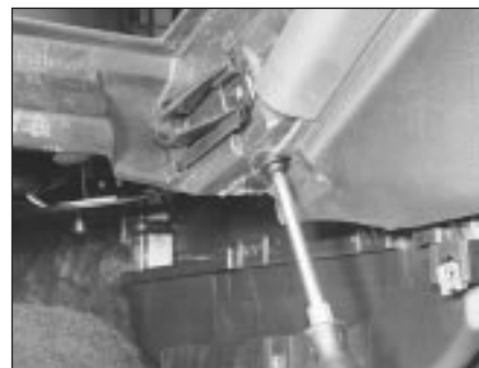
33.20D Facia mounting bolt near the heater
