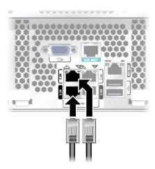
2. Connect Category 5 (or better) cables from your network switch or hub to the remaining Ethernet ports (NET 1, NET 2, NET 3), as needed.
