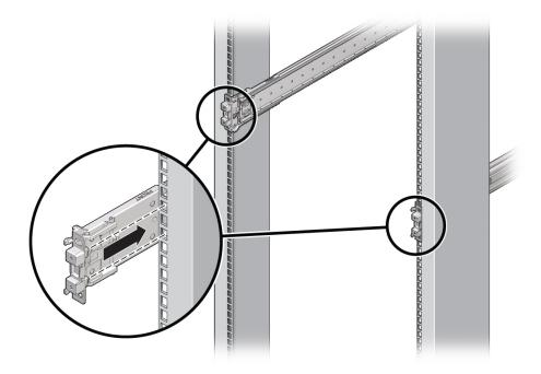
The slide assembly mounting pins accommodate either 9.5 mm square mounting holes or M6 round mounting holes. No other mounting hole sizes are supported.
