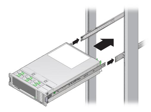
3. Insert the mounting brackets into the slide rails, and then push the server into the rack until the mounting brackets encounter the slide rail stops (approximately 12 inches, or 30 cm).
