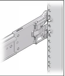
4. (Optional) If you chose to secure the slide rail assembly to the rack with screws, insert the M6 mounting screws through both front and rear slide rail brackets and rack posts, and then secure the screws to the rack posts with the caged nuts.
