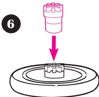
Firmly attach hub adapter onto wheel.
