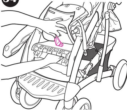
Pull crotch strap up through seat pan, and slide seat cover off backrest.
