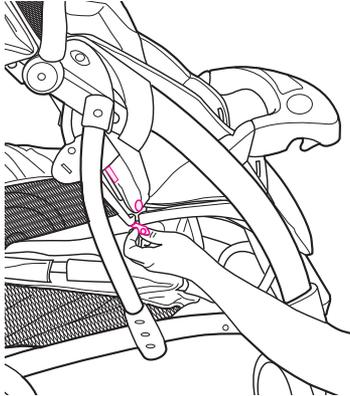
Undo snap and unfasten hook and loop strap on each side of the stroller.
