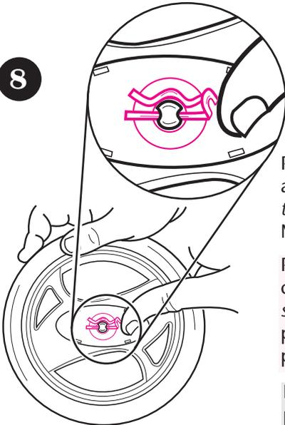
Push straight side of pin through axle hole. Pin will separate around the axle. Curved end of pin MUST face up as shown.
