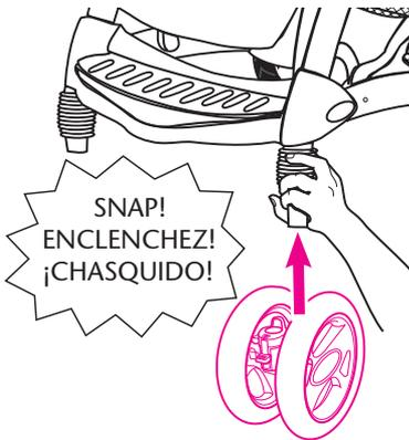
**CHECK** that wheels are securely attached by pulling on wheel assemblies.
