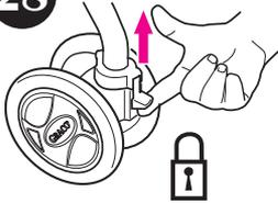
Front swivel wheels lock for use on uneven surfaces such as grass, stones or gravel.
