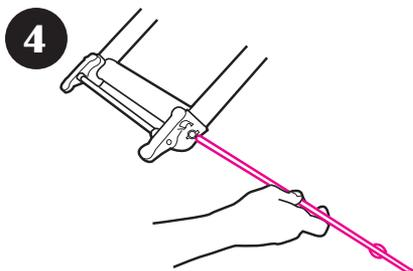
Insert axle rod through axle opening.
