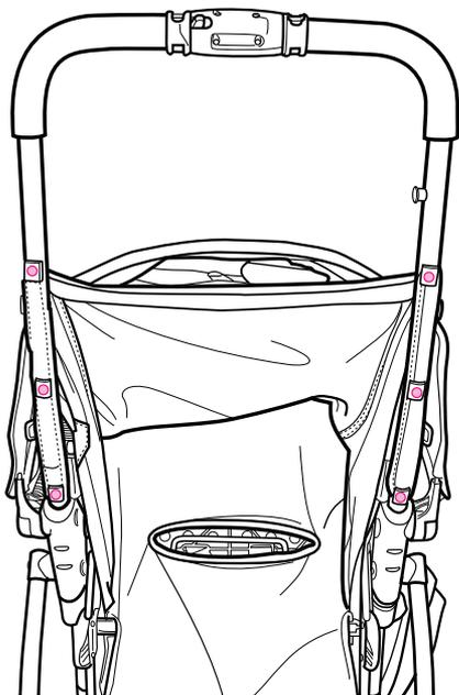
Remove screws from back of seat.
