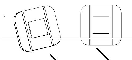
COILS SEATED IMPROPERLY ARE TOO TALL, MAKING INSERTION OF DISH INTO CABINET IMPOSSIBLE
