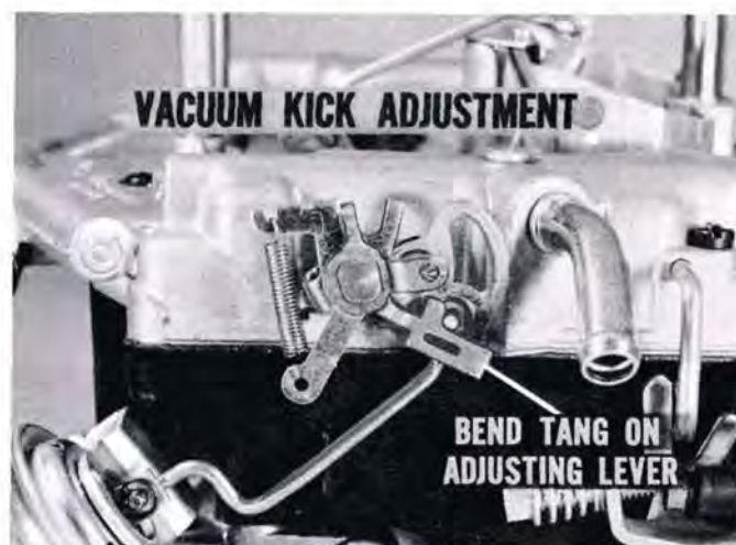
Fig. 25—Tang position determines kick opening
