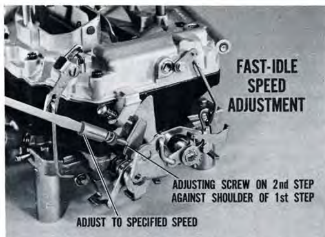
Fig. 31—Warm up engine before adjusting speed
