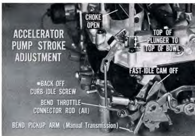
Fig. 20—Check setting with throttle valves closed
