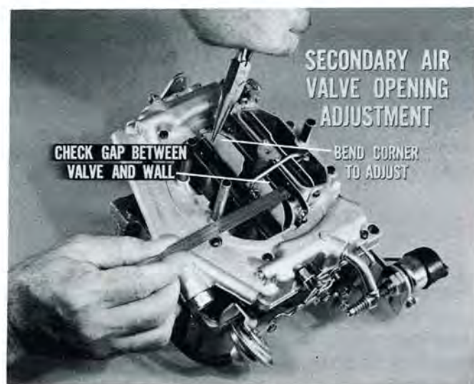
Fig. 18—Hold valve against stop to check opening
