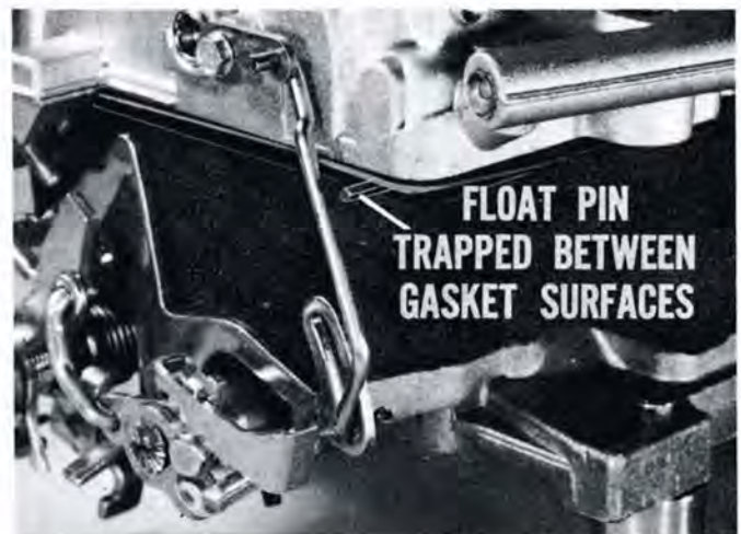
Fig. 36—Float pin can slip out of position
