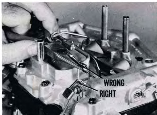
Fig. 12—Wrong link position can cause hangup
