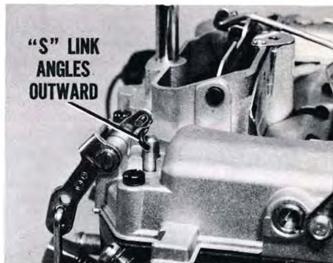
Fig. 10—Over-center action cuts plunger travel
