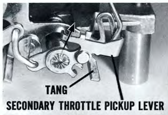
Fig. 4—No secondary operation when choke is on
