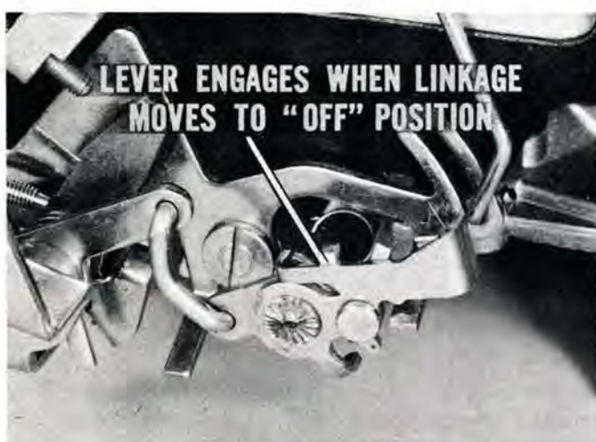
Fig. 5—Lever picks up secondary linkage
