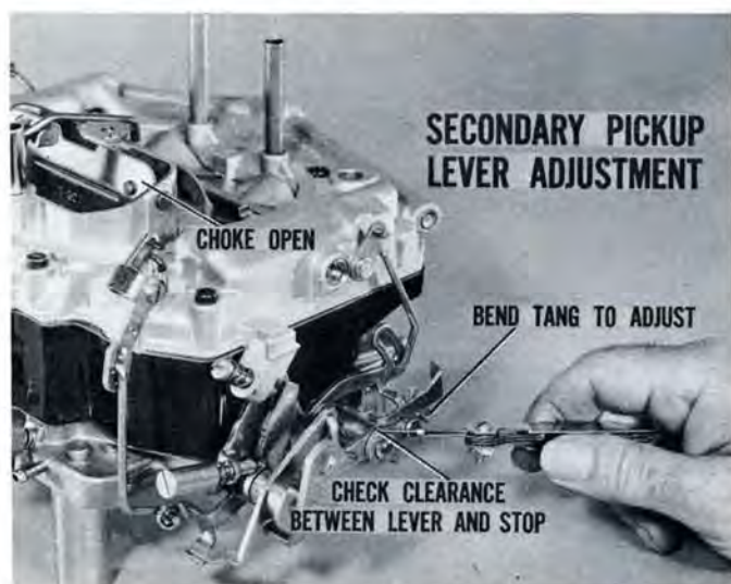
Fig. 30—Lever must clear its stop
