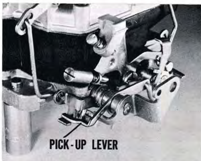
Fig. 11—Staged pump for manual-shift models
