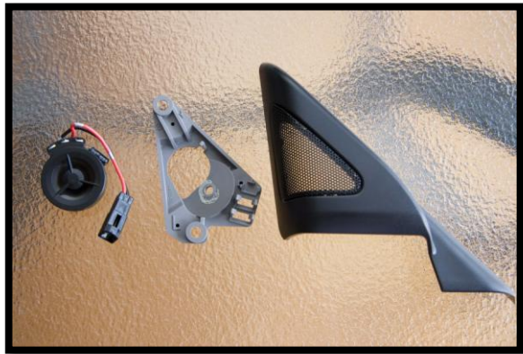
Figure 5 – The factory tweeter assembly consists of three parts; the tweeter itself, the grey mounting bracket, and the black housing.
