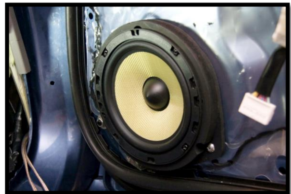
Figure 14 – With the spacer painted, it and the New Woofer can be mounted to the door.
