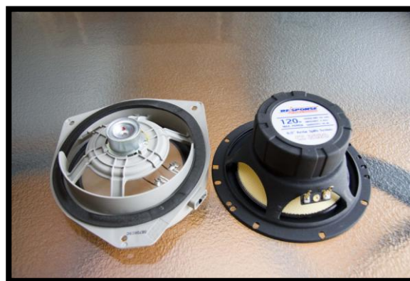
Figure 4 – Compare the size of the magnet in the Factory Woofer (left) and New Woofer (right). The Factory Woofer sounded surprisingly good considering how puny it looks, but was still no comparison to the New Woofer.
