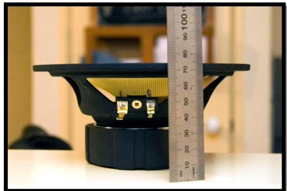
Figure 12 – Measure the depth of your New Woofer to get an idea of how much depth you need in the door. If your Woofers are more than 75mm thick then you will probably need to make thicker spacers than those shown here.
