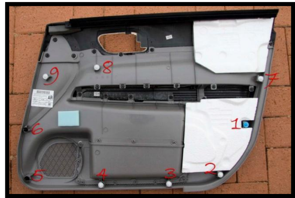
Figure 7 – This photo of the underside of the door skin shows the clips you need to pop off (and the suggested order you should do it in).
