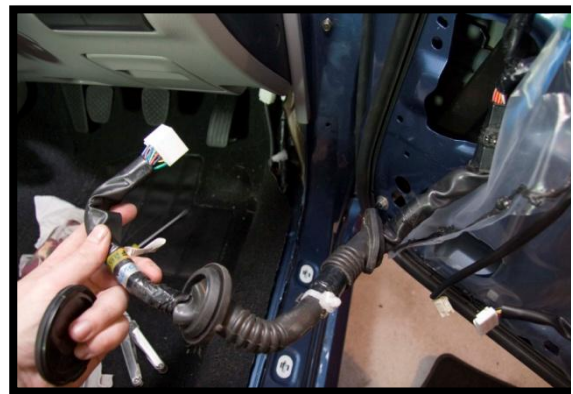
Figure 10 – Feed the connector and loom from the cabin into the door to gain access to it, and then feed the new Speaker Wire through the conduit.
