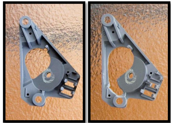
Figure 15 – The original Tweeter mounting bracket (left) and the modified bracket (right).
