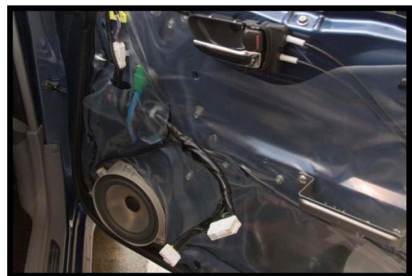
Figure 8 – With the door skin removed, the Factory Woofer can now be easily accessed.
