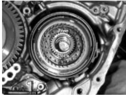
16) Underdrive sprag rotation, drum assembly free-wheels counter clockwise and locks clockwise. This photo also shows the underdrive brake band and the underdrive clutches.
