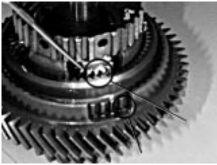
14) Care must be taken when re-assembling the planetaries. This photo shows the retaining ring mis-positioned. The internal ring gear is below the level of the carrier pinions.
