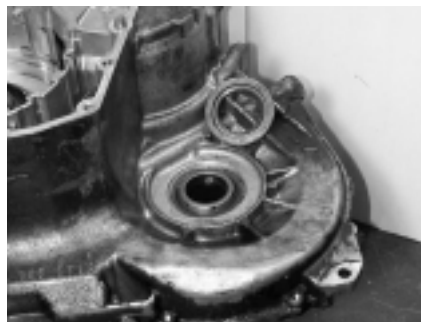
1) The Volvo and Opel versions of this trans use totally different axle seals. The Volvo uses the typical Aisin rubber coated seal, while the Opel seal is similar to the metal clad TH125 axle seals.
