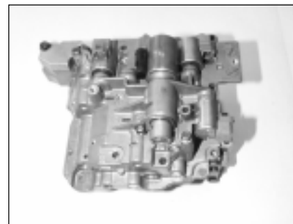
3) Solenoid identification: Top row from left to right: Lock-up solenoid (SL), pressure control solenoid (STH) shift solenoid A (S 1 ). Bottom row left to right: Arrow shows retainer end of the PCS, shift solenoid B (S 2 ).
