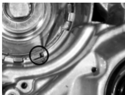
17) Did you think you were through with those #!# "Little" parts? Leave this anti-clunk spring out and you'll be chasing a driveline clunk all day.
