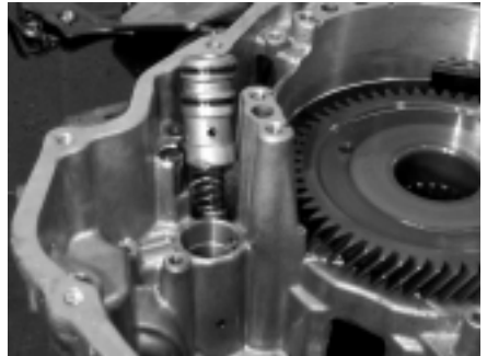
19) The parking pawl assembly plays double duty by also retaining the underdrive brake accumulator assembly. Caution: This is under spring pressure and may very well pop you in the nose.
