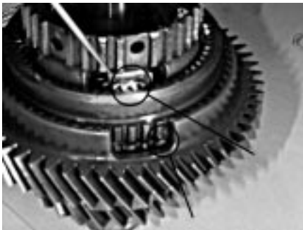
15) This photo shows the planetary retaining ring correctly installed. The internal ring gear is flush with the carrier pinions.
