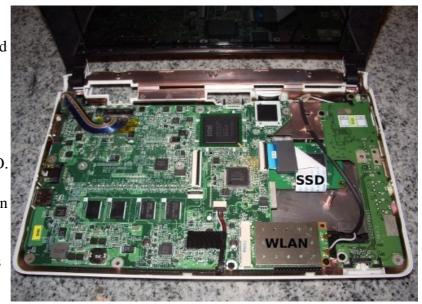
internal SSD seems to have its proprietary connector, so an upgrade is probably not possible. Therefore the cleanest way to expand the AAO is using the SD card slot on the lower left corner of the AAO, it is marked with the text "Storage Extension". Drawbacks are you can not boot from there and AAO Linpus is configured in a way that it automatically writes stuff there.
