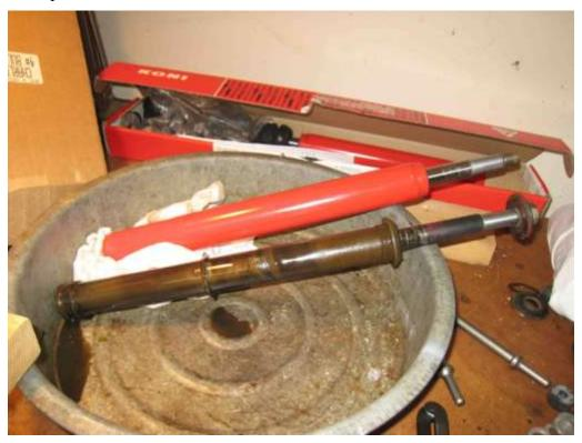
Once the retaining rings were removed the rest of the installation went fairly smoothly. The strut is filled with oil for cooling. I'd read on the Internet where some people put
