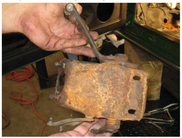
I'd bought a rebuild kit for the assembly, which consists of new brass bushings, springs, nuts, etc. We'll take the assembly apart and rebuild it. The first thing to come off is the pin holding on the clutch rod. No amount of banging on a punch with a five pound sledge would budge that pin. Scott suggested that we try to drill it out. Sounds reasonable! So I say, "Have at it!"
