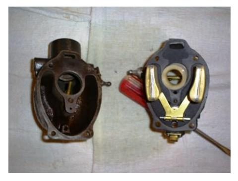
Remove the float by pulling the small pin out. Gently shake the float and listen for liquid. If any is heard replace the float. After removing the float remove the 3 sided float needle and venturi.
