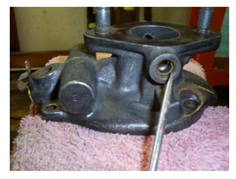
Check the fuel needle valve. It may be viton (rubber) tipped or just steel. Either is acceptable. Observe the hole in the seat for burrs. Check to see that the needle moves in the seat without burrs or snags.
