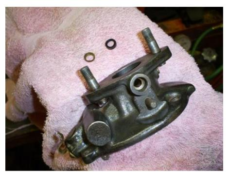
Remove the front hole plug. This hole was used in the manufacturing process only and we will use it to gain access to the small dia holes in the upper carburetor bore. It may be necessary to back out the stud bolt to gain access to the plug.
