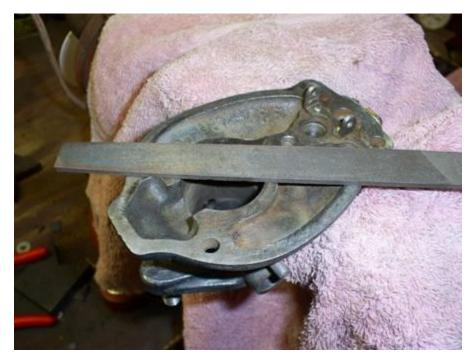
Check to see if the castings mate. There are many carbs out there and the halves may have been swapped or the castings could be damaged or warped. While you may be able to double gasket the carb the dimensions for the venturi are dependent on 1 gasket being used.
