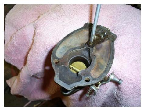
Remove the economizer jet using the widest screwdriver that will fit. I have ground the sides off a couple screwdrivers who tips fit. Many screwdriver shanks are wider than the tip. Keep the blade seated firmly in the jet when removing to avoid twisting the top off.
