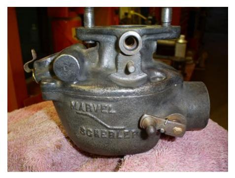
Using the info provided by GB in MT verify the orifice size on your Jets. You can use number drills, or welder tip cleaners with a MIC or any way you can. There are simply too many jets out there to assume yours are correct. I used a set of welder tip cleaners and very small drill bits finding the ones that fit then mic'd them.
