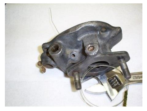
Run a fine mill file lightly across the mating surfaces to remove any burrs only.
