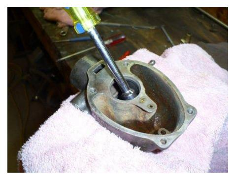
Install the nozzle using a gasket under the hex head. (picture from teardown)
