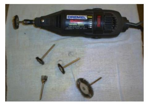
After cleaning your castings, run the wire through all the passages again. After cleaning and running the wire through the passages, clean them again with compressed solvent and follow-up with compressed air directed to all the passages.
