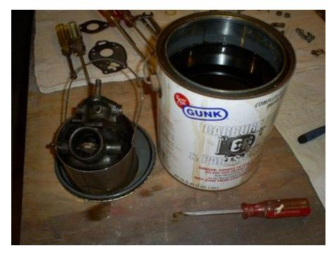
While your castings are soaking inspect all the parts. Replace any worn or damaged parts. I usually only replace parts that are worn or damaged. If you don't know the history of the carb or its in bad shape it may be advisable to order a full kit.
