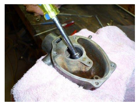
Remove the main jet using the widest screwdriver that will fit. I have ground the sides off a couple screwdrivers who tips fit. Many screwdriver shanks are wider than the tip. Keep the blade seated firmly in the jet when removing to avoid twisting the top off.
