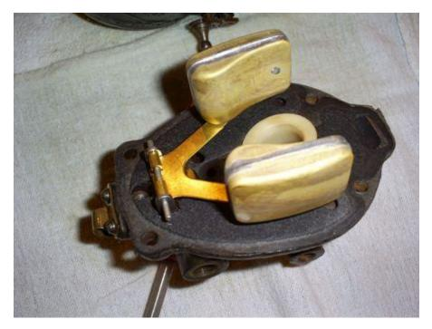
Remove the float valve seat. Note the modified screw driver I'm using. The seat is easily damaged if the screwdriver does not engage the seat fully. This was an inexpensive screwdriver that was ground down to fit the seats. Note the carb top is in a vice with a towel so as to not damage the casting. Keep pressure on the screwdriver to keep it engaged in the seat.
