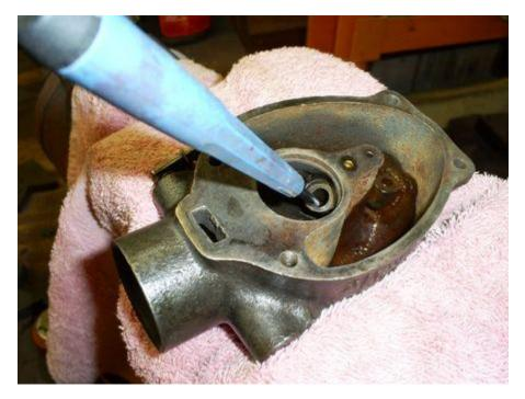
Remove the plug on the bottom of the carburetor. This plug is used to diagnose fuel flow problems but the area is frequently plugged with rust making the test result misleading. These passages lead to the inside of the fuel bowl. Open them with a piece of wire.
