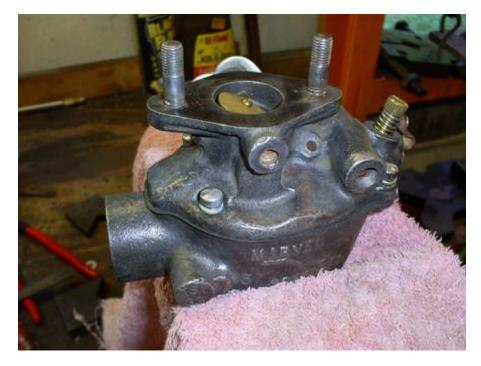
Install the power jet needle/spring/gasket and run it in untill it bottoms out. Back the screw out 1.5 turns. Install the idle mix needle/spring and run it in untill it bottoms out. Back the screw out .75 turns. Install the fuel strainer and install the completed carb on the tractor. If completed as shown and the tractor is in good general shape it will start on these settings once the fuel bowl receives gas.
