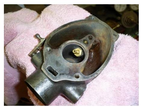
Remove the main nozzle. I use a 3/8 nut driver.
