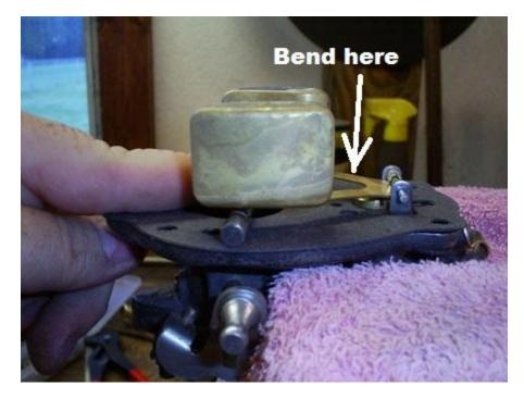
Remove the float and install the venturi. It only fits one way and if you check you will see that one end is larger than the other. Run the small end through a new body gasket and reinstall the float. Don't forget to verify the float needle valve is still in.
