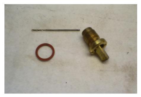
Install the float valve seat and gasket. Use a screwdriver that fits (modified) and tighten securely. Fuel leaking around this seat can cause other problems.
