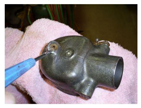
This is a choke butterfly installed backwards. If you see this you need to remove the choke plate and shaft. Unless you have this problem or have a leaking choke packing I recommend not removing the choke plate.
