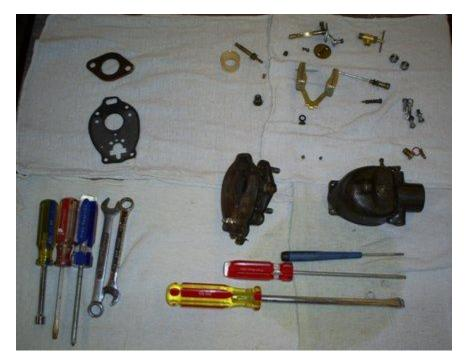
Remove the parts from the carburetor cleaner. While the casting is still wet and using the information documented by GB\_ MT and JMOR run a wire through all the passages. I use guitar strings.
