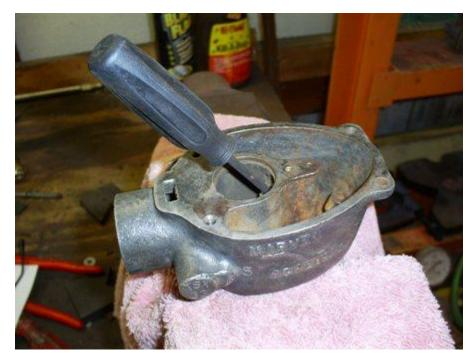
Clean the small holes in the main nozzle. There should be 3. There are other nozzles out there that fit that have different hole arrangements.
