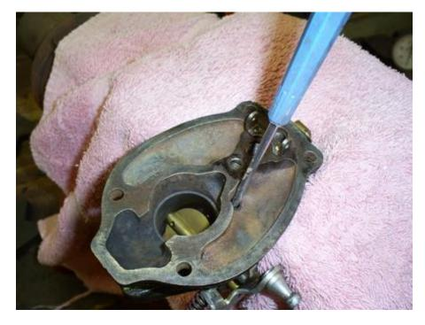
Remove the throttle butterfly by removing the 2 screws. Note the orientation of the butterfly. With the butterfly out, gently pull the throttle shaft out the side of the casting. Note how much play the shaft has up and down. The bore can wear in the casting which can be re-bushed and the throttle shafts wear which can be replaced.
