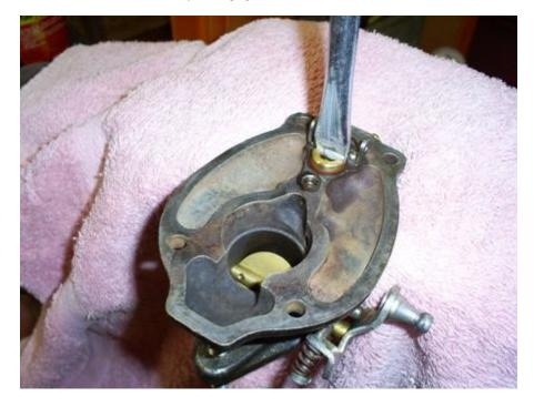
Remove the idle jet. Use a screw driver with the widest blade that will fit. Keep the blade seated firmly in the jet when removing to avoid twisting the top off.
