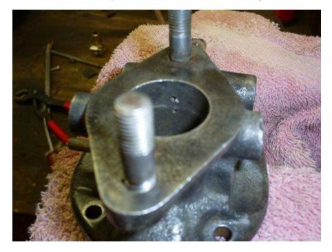
Clean the castings using your favorite canned quick drying solvent. Use the front access hole to spray cleaner in each of the holes ensuring the solvent is exiting a different hole. Here the tube is being directed to the economizer circuit. This is another place for Safety glasses and gloves. Follow-up with compressed air directed to all the passages.
