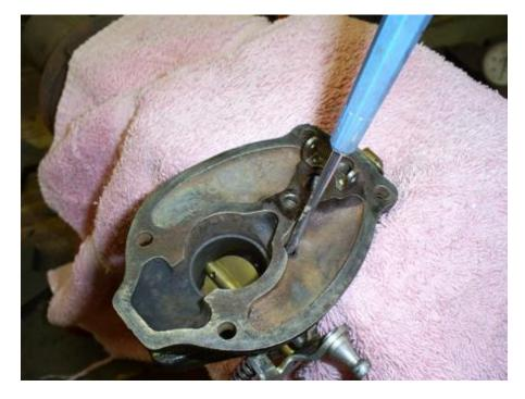
Install the throttle shaft and butterfly. If you've lost the orientation of the butterfly it's easy to determine the orientation. The edges are not machined square and if you observe how it opens it won't take long to see how it should fit plus the screw holes are slightly off center. I rotate the shaft as I tighten the screws down getting the butterfly to center/seat in the opening.
