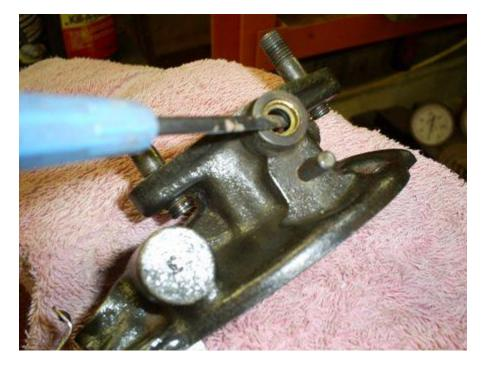
Here the throttle shaft seal and retainer are removed. Note that this carburetor has had a bushing installed in the throttle shaft bore. This is a common repair and the bushing is available from the usual sources.
