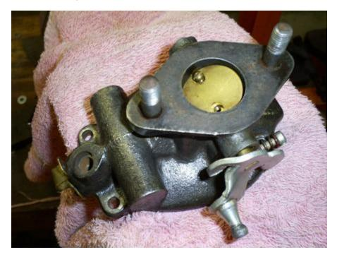
Remove the throttle shaft seal and seal retainer. Here you can see the seal behind the retainer. The retainer is a light press fit and can be removed by gently prying behind it and working around the casting.
