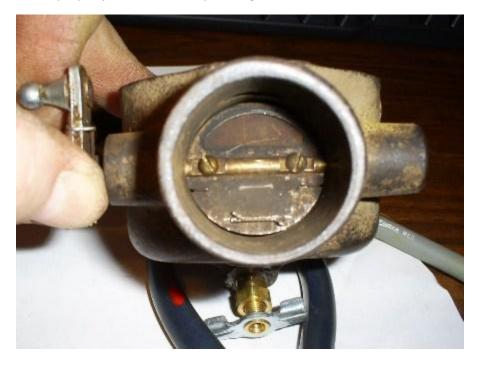
Scrape any remaining gasket material off being careful not to gouge the castings. Place the 2 castings in a gallon of carburetor cleaner and allow to soak. If the carb hasn't been cleaned in years you may want to soak it for a couple of days. This carb was cleaned recently but wasn't idling right. I soaked it overnight. This is a place for safety glasses and rubber gloves.
