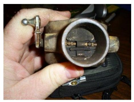
This is properly installed choke plate. Again I wouldn't remove it unless necessary.
