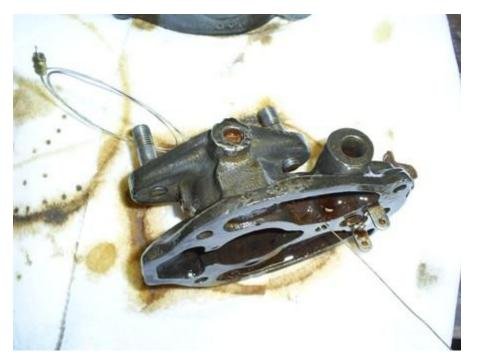
I can always get a wire through the top hole shown. I can sometimes get a wire through the lower hole as it does a tight turn. Not shown is the hole to the side which is part of the economizer circuit which I can't always get a wire through either but will be visible if the casting is turned over and you look in the hole for the economizer jet. Do the same to the lower casting.
