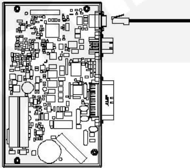
FIGURE 23. NETWORK CONNECTIONS (CONTROL BOARD AND ETHERNET CONNECTION)
