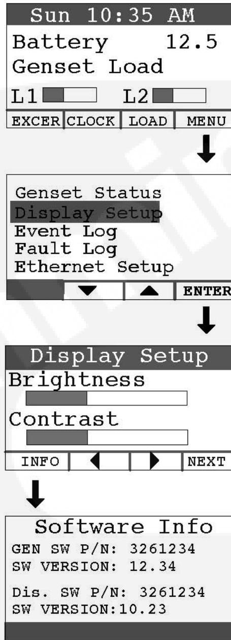
FIGURE 17. DISPLAY SETUP AND SOFTWARE INFO SCREENS
