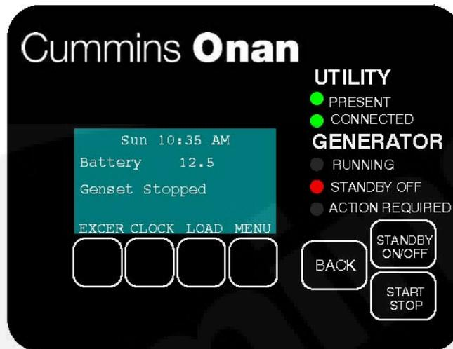
FIGURE 8. UTILITY PRESENT AND CONNECTED—STANDBY OFF LAMP ON
