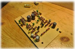
At the Input Amplifier there is an axial capacitor on the back side of the print, the reason for that is entirely unclear to me. This axial electrolytic capacitors have been replaced by a radial type and I have mounted them both on the front of the print. Of course I also replaced the other capacitors.
