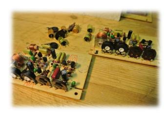
The last two plug-in PCB's. All capacitors are replaced and I replaced on each PCB two setup potentiometers, the other two were already replaced before by a good and sound type. Less beautiful to look at, but replacing good parts is not necessary in my opinion.
