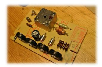
On the Oscillator PCB I replaced the axial elco by a radial type, also in this case a new hole was drilled in the PCB for better mounting of the elco. Replaced 4 setup potentiometers, all settings of the old ones copied and set the new ones on the same value. PCB looks great with the new parts.
