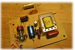
On this PCB only one axial elco to replace, in this case replaced by a new axial one.
