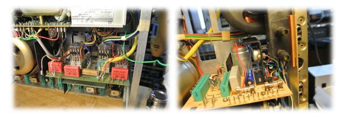
Before I continued with overhauling the plug-in PCB's I first mounted all fixed PCB's back in the recorder. The photographs and sketches that I had made of the wire connections came very useful for this job.
