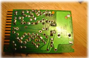
There are two of them in the A77, they are identical, the large axial electrolytic capacitors are replaced by radial types. For a neatly mount on the PCB I drilled a new hole in the PCB. One of the capacitors is mounted above other components, I insulated the connecting wires, just in case. I also replaced the setup-potentiometers.
