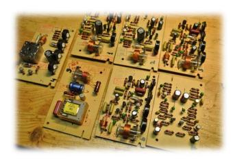
A group picture of all the rebuilt PCB's. Next replaced the PCB's back in the recorder.
