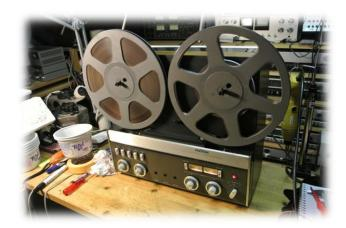
Finally, the front panels and buttons mounted back on the recorder, two reels, one with tape and we can play. Everything is working fine again, sounds fine to me, no audible difference between source and recording and it looks neat again. I am very satisfied with the result and can enjoy this ReVoX A77 for many years again.
