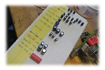
Always nice to get such a package with new parts with an overhauling in prospect. Right here the capacitors are sorted, this way you save up yourself a lot of time to searching during overhauling.
