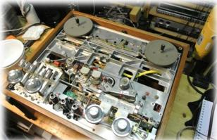
The cabinet is ready and the recorder can be replaced in its cabinet. Replaced bottom plate, removed service pins, removed dummy plug of the remote control and gently placed the recorder back into the cabinet. The mounting screws back in and the recorder can get back on his back. We are not done yet.
