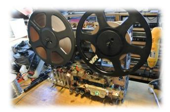
At first I check if all functions are working correctly. All functions appear to work fine, play, winding left, winding right, record, brakes, no problems at all. Some creaking of the switches fixed with an IPA treatment. There is also a clear volume difference between source and recording, but that was to be expected given almost all setup potentiometers have been replaced. So the next step is to adjust the recorder in accordance with the service manual.
