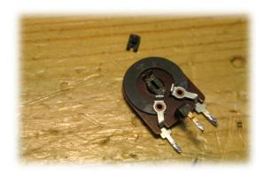
I measured the original setting of the old potentiometer, next I set the new potentiometer to the same value before soldering the new potentiometer on the PCB. Now I know that the setting is at least in the right direction.
