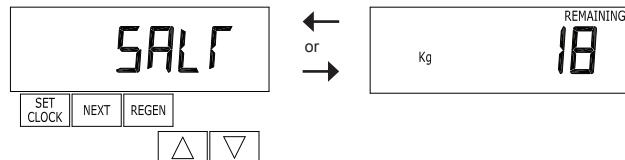
Once the salt remaining has gone below the set point the display will automatically flash Salt Fill.
