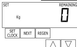
**Step 3US** – Set Kg REMAINING: Use the ▼ or ▲ button to adjust the Kg remaining in the brine tank.
