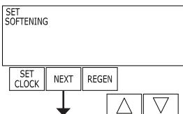
**Step 2S** – Choose SOFTENING using the ▼ or ▲ button. Press NEXT to go to Step 3S. Press REGEN to exit OEM Softener System Setup.
