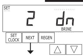
**Step 7CS** - Press the ▼ or ▲ buttons until dn BRINE appears. Press NEXT to go to Step 8CS. Press REGEN to return to previous step. For a WS1 control valve; prior to selecting a regenerant flow cycle, verify the correct valve body, main piston, regenerant piston and stack are being used, and the injector or injector plug(s) are in the correct location. Refer to WS1 & WS1.25 Common Information manual, Valve Body Compliance Table.
