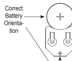
Battery replacement is 3 volt lithium coin cell type 2032.
