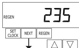
**STEP 3VH** – Regenerations, total number since start-up: This display shows the total number of regenerations that have occurred since startup. Press the **NEXT** button to go to Step 4VH. Press **REGEN** to return to previous step.
