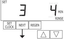
**Step 5S** – Select the time for the third cycle (which in this example is RINSE) using the ▼ or ▲ button. Press NEXT to go to Step 6S. Press REGEN to return to previous step.
