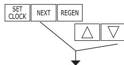
**Step 1S** – Press NEXT and ▼ simultaneously for 3 seconds and release. If screen in Step 2S does not appear in 5 seconds the lock on the valve is activated. To unlock press ▼, NEXT, ▲, and SET CLOCK in sequence, then press NEXT and ▼ simultaneously for 3 seconds and release.
