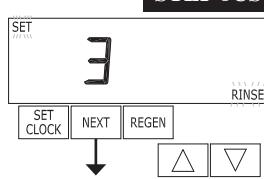
**Step 8CS** - Press the ▼ or ▲ buttons until RINSE appears. Press NEXT to go to Step 9CS. Press REGEN to return to previous step.
