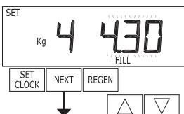
**Step 6S** – Select the Kg for the fourth cycle (which in this example is FILL) using the ▼ or ▲ button. Press NEXT to go to Step 7S. Press REGEN to return to previous step.
