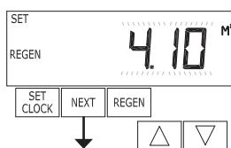
**Step 7F – Set Volume Capacity** using the ▼ or ▲ button. If value is set to:
