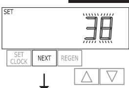
**Step 2CS** – Use the ▲ or ▼ to select 25 for WS1 valve, 32 for WS1.25 valve, 38 for WS1.5 valve or 50 for WS2L valve. Press NEXT to go to Step 3CS. Press REGEN to exit OEM cycle sequence.
