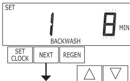
**Step 3S** – Select the time for the first cycle (which in this example is BACKWASH) using the ▼ or ▲ button. Press NEXT to go to Step 4S. Press REGEN to return to previous step.
