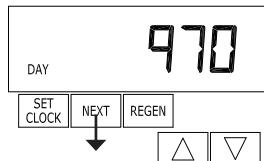
**STEP 2VH<sup>2</sup>** – Days, total since start-up: This display shows the total days since startup. Press the **NEXT** button to go to Step 3VH. Press **REGEN** to return to previous step.
