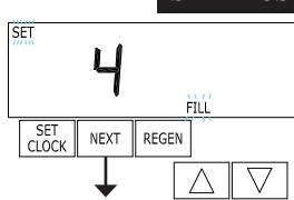
**Step 9CS** - Press the ▼ or ▲ buttons until FILL appears. Press NEXT to go to Step 10CS. Press REGEN to return to previous step.
