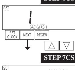
**Step 6CS** – Press the ▼ or ▲ buttons until BACKWASH appears. Press NEXT to go to Step 7CS. Press REGEN to return to previous step.
