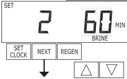
**Step 4S** – Select the time for the second cycle (which in this example is dn BRINE) using the ▼ or ▲ button. Press NEXT to go to Step 5S. Press REGEN to return to previous step.
