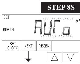
**Step 8S** – Set Volume Capacity using the ▼ or ▲ button. If value is set to:
