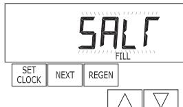
When adding salt to the brine tank (if the salt remaining feature is activated) the following steps must be completed:
