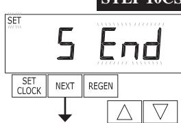
**Step 10CS** - Press the ▼ or ▲ buttons until END appears. Press NEXT to exit OEM Cycle Sequence. Press REGEN to return to previous step.
