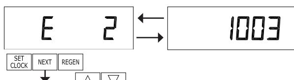
**STEP 5VH** – Error Log: This display shows a history of the last 10 errors generated by the control during operation. Press the **▲** or **▼** buttons to view each recorded error. Press the **NEXT** button to exit Valve History. Press **REGEN** to return to previous step.
