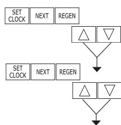
**STEP 1VH** – Press **▲** and **▼** simultaneously for three seconds and release. Then press **▲** and **▼** simultaneously and release. If screen in step 2VH does not appear in 5 seconds the lock on the valve is activated. To unlock press **▼**, **NEXT**, **▲**, and **SET CLOCK** in sequence, then press **▲** and **▼** simultaneously for 3 seconds and release. Then press **▲** and **▼** simultaneously and release.
