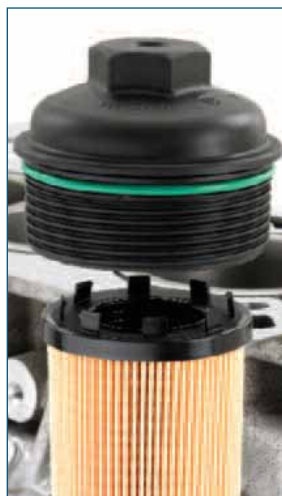
The O-ring on an ACDelco OES oil filter cap will not compress and develop a flat side. (Service reminder: Insert the filter in the cap before installing in the engine.)
