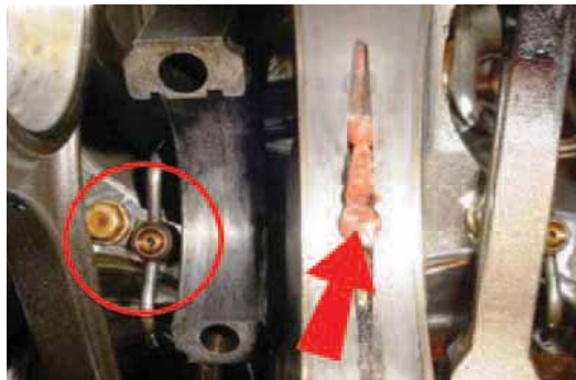
Foreign material blocking oil flow to the main and rod bearings.
