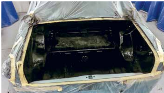
CLOCKWISE FROM TOP LEFT: Front quarter panels, hood and trunk in the spray booth. The painted rolling chassis. Painted and baked quarter panels before being reunited with the chassis. The trunk needed some work! Repaired, masked and sprayed trunk interior. Heckflosse comes home, and now it's time for the next step in the restoration.
