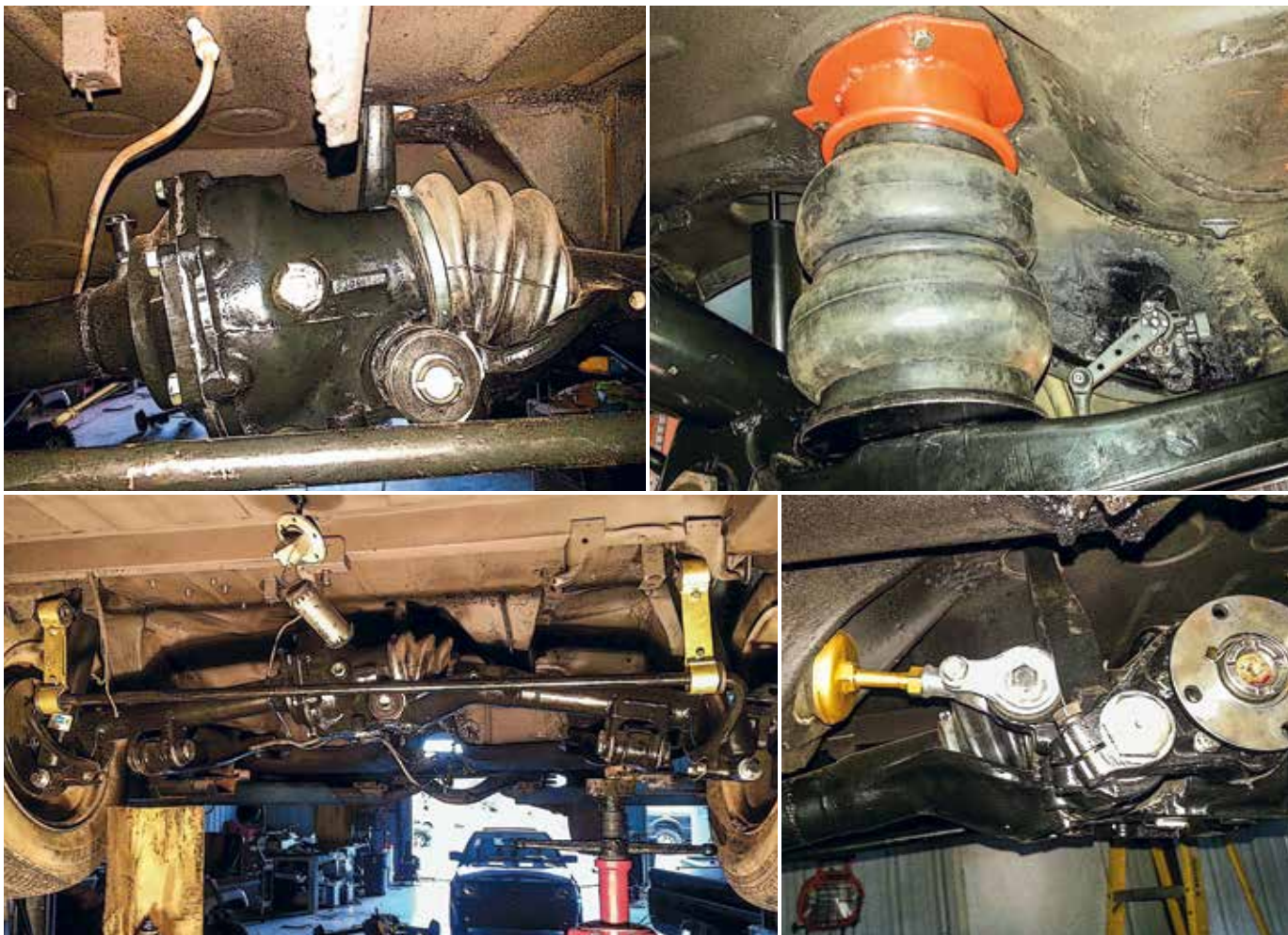
CLOCKWISE FROM TOP LEFT: My rebuilt W112 swing-axle differential. Removing and tearing down one of these requires great care, with special tools and specific disassembly and reassembly procedures. A rear airbag/air can assembly installed. View of a rear suspension stabilizer. The completed rear suspension. The vertical yellow elements are the rear anti-sway bar links. I am very pleased with my aftermarket air suspension system. The only modification I had to make to the Heckflosse was to drill two one-eighth-inch mounting holes in the body and subframe for each sensor. I have all original parts and can return the suspension to factory specification at any time.
