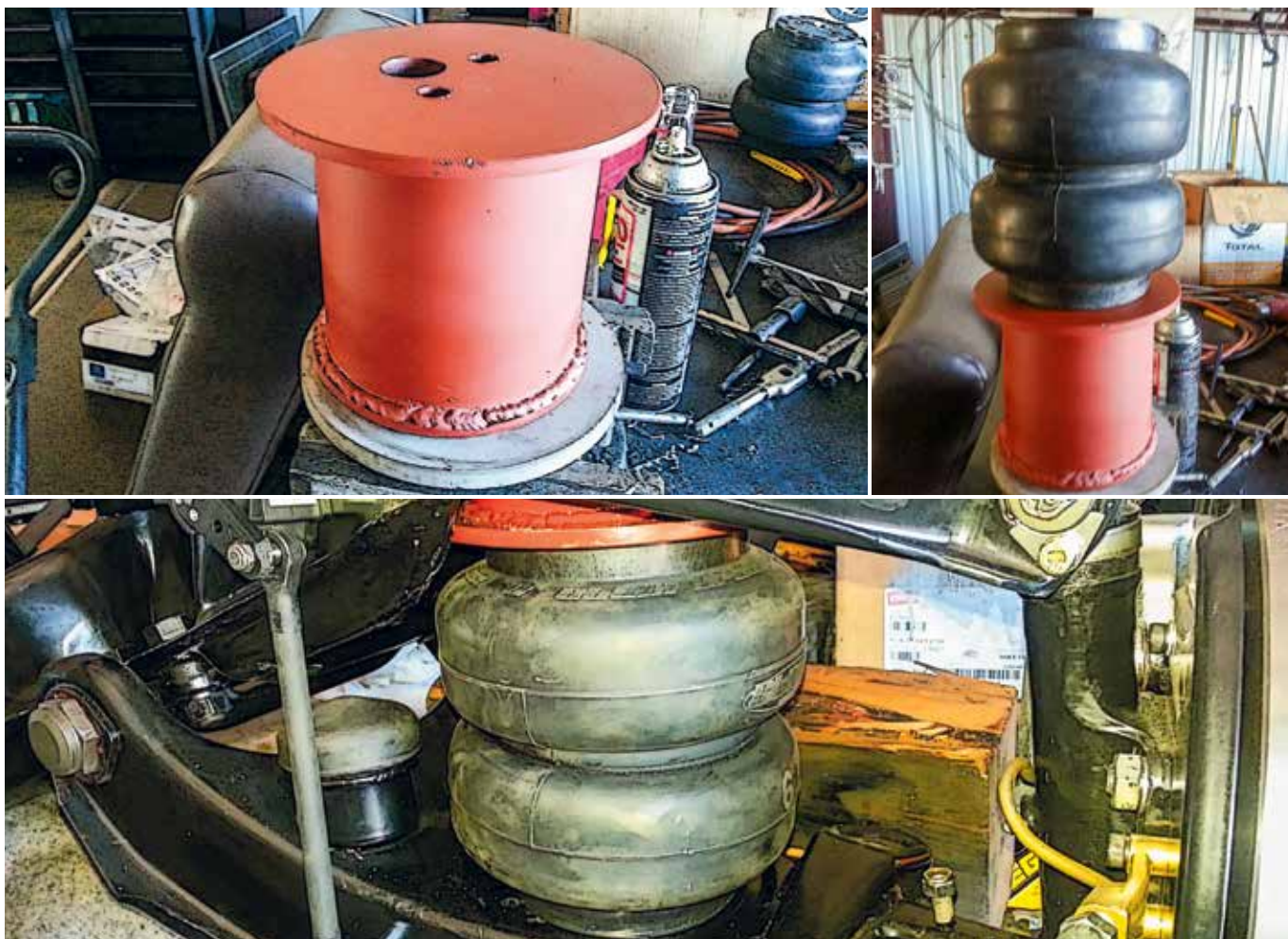
CLOCKWISE FROM TOP LEFT: After researching and pricing the parts needed to get the factory suspension working, I decided instead to install a modern four-corner suspension system, which uses electronic ride-control sensors at each corner of the car similar to the yaw and height sensors used on 2014 Mercedes models. This modern system helps keep the car perfectly level, improving ride and handling over the original system. As a first step, I had to fabricate new air bag cans so that none of the original Mercedes parts were altered. A completed airbag/airbag can assembly. Detail of the completed front suspension with airbag system installed.
