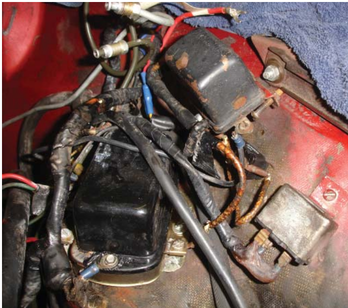
This under hood rats' nest shows much evidence of splices and patches gained over the years. Everything worked, at least most of the time. But just looking at this mess made me shudder.
