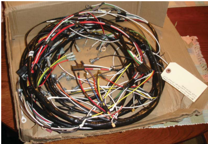
The Avanti's main harness as it arrived from Studebakers West. A couple specialty connectors and grommets are not included and must be reused from the old. All the many white wires are grounds, needed since this is a fiberglass bodied car.
