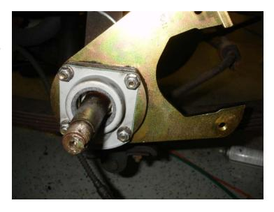
Installing the shims/washers etc. in the wrong order can clamp the wheels solidly in place. Just make sure you haven't done so. Use a drop of red Locktite on the threads of each mounting bolt for extra safety.
