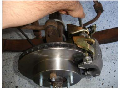
remove the tape and slide it out once the caliper is installed.
