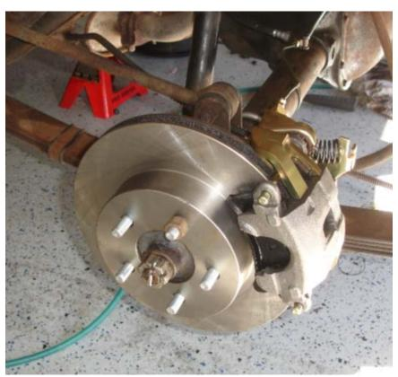
The Turner rear disc conversion is well engineered, but is in some ways a bit more difficult than the front conversion to install. While the front brakes are very much a bolt-on affair, requiring few specialized tools or knowledge, mounting the rear brakes present a number of twists that, while not difficult for the experienced garage mechanic, make the change-over a bit more complicated.
