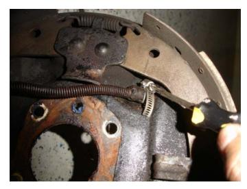
spring from sliding back into place. Then, using the first pair of vice grips, clamp onto the end of the brake cable and twist it free.
