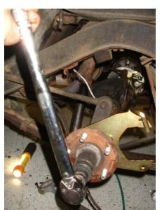
**Step 8-** Now reinstall the hub. Clean the axle shaft and the inside of the tapered hub thoroughly with solvent and dry them. Leaving grease on the mounting surfaces leaves you with the possibility of cracking the hub when torquing it into place.
