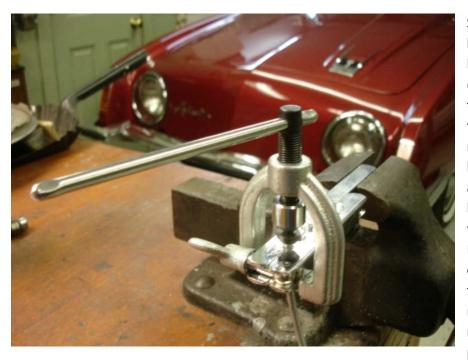
Starting with storebought lengths of steel brake line, I cut them down and double flared the ends to make them the proper length to mate with the flexible braided steel hoses that are supplied with the kit. Never use Teflon tape on these fittings. Brake fittings are double flared because the flare against the matching seat is what makes the highpressure connection
