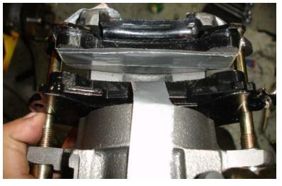
parts you will know what to ask for at the parts counter. The calipers are not marked 'right' or 'left', but just remember that the bleeder screw faces INSIDE towards the center of the car, and the bleeder is at the top of the caliper and you will have it right.
