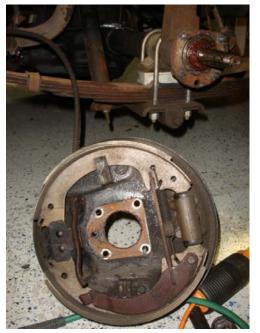
There is no need at all to waste time disassembling the brakes from the backing plate. Simply remove the brake line from the backing plate with a brake tubing wrench. I strongly suggest replacing all steel brake lines with new ones. You will need to shorten them from original anyway, and there is no sensible reason to reuse nearly fifty year old steel lines that you depend on for your life.
