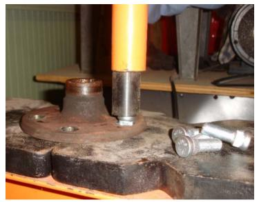
Step 5- Remove the old studs from the hub. The press makes quick work of these. Notice that the original studs are smooth and not knurled, explaining why these are known to frustratingly strip and spin on occasion.
