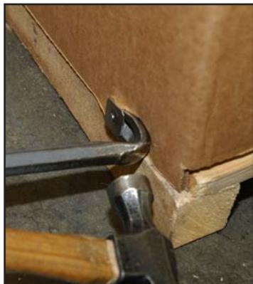
Image 2. Remove nails securing cardboard box to skid.
