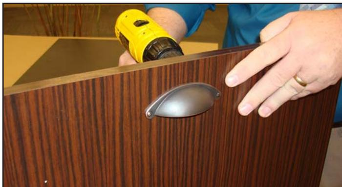
Image 4. Attach drawer handle to overlay panel.
