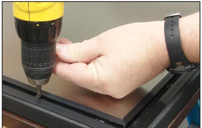
Image 9. Anchor overlay on door front.
