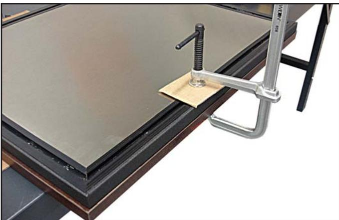
Image 7. Clamp door front with the overlay panel.
