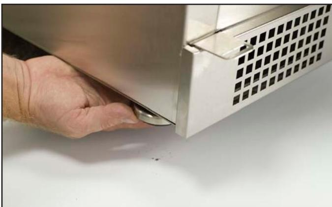
Image 1. If the front of the cabinet needs to be lowered or raised adjust the leg levelers.
