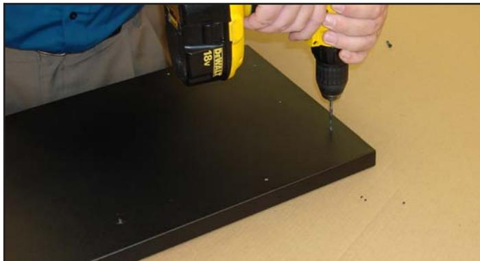
Image 3. Drill out eight pilot holes from the front of the drawer panel.
