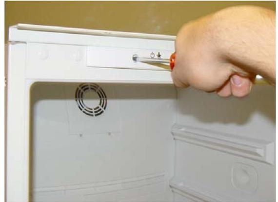
4. Loosen the printed circuit board screws
