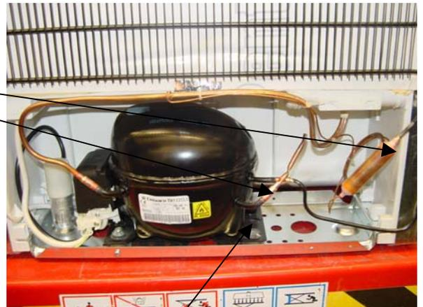
4. Loosen the screwed connection and remove the compressor
