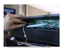
e. When changing the control panel, you should push the button to pull out of the control panel. Do never pull it wildly without pushing the button. That will break it.
