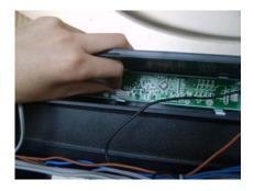
d. The socket of sensor wire is connecting
