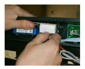
c. One side of the signal wire was connecting with the control panel, the other side was connecting with the middle of the display panel. Take it apart firstly, note that you should unplug it softly in order to protect the plug.
