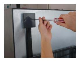
C. When you take the box cover apart, as on the picture, the blue one is lamp wire, connecting with the connect wire and ballast wire. The red one is fan wire, connecting with the control wire. The white one is connect wire, connecting with heater wire.
