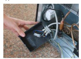
e. The ba llast w ire has I ocked onese If port, When changing it, you can use a thin steel bar insert in the faucet and then pull the wire out, when fix the wire again you need to use the other two faucet, the used ones is broken for it is one-off.
