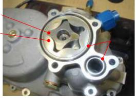
Tighten oil pump with bolt M6-60, 4 bolts M6-110 and washers evenly to 1.2 [kgfm] applying LOCTITE243.
