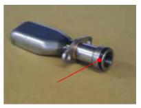
• Place oil strainer to RH crankcase and tighten bolt M6-20 temporary.
