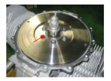
**CHANGE PARTS AT OVERHAUL: M8-13 bolt**
