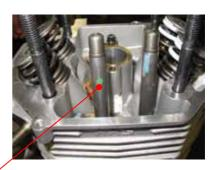
**NOTE:** Coloring side is turned to cylinder head side.
