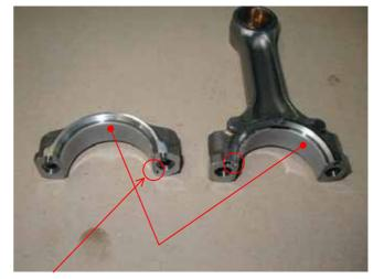
**NOTE:** Confirm the turn stop of bearing entered the ditch.
