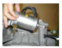
• Tighten electric starter with 2 bolts M6-35 and washers to 1.2 [kgfm] applying LOCTITE 243.
