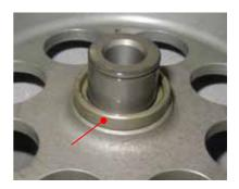
• Compress gear using **ST-07** and attach half rings with the flat side out.
