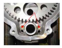
Remove 8 bolts M6.Remove 2 bolts M8.
