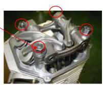
• Lift out push rods; stop oil dripping by sealing with finger.
