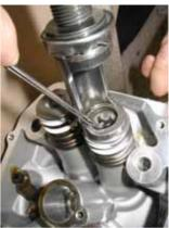
• Remove valve spring retainer, valve springs and valve.
