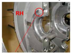
**NOTE:** There are two kinds of bearings. Bearing with a lug is attached to a RH side crankcase. Flat side of bearing is assembled to the crankcase side.
