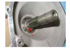
• Press PTO shaft to remove from gearbox.
