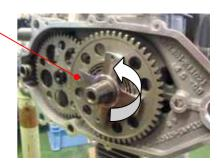
Attach idler gear , idler shaft and 2 thrust washers applying motor oil.
