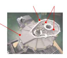
• Attach drive gear and washer to crankshaft.
