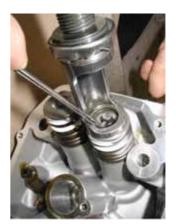
**NOTE:** Check correct positioning of valve cotters.
