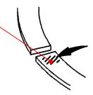
Insert **new** piston pin circlip in groove of front marked (triangular sign) side.
