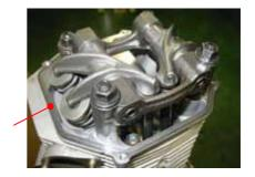
• Attach cylinder head cover to cylinder head with 5 bolts M5-25 with LOCTITE 243 and washers. Tighten evenly to 0.8 [kgfm].
