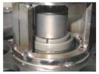
• Set inner race with **ST-09**. Press **ST-07** to insert inner race.
