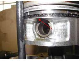
**CHANGE PARTS AT OVERHAUL:** Piston, piston pin, piston rings and piston pin circlip (See para 7)
