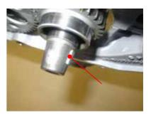
• Fit stator hub and washer Apply LOCTITE 243. to bolt M10-50 and tighten to 5.0 [kgfm].
