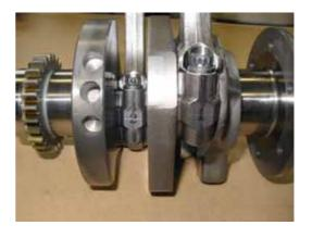
**CHANGE PARTS AT OVERHAUL:** Connecting rod bearing (See para 6.1)
