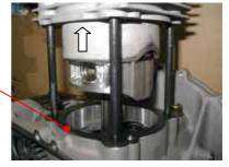
Remove piston pin circlip using the specially shaped screwdriver.
