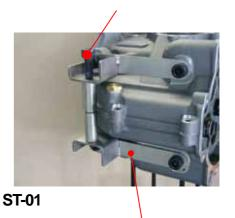
Split crankcase with tightening bolt.
