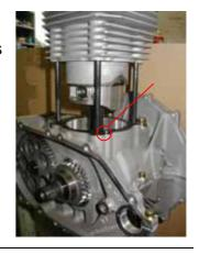
**CAUTION:** Use piston ring spanner to avoid ring breakage.
