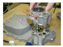
• Shift to remove inner feed rotor Assy
