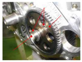
• Remove driven gear by turning clockwise (left).
