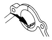
• Fix oil strainer with 2 bolts M6-20 with applying LOCTITE 243. Tighten to 1.2 [kgfm].
