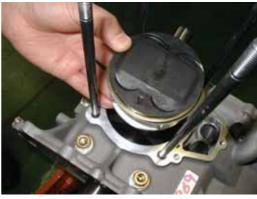
• Insert **new** piston pin circlip in another groove.
