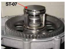
• Compress gear and remove half rings .
