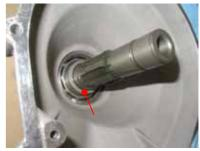
• Attach 12 spring washers on the shaft as illustrated.
