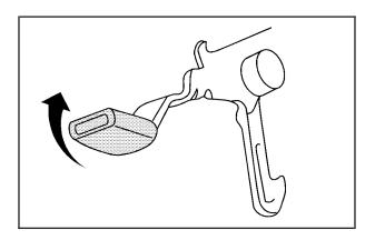
Then go to the front of the vehicle and lift up the secondary hood release lever. The secondary hood release lever is located under the front center of the hood.
