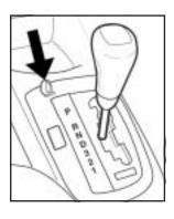
Insert the key into the shift-lock release slot and press and hold the key.
