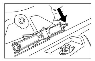
6. Remove the jack, the jack handle and the wheel wrench. The jack is located in the trunk, in front of the compact spare tire. Turn the jack retainer, located on the right side of the jack, counterclockwise to release it. The jack handle and the wheel wrench are located inside the foam tray.
