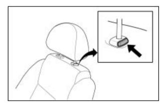
Push in the release button in order to adjust the position downward.
