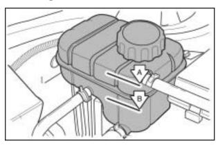
The engine coolant surge tank is located in the rear of the engine compartment on the driver's side. See *Engine Compartment Overview on page 5-12* for more information on location.
