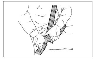
To unlatch the belt, just push the button on the buckle.
