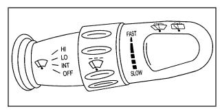
Use this lever located on the right side of the steering wheel to operate the windshield wipers. The ignition must be turned to ON to operate the windshield wipers.
