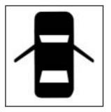
If one of the doors on your vehicle is not closed properly while the ignition is on, the door ajar light on the instrument panel cluster will come on and stay on until the doors are closed. See Door Ajar Light on page 3-40 for additional information.
