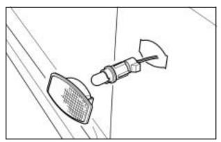
Remove the bulb from the lamp housing by pulling the bulb straight out of the socket.
