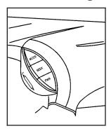
If your vehicle has this feature, some audio controls can be adjusted at the steering wheel. They include the following:
