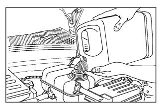
3. Fill the coolant surge tank with the proper mixture to the MAX mark on the coolant surge tank. Wait about five minutes, then check to see if the level is below the MAX mark. If the level is below the MAX mark, add additional coolant to bring the level up to the MAX mark. Repeat this procedure until the level remains constant at the MAX mark for at least five minutes.
