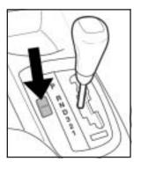
Press the HOLD button on the shift lever console to turn on hold mode.
