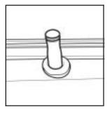
All doors, except for the driver's door, can be locked from the outside by pushing down the manual door lock and then closing the door.
