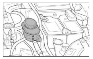
The level should be between the MIN (B) and MAX (A) marks on the reservoir. If the level is below the MIN (B) mark, add the power steering fluid to the appropriate level. Replace the cap and completely tighten it.
