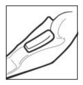
To adjust the seatback, lift the lever located on the outboard side of the seat and move the seatback to where you want it.
