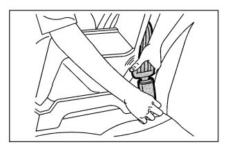
3. Buckle the belt. Be sure the latch plate clicks when you put it into the buckle. This means you are using the correct buckle. Also, make sure the release button is positioned so you would be able to unbuckle the safety belt quickly if you ever had to.
