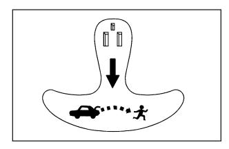
There is a glow-in-the-dark emergency trunk release handle located inside the trunk on the underside of the trunk lid. This handle will glow following exposure to light. Pull the release handle down to open the trunk from the inside.
