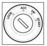
With the key in the ignition switch, you can turn the key to four different positions.
