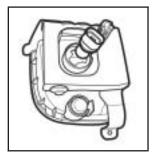
Disconnect the wiring harness connector from the fog lamp bulb socket.
