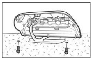
Remove the two screws which are recessed on the underside of the hood.
