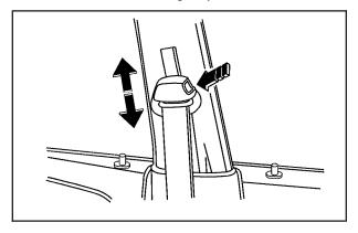
To move the shoulder belt height adjuster down, press the release button and move the height adjuster to the desired position. After you move the height adjuster to where you want it, try to move it down without pressing the release button to make sure it has locked into position.
