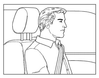
Adjust your head restraint so that the top of the restraint is closest to the top of your head. This position reduces the chances of a neck injury in a crash.
