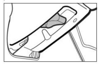
The lever that allows you to tilt the steering wheel is located under the steering column.
