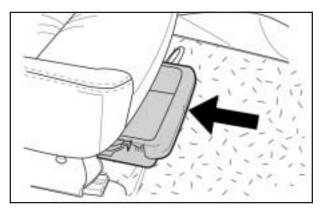
Your vehicle may have a sliding storage tray located under the front passenger seat. To use the tray, pull up on the end of the tray and pull it toward the instrument panel. Push the tray toward the seat to return it to its original position.
