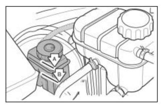
You do not need to check the fluid level unless you suspect a clutch problem. To check the fluid level, look on the side of the reservoir. If the fluid reaches the MAX (A) mark on the reservoir, the fluid level is correct. The reservoir is located near the back of the engine compartment on the driver's side of the vehicle. See *Engine Compartment Overview on page 5-12* for more information on location.
