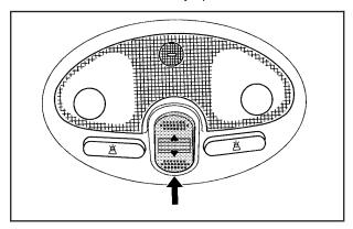
To open the sunroof to the vent position, push the front part of the switch. To return the sunroof to its original position, push the rear part of the switch and hold it until the sunroof reaches the desired position.
