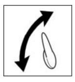
To adjust the front seat lumbar support, use the lever located on the outboard side of the seatback.
