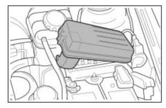
The engine compartment fuse block is located on the driver's side of the vehicle, near the battery. See *Engine Compartment Overview on page 5-12* for more information on location. To access the fuses, press in the top flap to release the cover.
