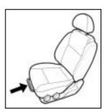
Pull up and hold the bar located under the front of the seat to unlock it.
