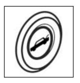
Press the remote trunk release button, located on the side of the driver's door trim, to release the trunk lid.
