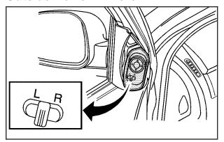
Your vehicle may have outside power mirrors. The control for the power mirrors is located on the driver's side door trim.
