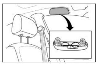
The sunglasses storage compartment is located above the driver's door. To open the sunglasses storage compartment, pull down and hold the upper part of the cover. To close the compartment, let go of the cover and the compartment will automatically close.
