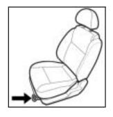
Pull up and hold the lever located under the front of the seat to unlock it.
