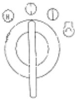
Flameout: The key switch may be inserted or pulled out only at this position. As the switch is situated at this position, the power source of most circuits of the cab will be shut off.
