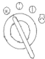
Pre-heating: Turn the key switch anticlockwise to this position to put through preheating device.
