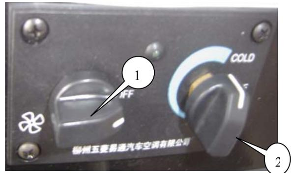
1 Blowing rate switch 2 Temperature control switch
