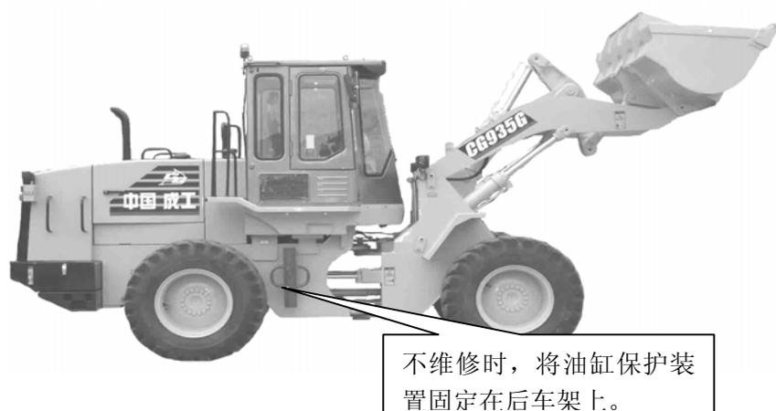
文本筐: When not repairing, fix the protective device for the oil cylinder at the rear frame.
