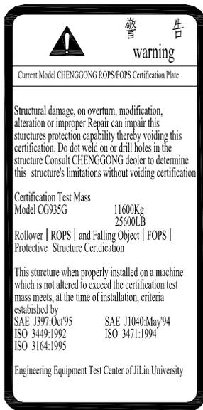
**The cab has a rollover And falling object protective structure which shall not be modified.**
