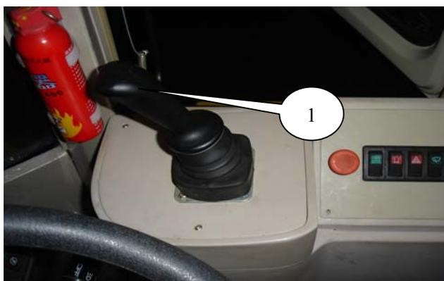
In bucket reversion, the joy stick (1) shall be placed at the position of bucket reversion. And then turn back it to the original position. Repeat the operation until materials are unloaded.
