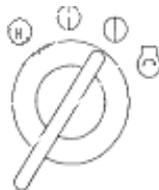
Rotation: Turn the key switch clockwise to this position to put through the power of electronic control and cab meter,, charging indicator's relav etc.
