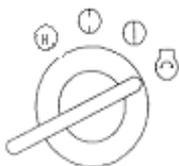
Starting: Turn the key switch clockwise to this position to start the engine. After starting, release the key switch, the key switch will automatically return to the power-up position.
