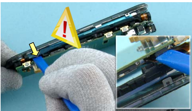
21) Use the SS-93 to open the LCD FRAME ASSY connector. While opening the connector, be careful not to damage the connector or any nearby components!
