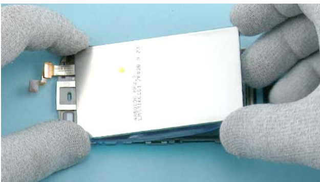
33) Remove also the LCD.
