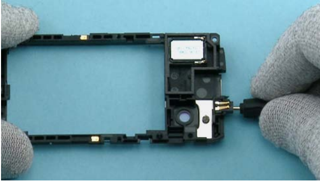
37) Use the DC plug to lift up the DC JACK.
