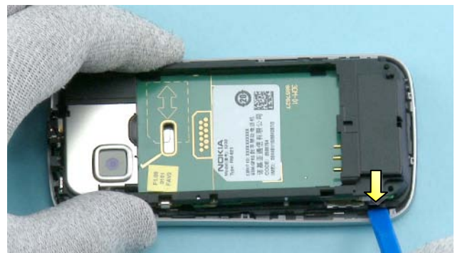
10) To remove the A-COVER, first release the clip from the bottom corner with the SS-93.
