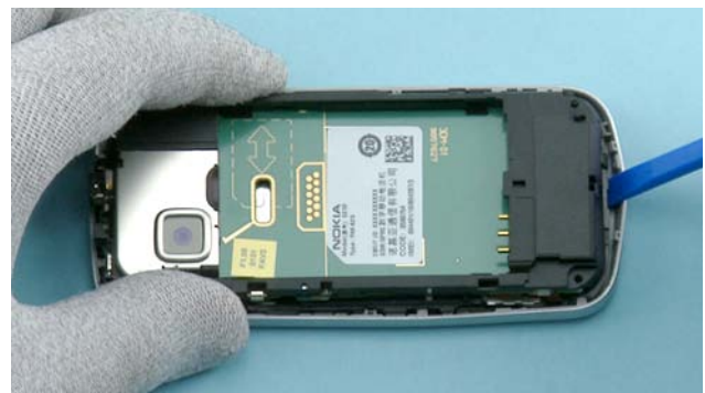
12) Then release the remaining clips on both sides of the phone.
