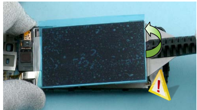
18) Lift up the bottom side of the LCD and then carefully lay it down. Be careful not to break the flex!
