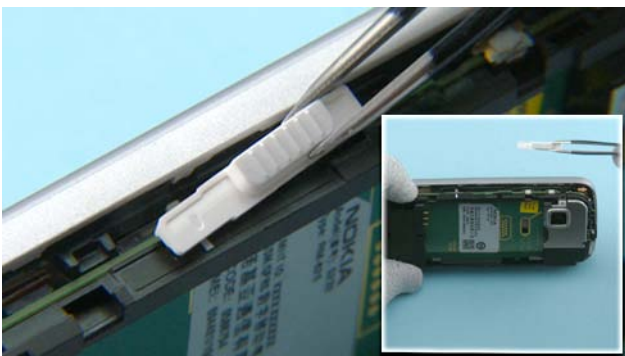
9) Remove the SLIDE KEY with the tweezers.
