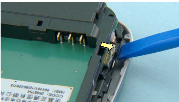
11) Continue to the bottom side and release two clips holding the A-COVER.
