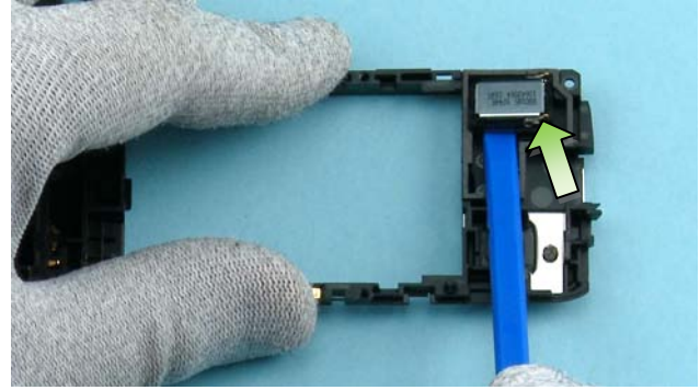
38) Lift up the IHF SPEAKER with the SS-93 and remove it using tweezers. Remains of the GASKET have to be removed from the IHF SPEAKER.
