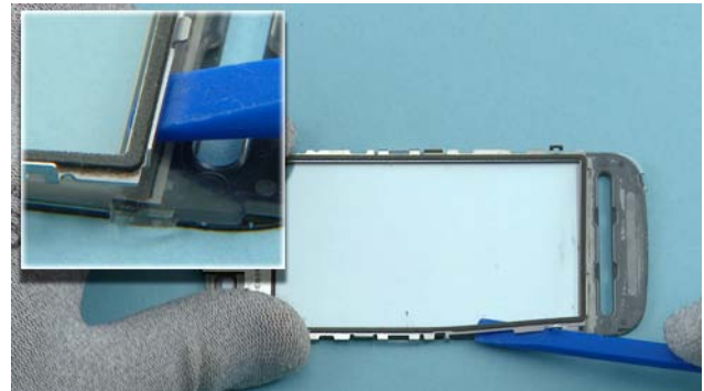
40) Use the SS-93 to detach the TOUCH FRAME ASSY from the TOUCH PANEL ASSY. TOUCH FRAME ASSY and TOUCH PANEL ASSY can now be separated. Note: If TOUCH PANEL ASSY or TOUCH FRAME ASSY is damaged, both of them need to be renewed. However, if TOUCH PANEL ASSY and TOUCH FRAME ASSY are undamaged, they should be reused
