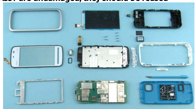
42) Nokia 5235 disassembly is now complete.
