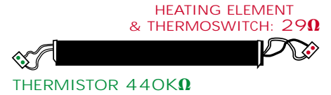
AX RESISTANCE TEST POINTS
