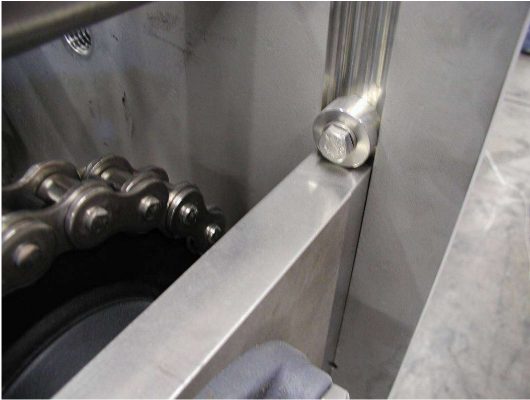
6" BAR WITH RAIL STOP IN PLACE
