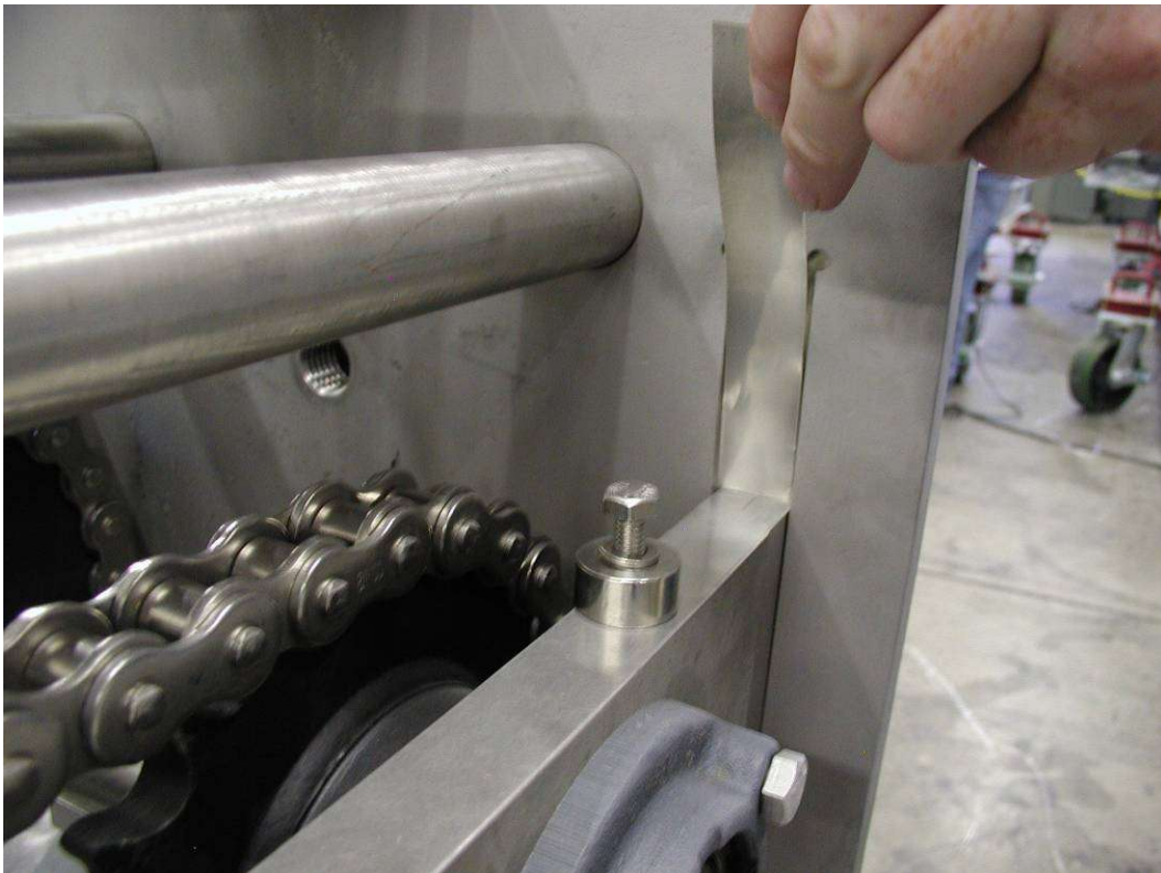
6" BAR WITH RAIL STOP REMOVED, READY FOR INSTALLATION OF SHIMS
