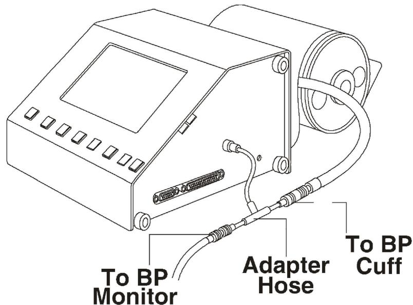
Figure 8 - Connecting AccuSim-BP to the NIBP Monitor
