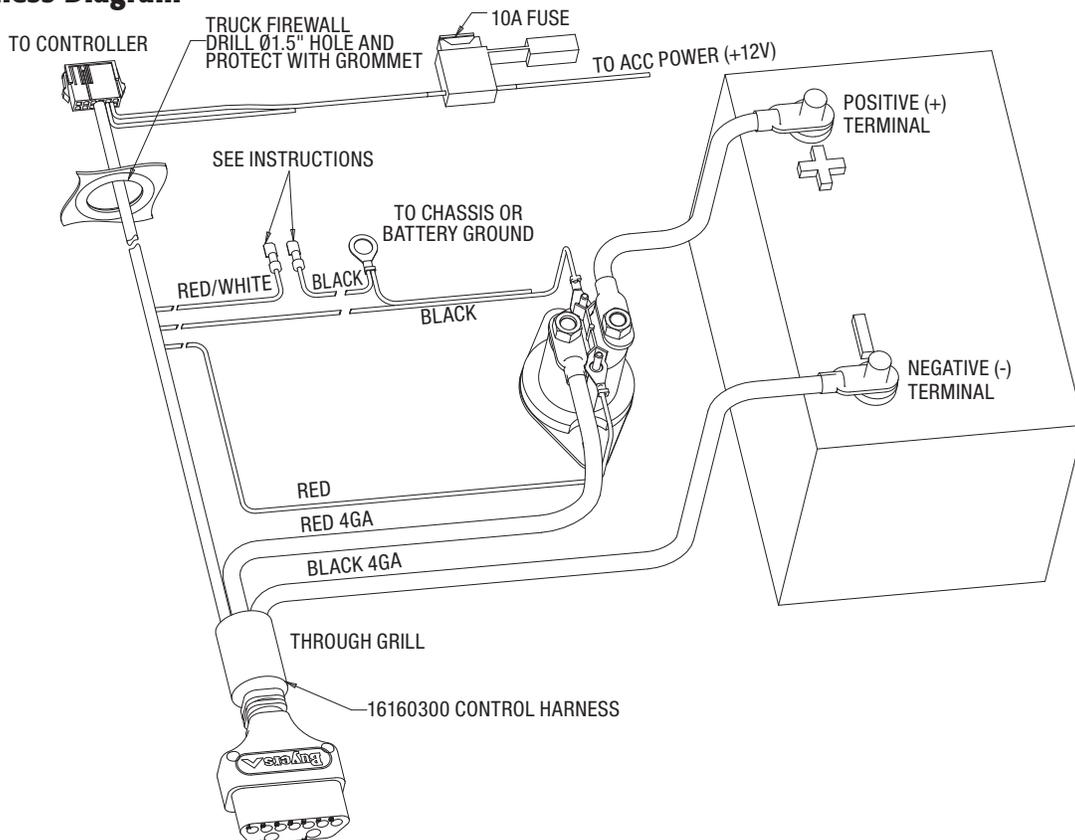
1. Route the CONTROL HARNESS through the truck grill, by the battery, and through the firewall. Some trucks will require drilling a  $\varnothing 1.50$ " hole through the firewall, while some will have holes provided (usually plugged). Check your truck Owner's Manual for details. If the hole is drilled it is critical that a grommet be used to prevent damage to the wire harness.
