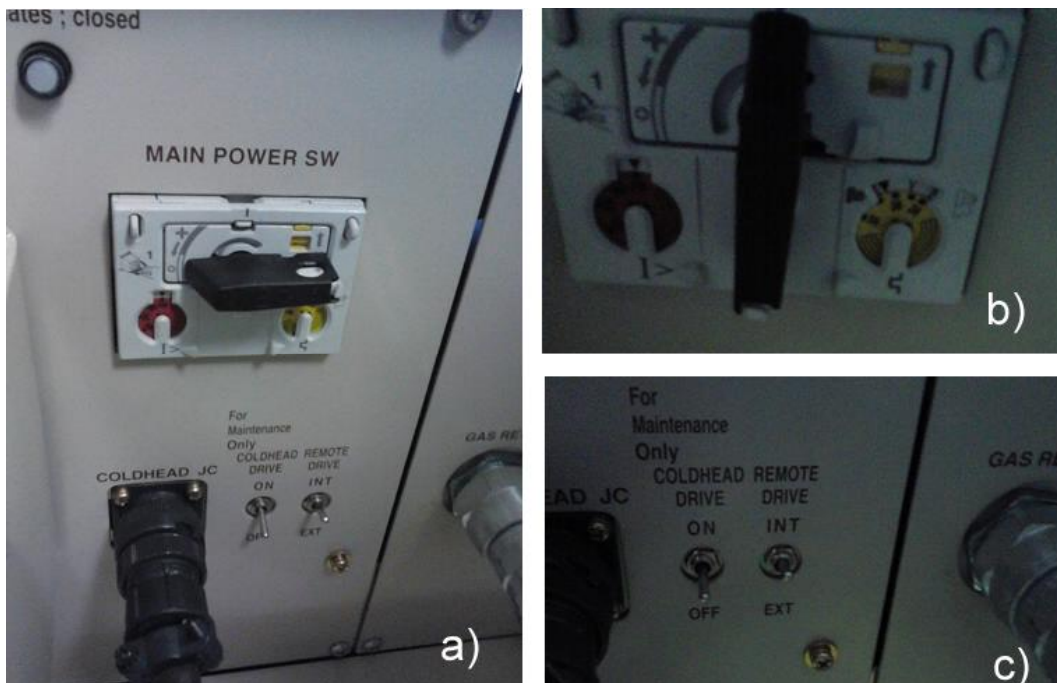
Figure 6: (a) The He-compressor is powered off. (b) The main power is turned back on. For purging the cold head without connecting the flux-lines, the cold-head drive should be turned on (c): however in the image it is off). Cold-head drive switch should be turned off after reconnecting the flux lines and the He-compressor in the normal operational mode.
