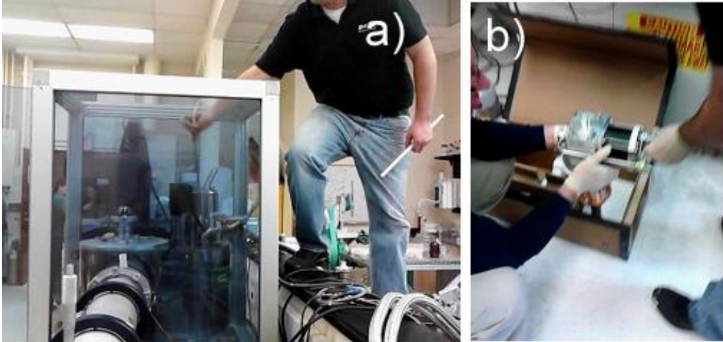
Figure 5: (a) The magnet chamber was cleaned with Kim wipe (ethanol) and then subsequently purging with He-gas prior to attaching the cold-head. (b) Disassembling the refurbished cold-head from the casing by unscrewing the 4 hex screws.
