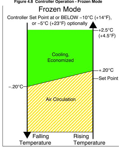
Figure 4.8 Controller Operation - Frozen Mode
