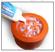
b. Install the orange gasket part onto the compressor fusite with the grooved or threaded side out as shown in Figure 7.8. Ensure that the gasket is seated onto the fusite base.
