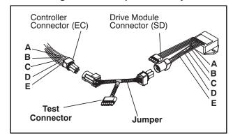
There should be approximately five volts DC on sockets "C" and "D" (S1 and S2) when measured as above. If not the connections or controller is faulty. If any of these pins are not consistent, the connections or the controller is suspect. Check and replace as required.
