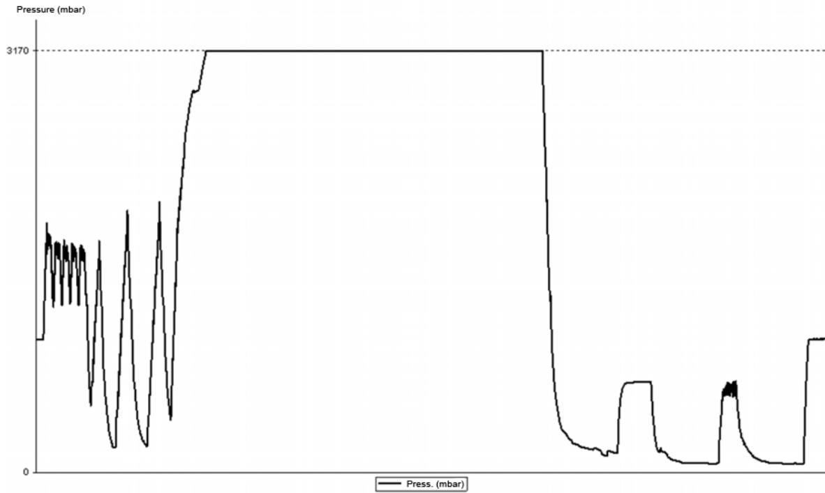
Fig. 10: Pressure-Time chart for Prion-Program, 134 °C and 2.1 bar
