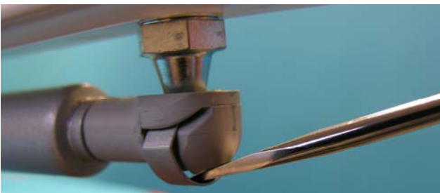
Fig. 5.1.2/ 4 Detaching soft stop mechanism from spherical head
