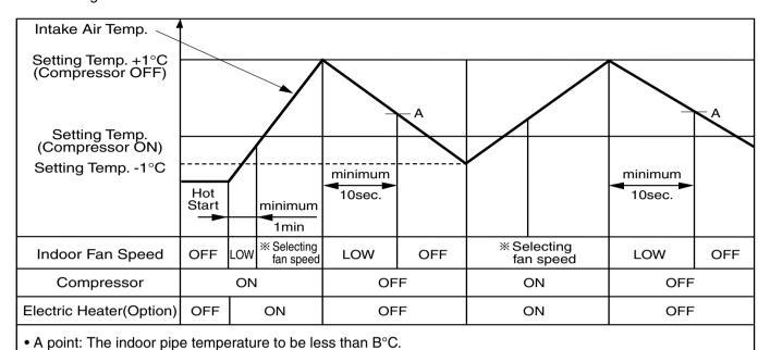
The indoor fan operates for minimum 10sec. even if the indoor pipe temperature falls lower than B°C.
