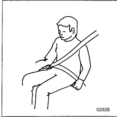
Improperly worn belt
