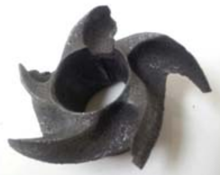
Impeller damaged from high acid solution
