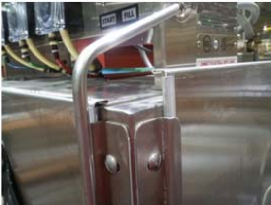
Showing misaligned arms
