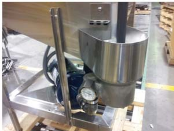
Showing AF-ES sump, drain ball, thermometer
