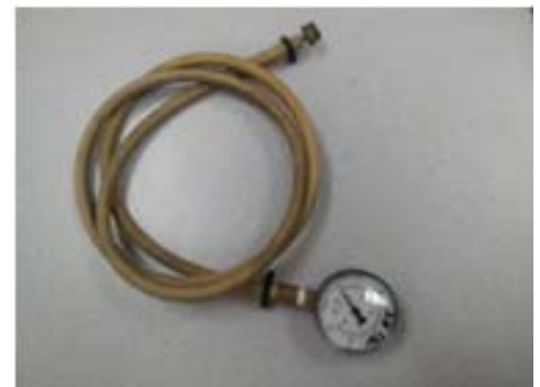
Spray arm pressure tester #088-1048
