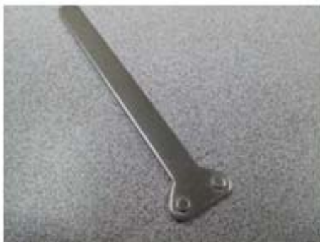
Cam timer adjustment tool
