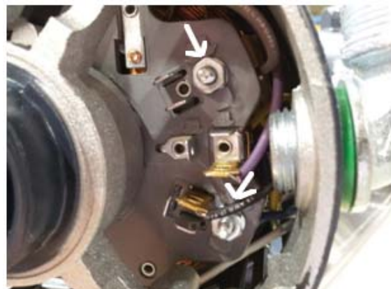
Line connection spades for L1, Neu (arrow 1 & 2)
