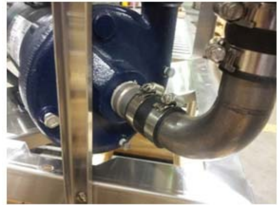
Pump intake and connector sleeves with clamps
