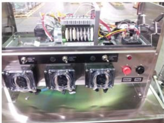
Showing control box, chemical pumps, prime switches
