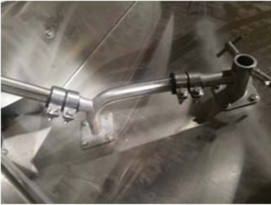
Showing first cycle run without spray arm in spray bases
