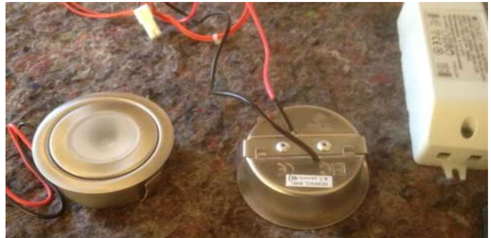
New lamps and transformer
