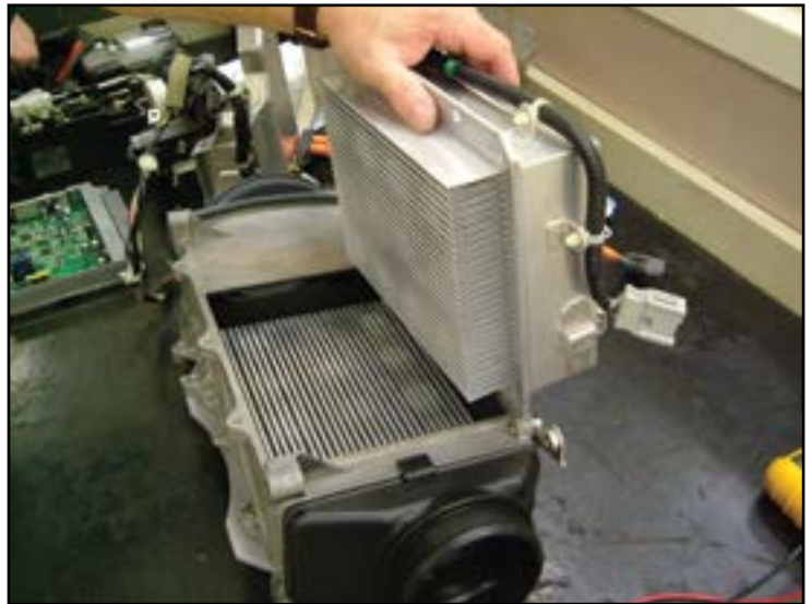
Honda DC-DC Converter uses forced air and cooling fins.
