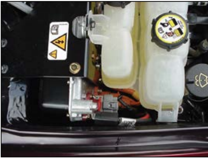
DC-DC Converter is liquid cooled on Ford Escape 2005 - 2012.
