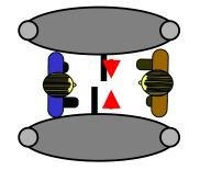
When an unauthorised person is standing in the Speedlane and a second person is approaching from the same direction, the second person can be authorised. The first person has to leave the Speedlane at the side the other person is approaching to allow the second person to pass. When the unauthorised person does not step out, this person can pass the door wings using the authorisation of the second person. The second person then needs to be authorised again to be able to pass the Speedlane.
