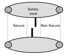
A person is given authorisation by presenting a proximity card to the access control system or when the push button is pressed (depending on the authorisation system chosen). When an authorised person enters or is already in the Secure (Non-Secure) zone, the door wings will open. After the person has passed the safety zone, the door wings will close immediately. When no one passes through the Speedlane, the door wings will close after 8 seconds (maximum authorisation time).
