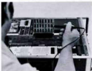
**STEP 2.** Test for an open output bond driving the failing node using the Logic Probe. If an open output bond is indicated, replace the IC driving the failing node.
