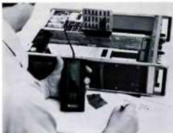
**STEP 1.** Test all IC's using the Logic Comparator or Logic Probe, Pulser and Clip and note the failing nodes.
