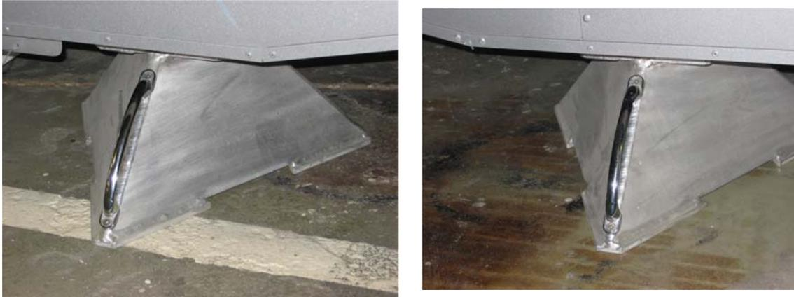
**Figure 32: Rear Stabilizing Stands**
