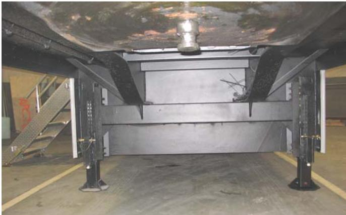
**Figure 17: Front Stabilizing Legs and Auxiliary Support Legs**
