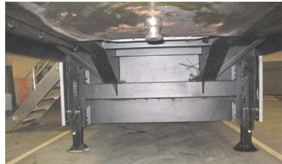
**Figure 31: Front Stabilizing Leg Assembly**
