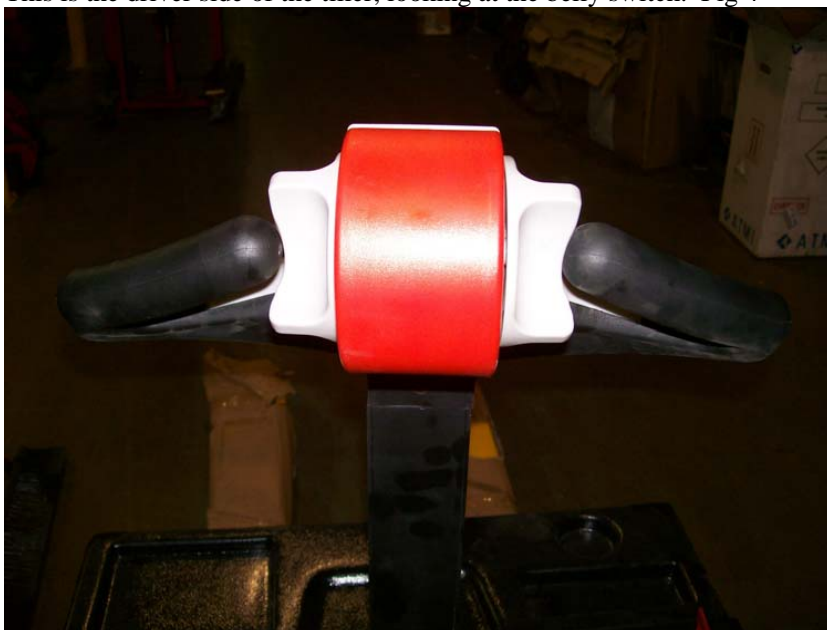
This is the driver side of the tiller, looking at the belly switch. Fig 4
