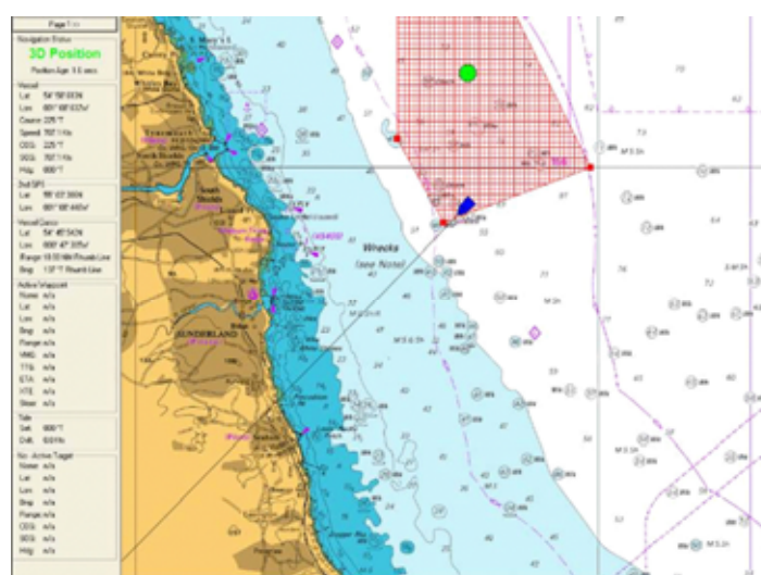
Figure 2: A screen shot of the modified electronic chart showing two positions reported from the demonstration vessel. The green dot is the eLoran position and shows the true location of the vessel within the jamming area (red hatched box). The blue vessel icon is the erroneously reported GPS position. The line emerging from the icon is an indication of the reported speed, which was given as over 700 knots.
