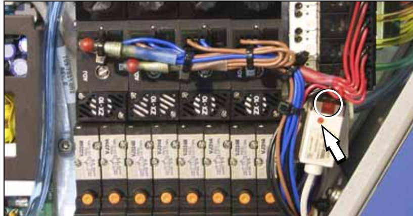
Figure 17—Adjusting the Low Pressure Sensor on the Pneumatic Module. The arrow points to the adjustment screw. The LED is circled.
