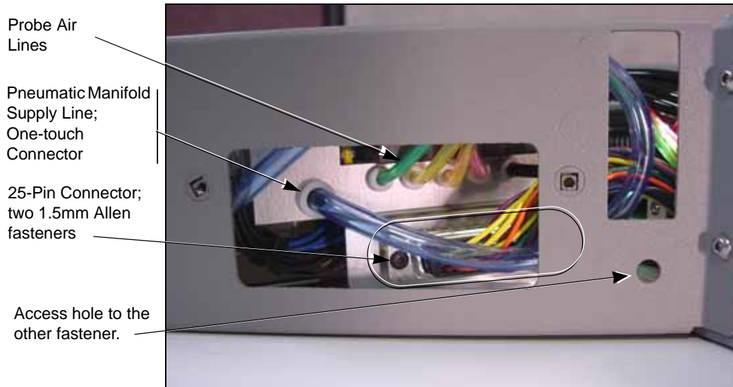
Figure 15—Location of the Pneumatic Manifold Supply Line and Wiring Connector
