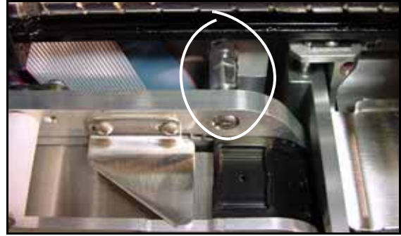
Figure 9—Some Tape-In Modules have an Adjustable Standoff for setting the Alignment with the Probes. The wrench flats and Locknut identify the Adjustment Stud from a non-adjustable Standoff.
