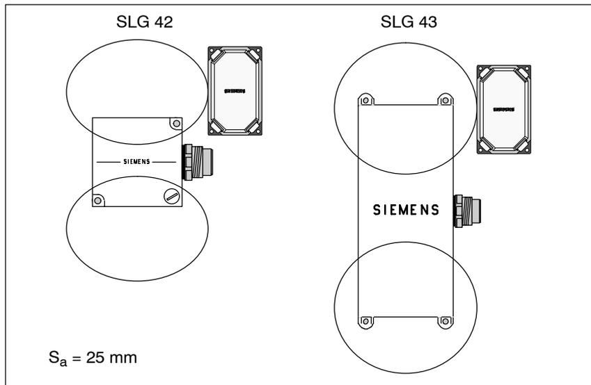
Figure 3-30 Transmission window of the MDS 507 with dead battery
