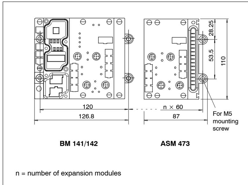
Figure 6-47 Dimensions for mounting holes for basic and expansion modules.
