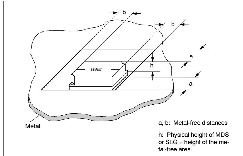
Figure 3-16 Flush installation
