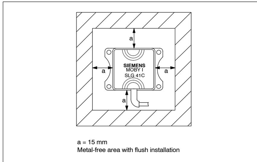
Figure 5-20 Metal-free area of SLG 41C/41CC
