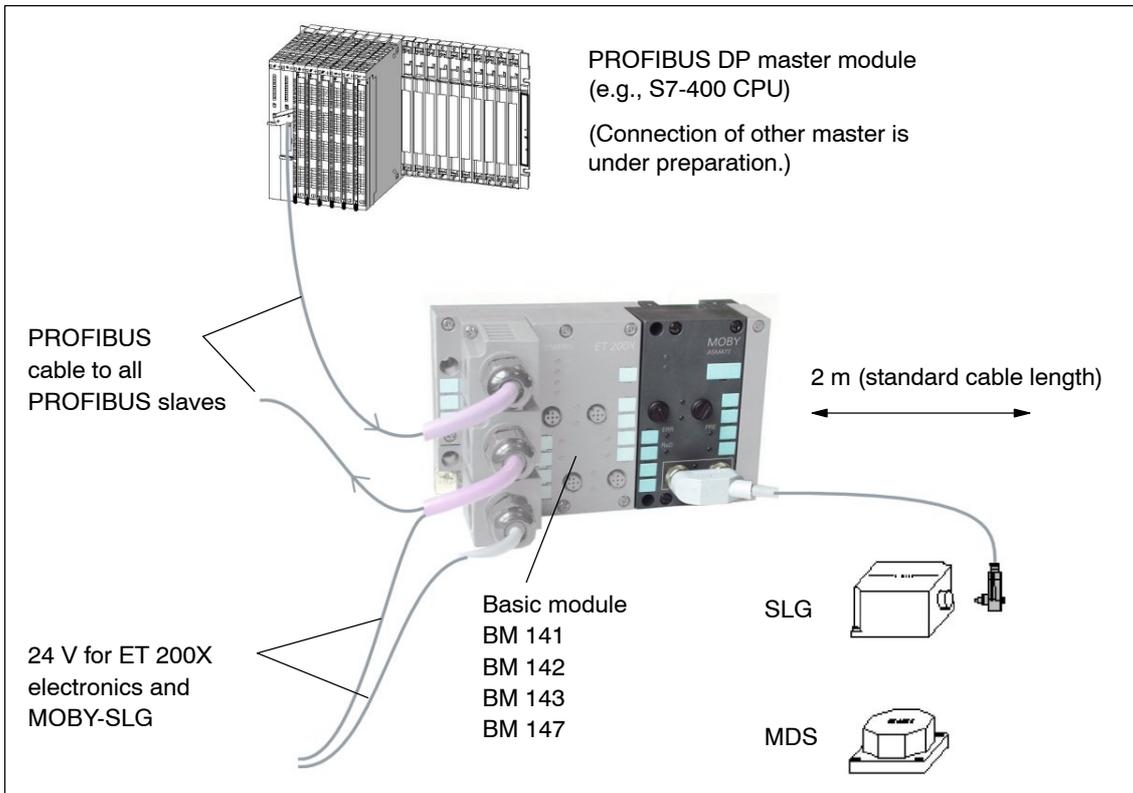
Figure 6-44 Configurator for an ASM 473
