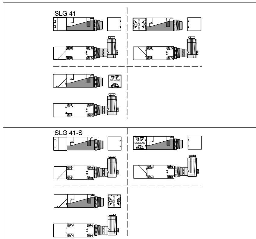
Figure 5-17 Read head changes of SLG 41/SLG 41-S
