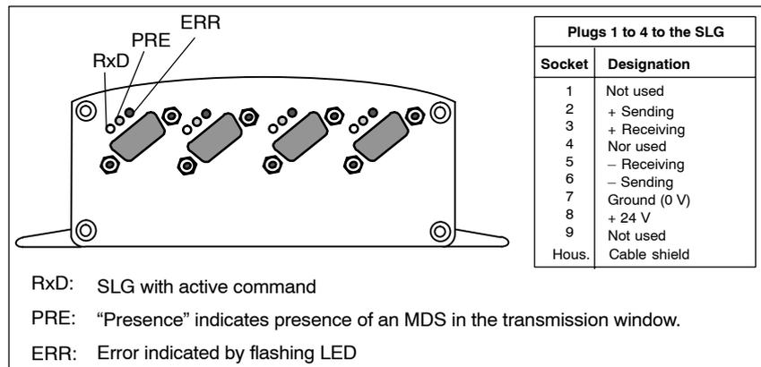
Figure 6-33 Serial interfaces of the ASM 454/424 to the SLG
