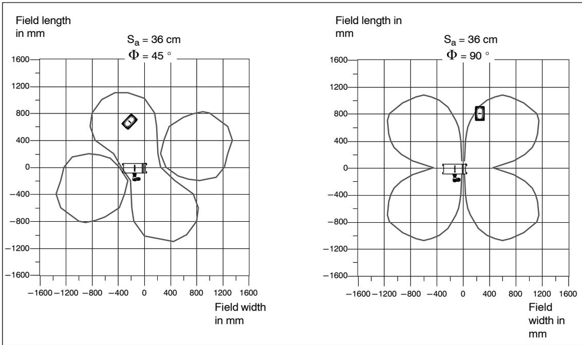
Figure 3-29 Switch-on window with various angle deviations
