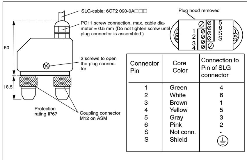
Figure 6-23 Connection plug, ASM 450/452/473 ↔ SLG (6GT2 090-0BC00)
