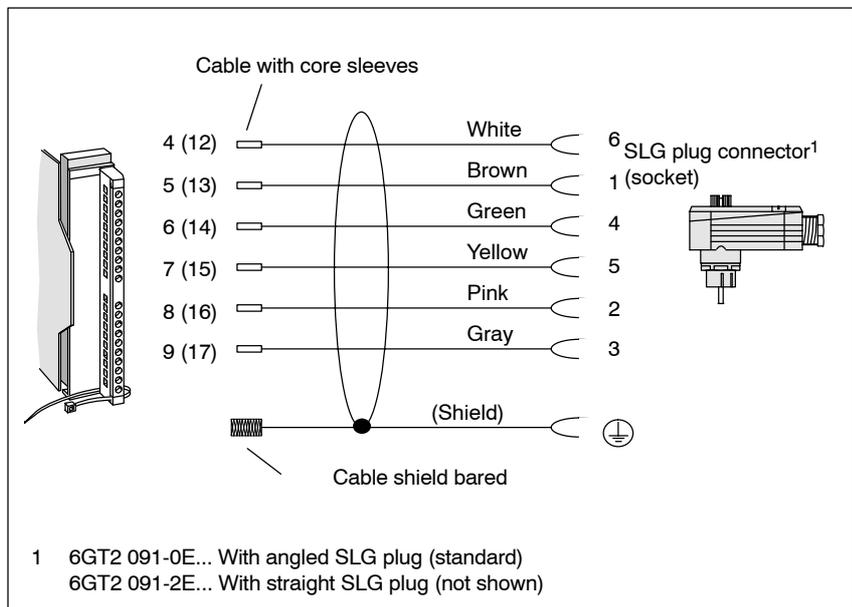
Figure 3-62 Connection cable: ASM 470/475 ↔ SLG
