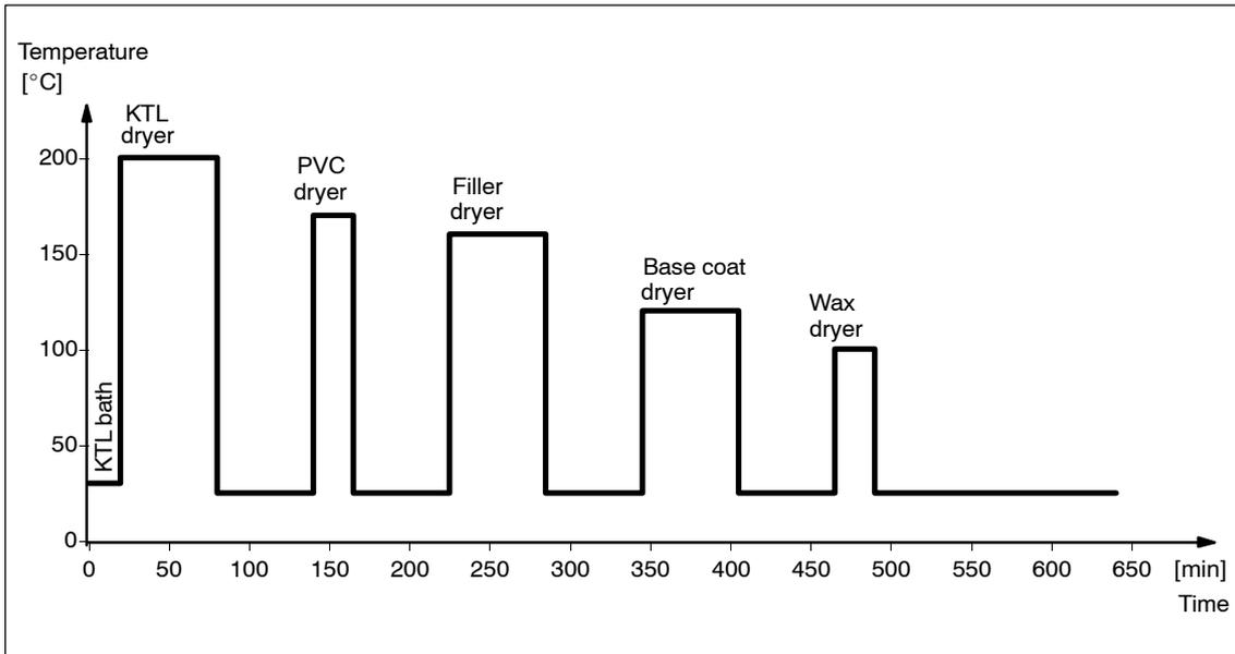
Figure 3-39 Diagram of the temperature progression from table 3-14
