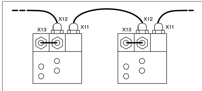
Figure 6-25 PROFIBUS cable with 24 V power
