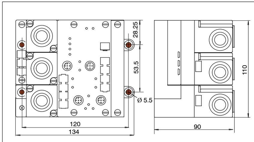
Figure 6-27 Dimensional drawing of the ASM 450/452
