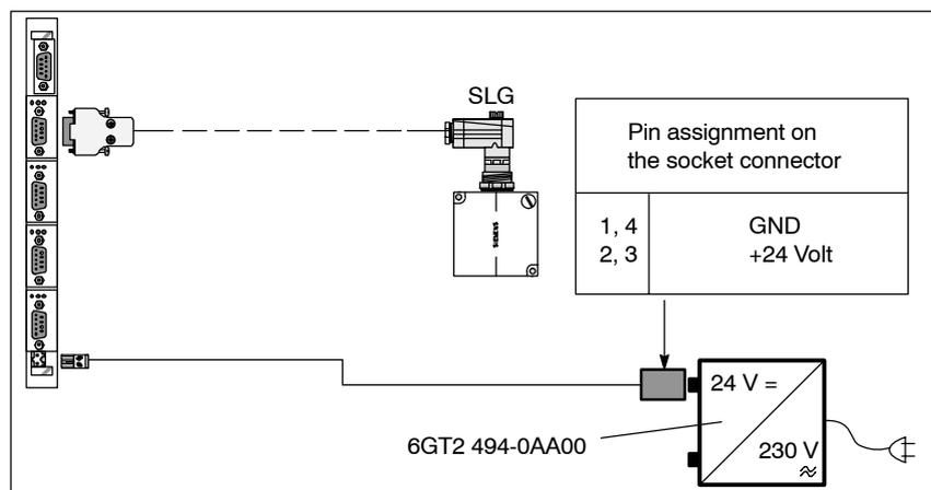
Figure 3-57 MOBY wide-range power pack on the ASM 400
