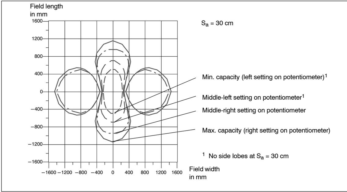
Figure 3-28 Switch-on window for various receiving capacities
