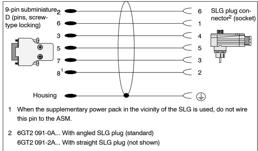
Figure 3-59 Connection cable: ASM 400/401/424/454, ES 030 ↔ SLG
