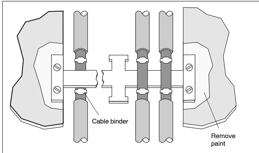
Figure 3-52 Connection of the shield rail
