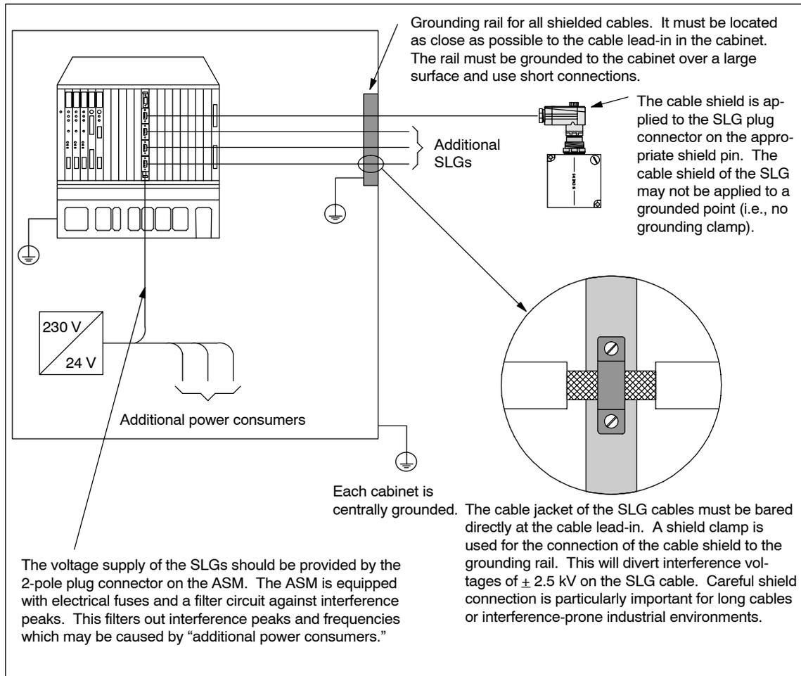
Figure 3-54 Simple layout with ASM 400/401
