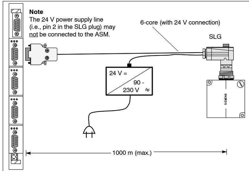
Figure 3-56 SLG with supplementary power pack
