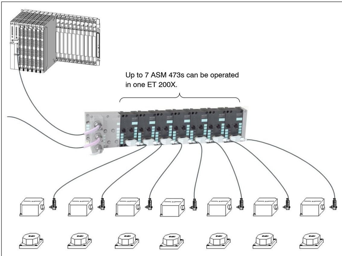
Figure 6-45 Maximum configuration of ASM 473 on an ET 200X
