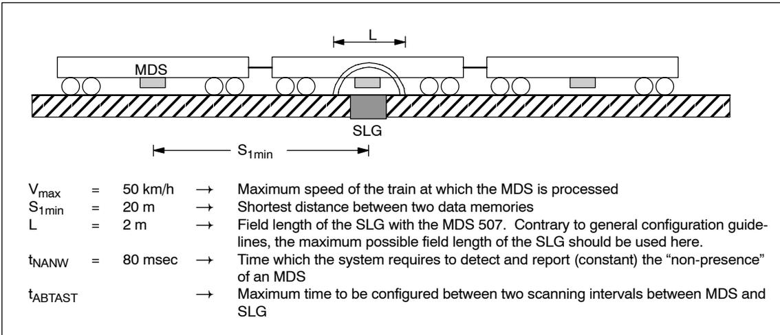
Figure 3-22 Sample configuration of  $t_{ABTAST}$ : Train with several cars
