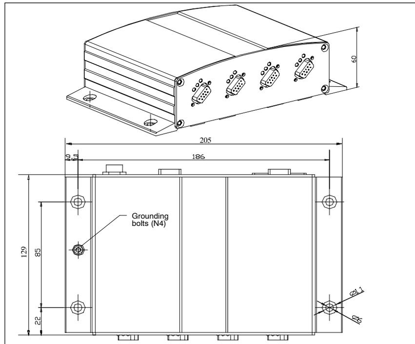
Figure 6-35 Dimensional drawing of ASM 454/424
