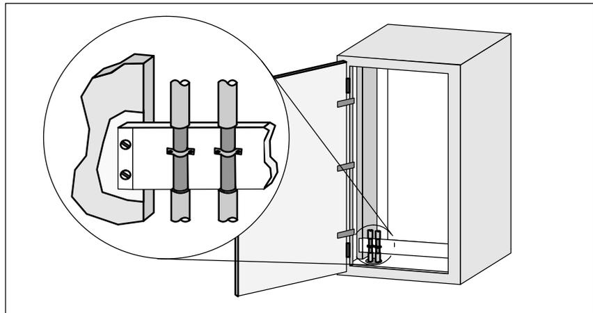
Figure 3-51 Shielding of the cables
