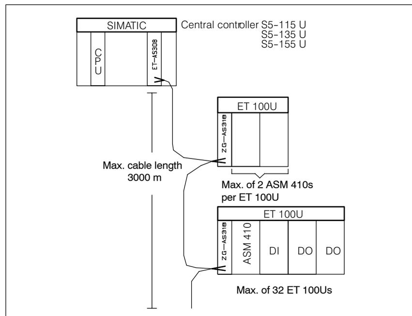
Figure 6-18 Configurator for ASM 410 in ET 100U
