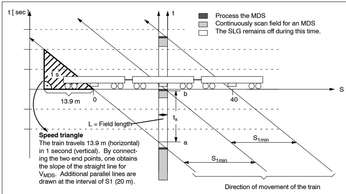
Figure 3-23 Diagram of the configuration (drawn to scale)
