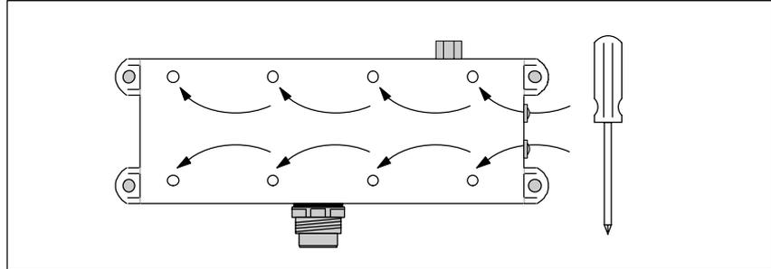
Figure 3-34 Opening the cover of the SLG 44
