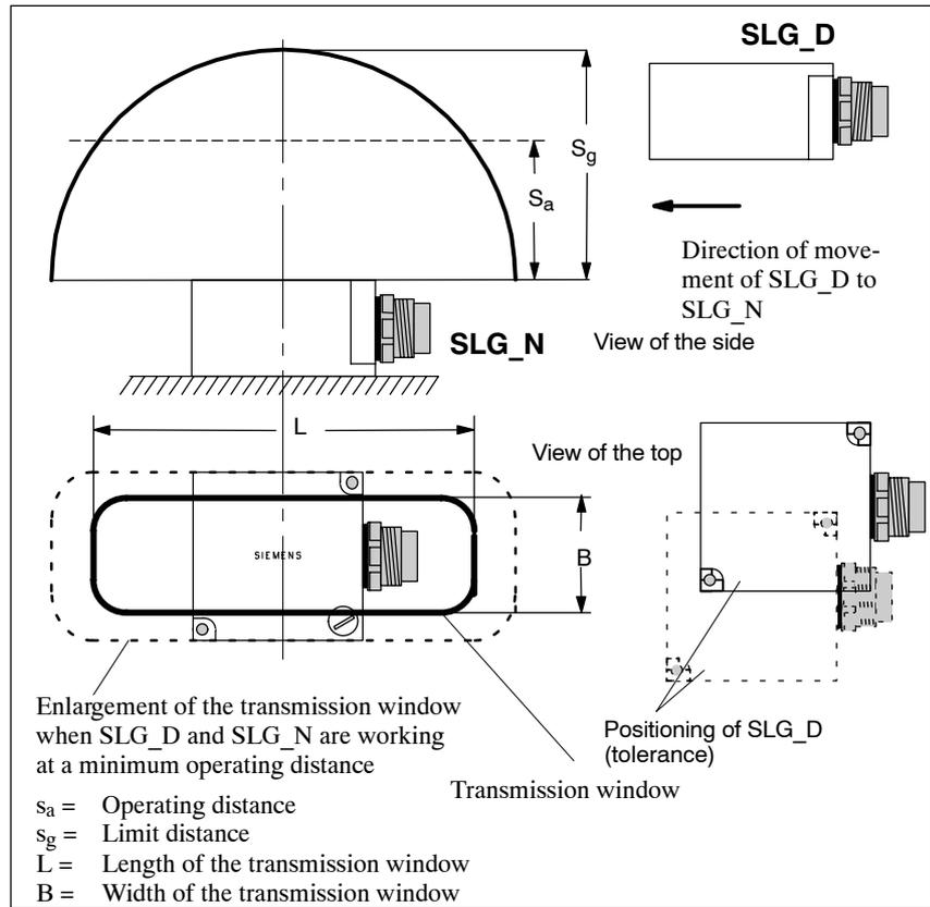
Figure 3-9 Transmission window during dialog
