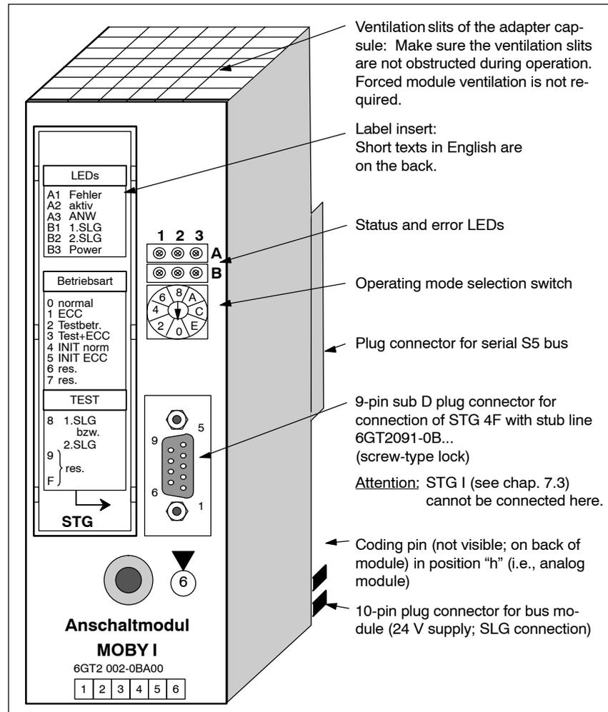
Figure 6-19 ASM 410 interface with operational and indicator elements
