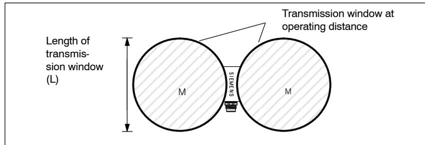
Figure 5-29 Transmission window of SLG 43
