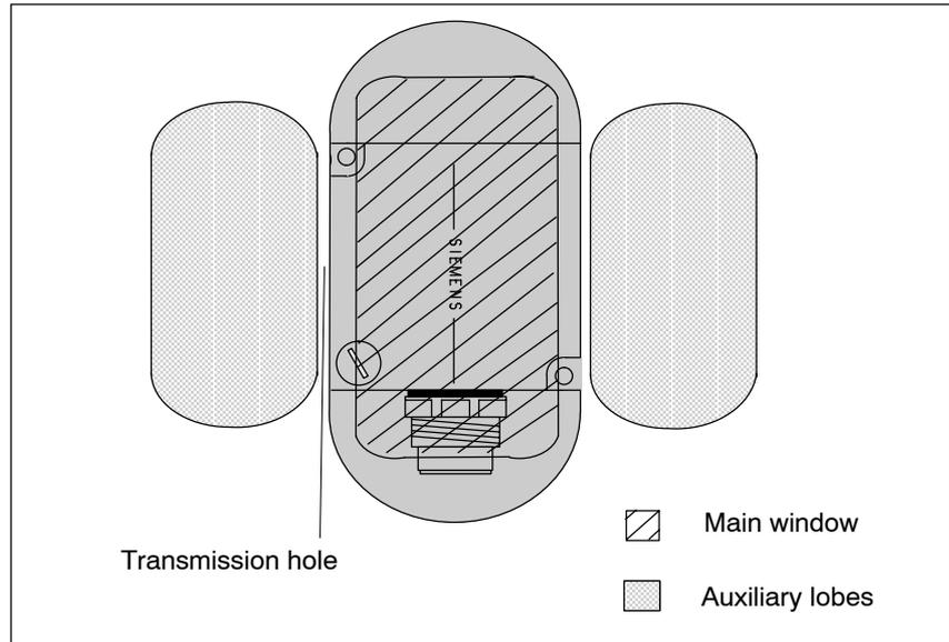
Figure 4-11 Transmission window of the MDS 403 with auxiliary lobes
