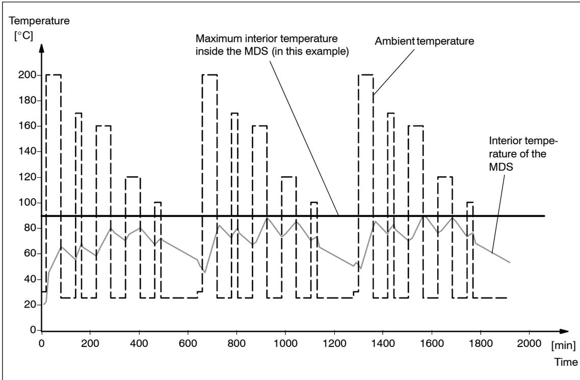
Figure 3-40 Complete temperature progression during simulation
