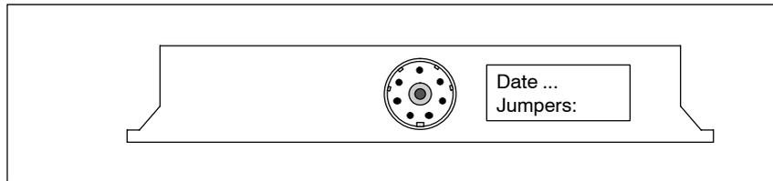
Figure 3-36 Label for identification of the hardware status
