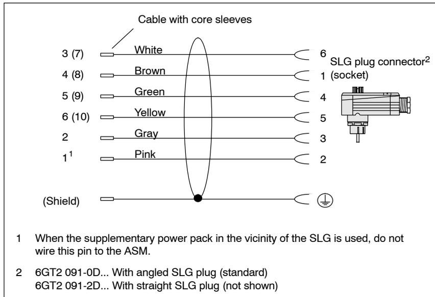
Figure 3-61 Connection cable: ASM 410 ↔ SLG
