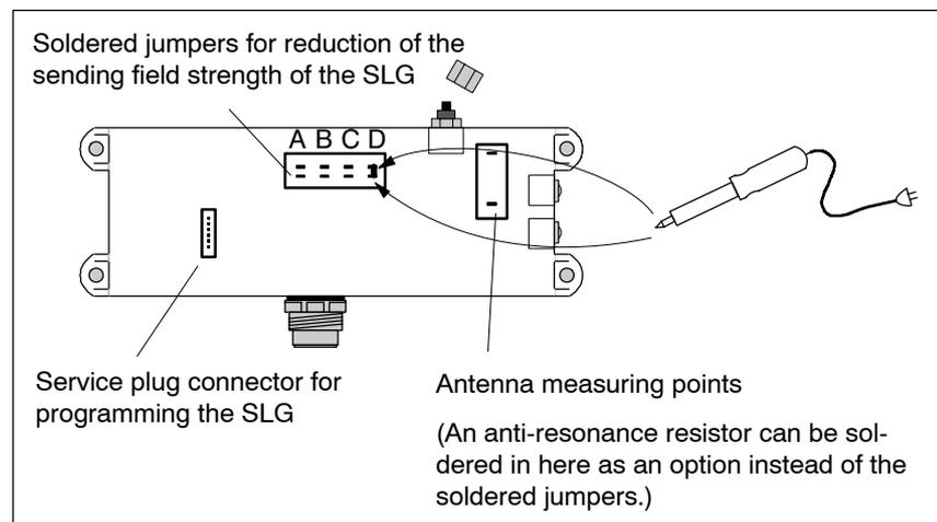
Figure 3-35 Soldered jumpers and antenna measuring points on the SLG 44
