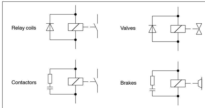
Figure 3-46 Suppression of inductive interference
