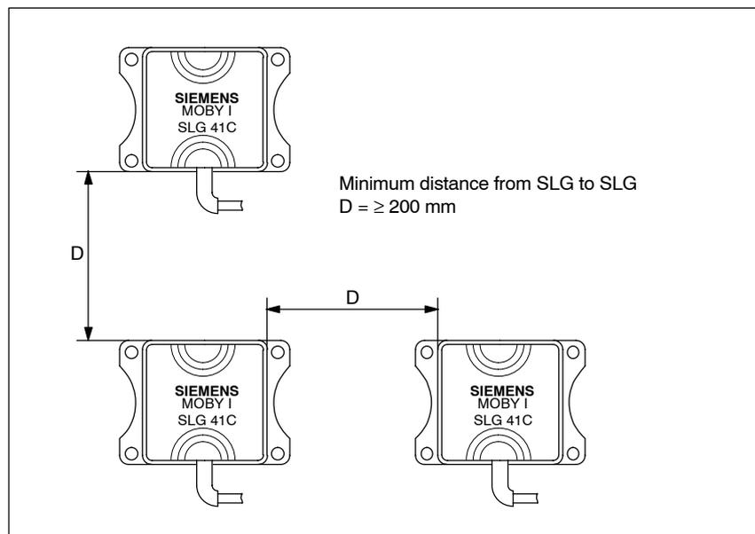
Figure 5-21 Distance D: SLG 41C/41CC
