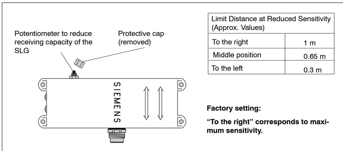
Figure 3-33 Reduction of the receiving capacity of the SLG 44
