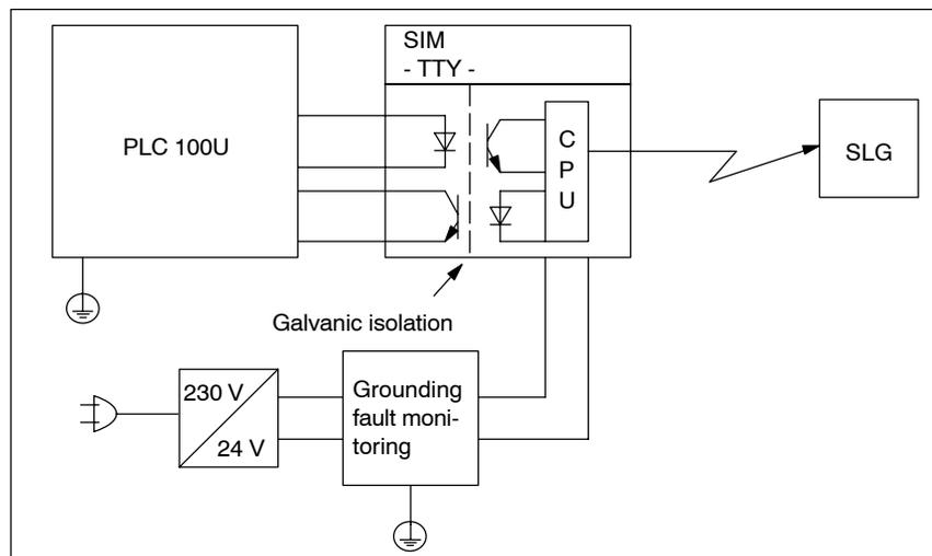
Figure 3-50 Serial interface SIM with TTY interface
