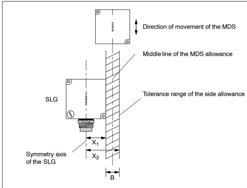
Figure 3-7 Tolerance of the side allowance of the pallet
