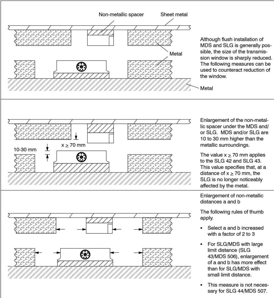
Figure 3-20 Flush installation
