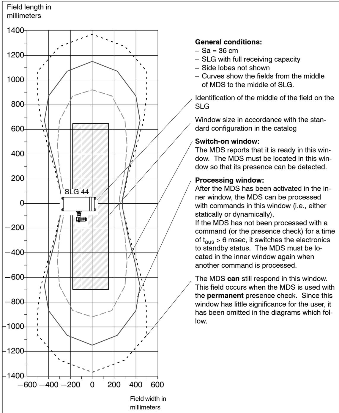
Figure 3-25 Real transmission window between the MDS 507 and the SLG 44
