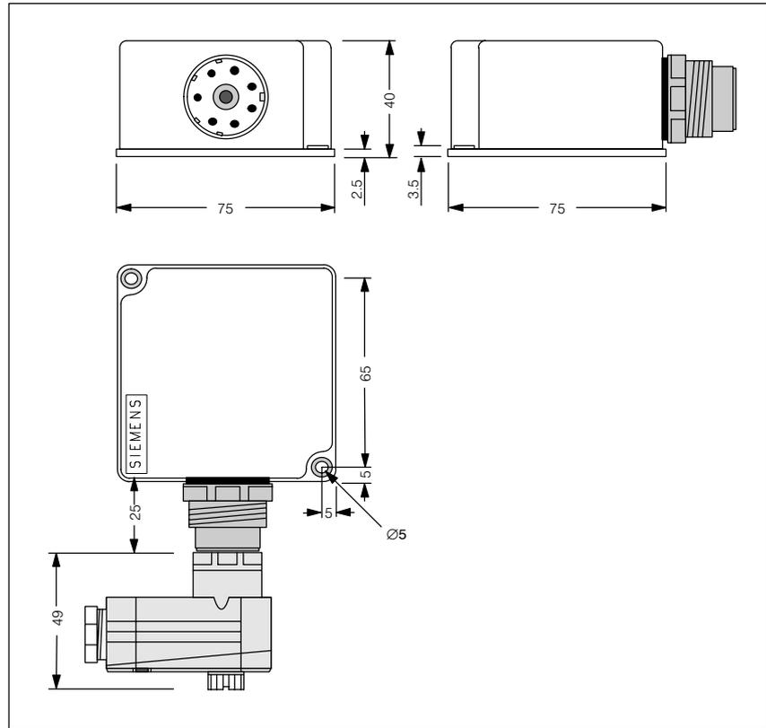
Figure 5-27 Dimensional diagram of SLG 42
