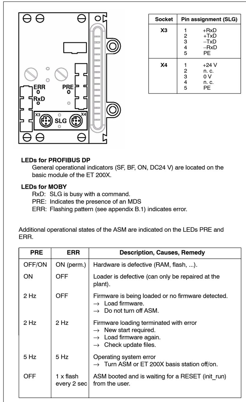
Figure 6-46 Pin assignment and LEDs of ASM 473
