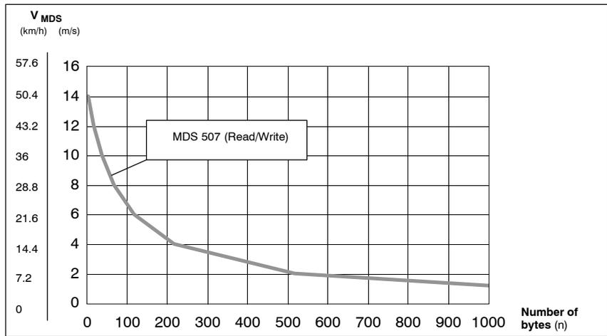
Figure 3-13 SLG 44 (data quantity at low speed)
