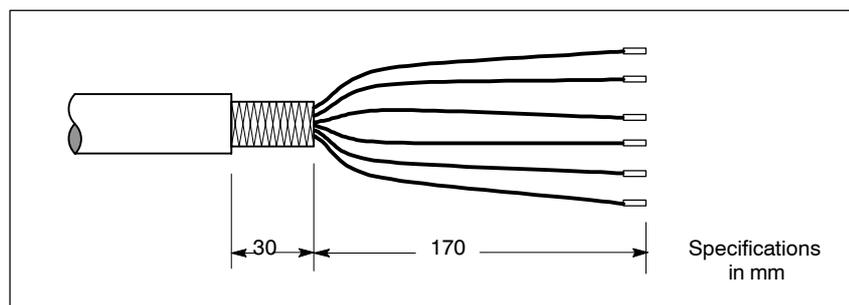
Figure 6-41 Baring of the cable shield when customer makes own cable
