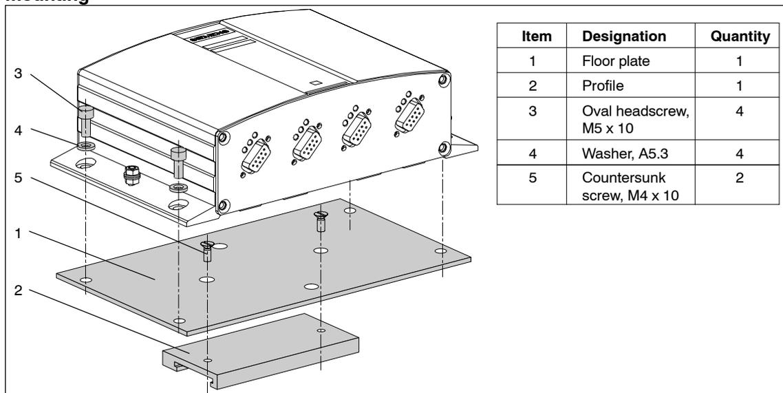
Figure 6-36 Mounting diagram for the adapter floor plate
