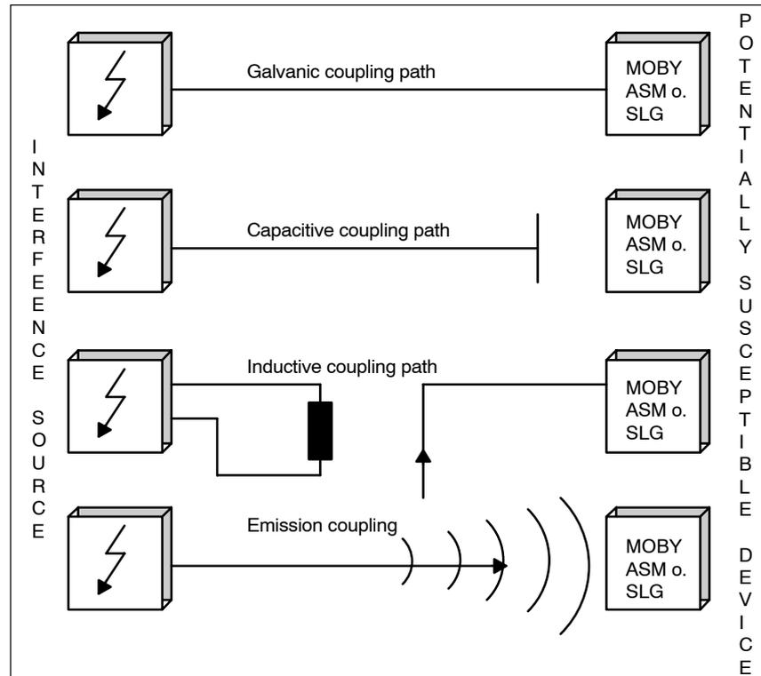
Figure 3-42 The four kinds of interference coupling
