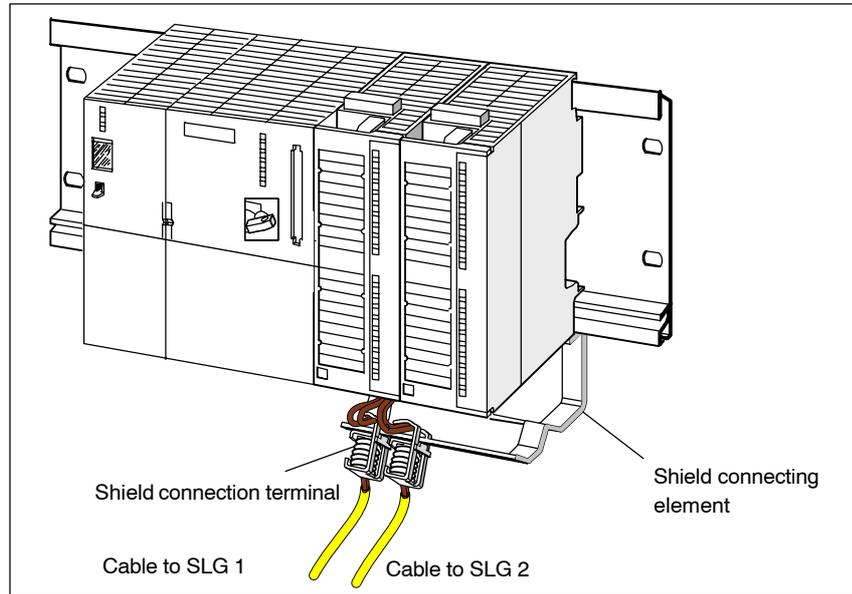
Figure 3-55 Layout of the ASM 470/475 with shield connecting element
