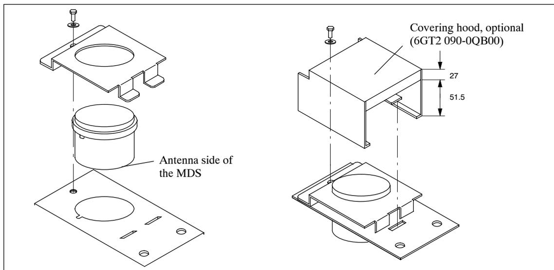
Figure 4-23 Assembly of MDS 439 E with holder
