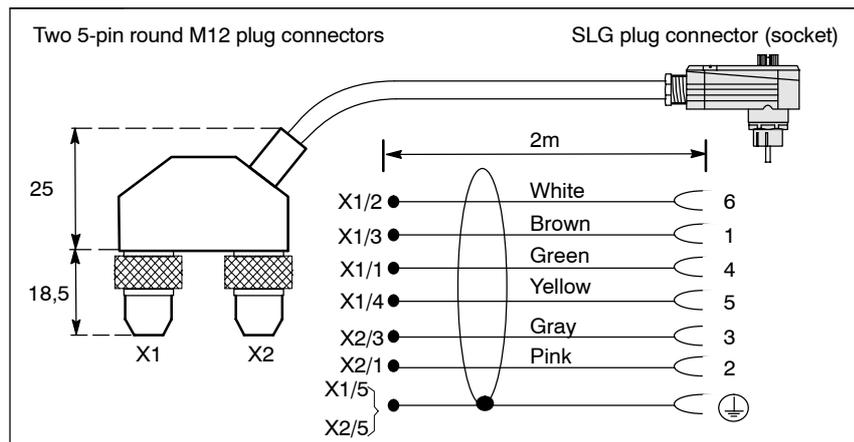
Figure 3-60 Connection cable: ASM 450/452/473 ↔ SLG
