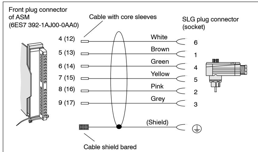
Figure 6-40 Wiring of ASM 470/475 to SLG (6GT2 091-0E...)
