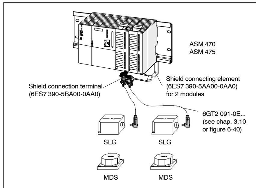
Figure 6-38 Configurator for ASM 470/475
