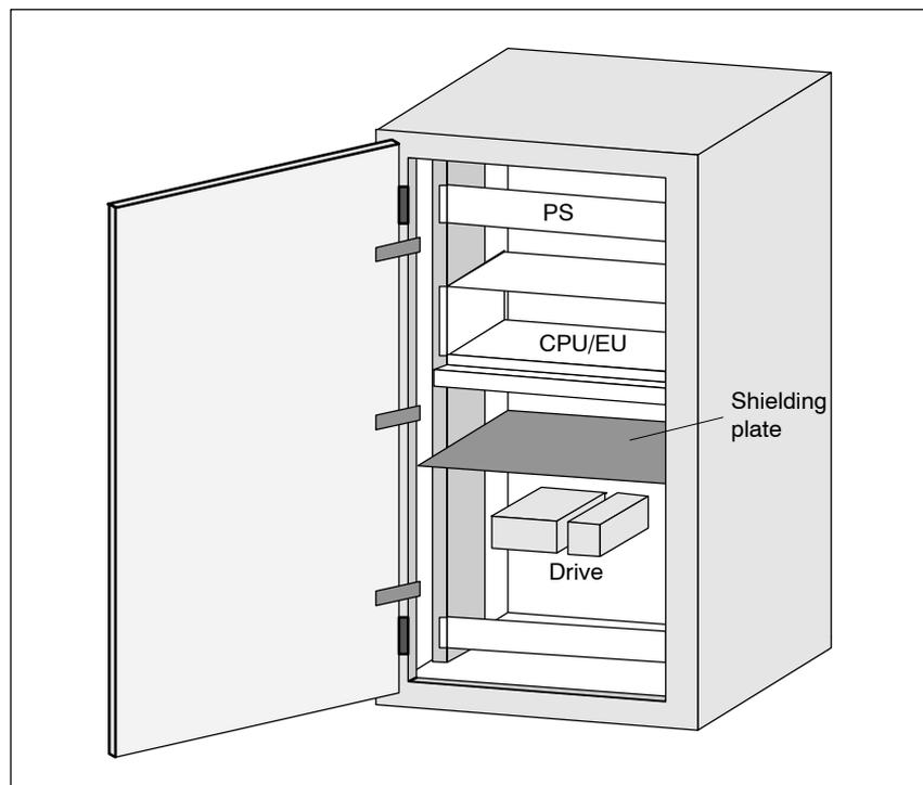
Figure 3-44 Avoidance of interference via optimal layout
