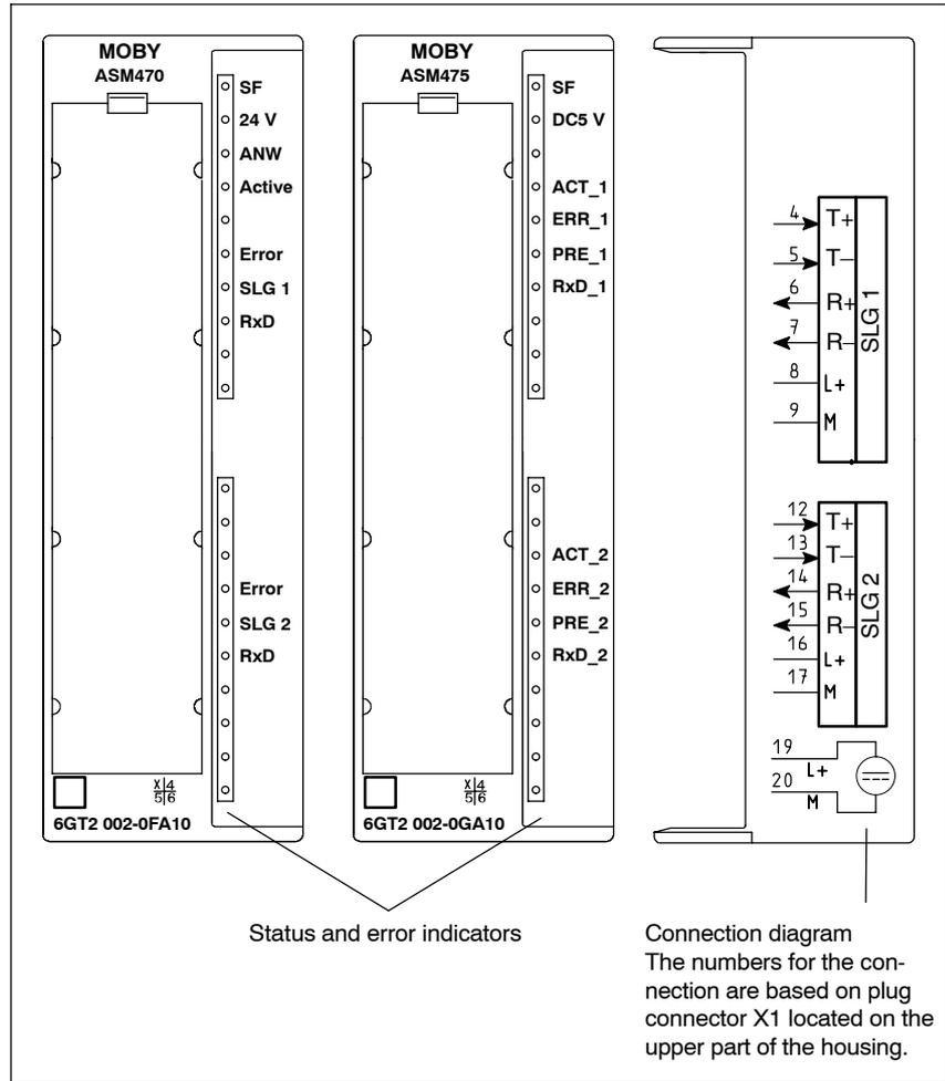
Figure 6-39 Front plate and inside of the front door of the ASM 470/475
