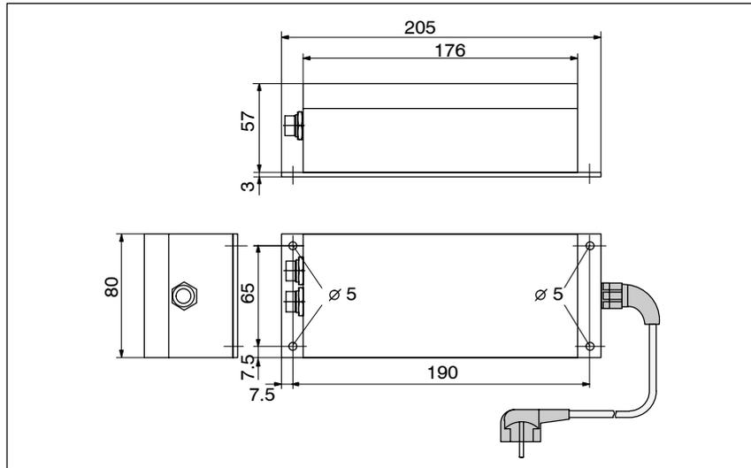
Figure 7-3 Dimensions of MOBY wide-range power pack
