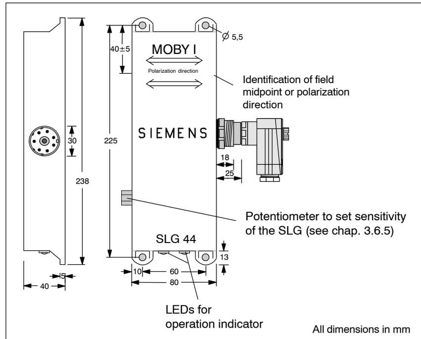
Figure 5-37 Dimensional diagram of SLG 44
