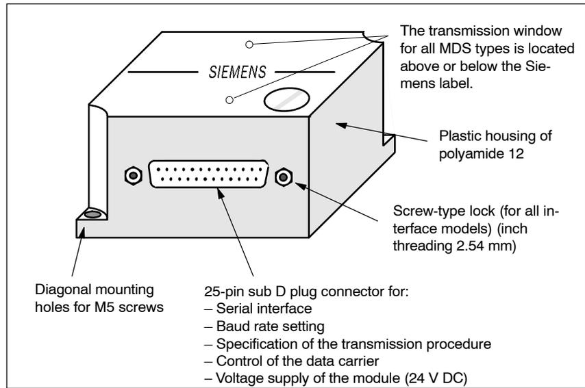
Figure 6-49 SIM serial interface module
