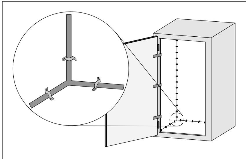
Figure 3-43 Shielding via housing
