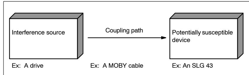
Figure 3-41 Spreading of interference
