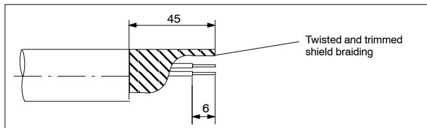
Figure 6-29 Length of baring for a PROFIBUS cable
