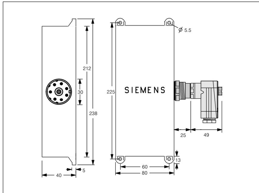
Figure 5-32 Dimensional diagram of SLG 43
