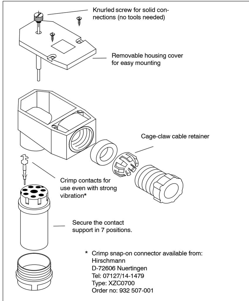
Figure 3-58 Drawing of mounting the SLG plug connector
