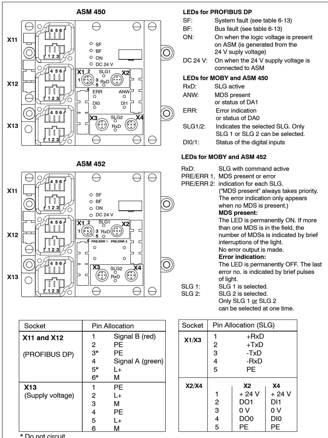
Figure 6-28 Pin allocation and LEDs of ASM 450/452
