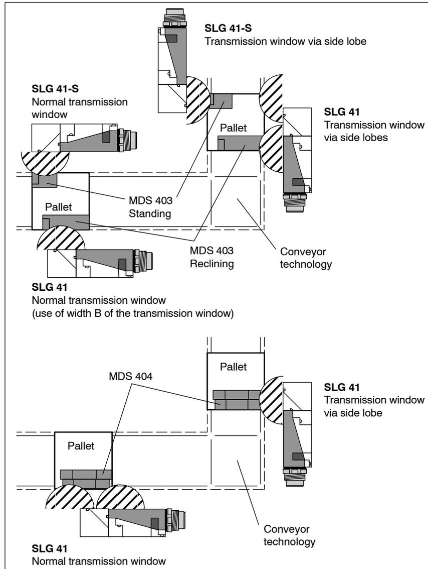
Figure 3-21 Assembly line with MDS 403 reclining or standing (top) and MDS 404 (bottom)
