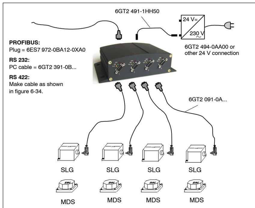
Figure 6-32 Configurator for ASM 454/424
