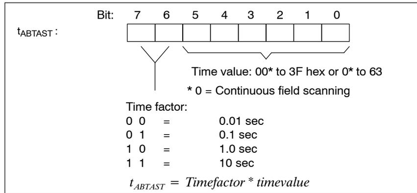
Figure 3-24 Coding for  $t_{ABTAST}$
