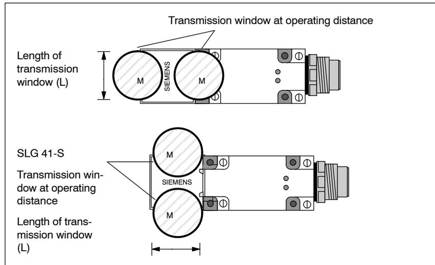
Figure 5-13 Transmission window of SLG 41/SLG 41-S
