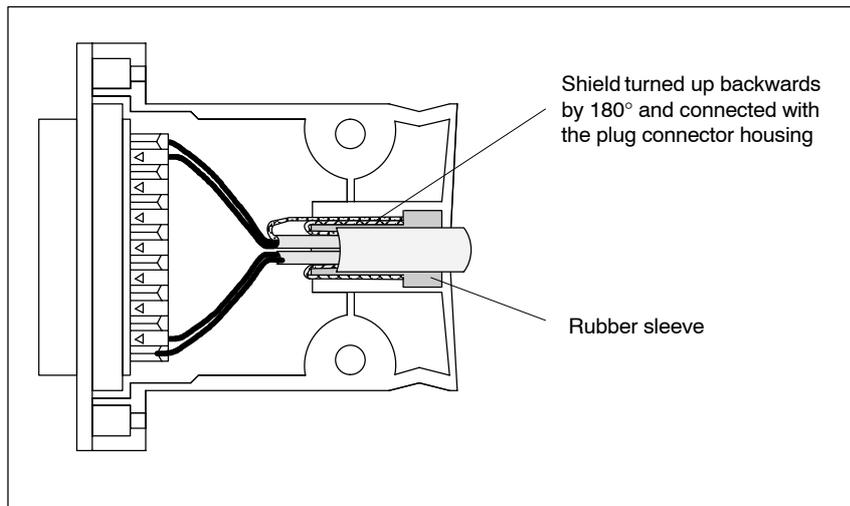
Figure 3-53 Interruption of shielded cables
