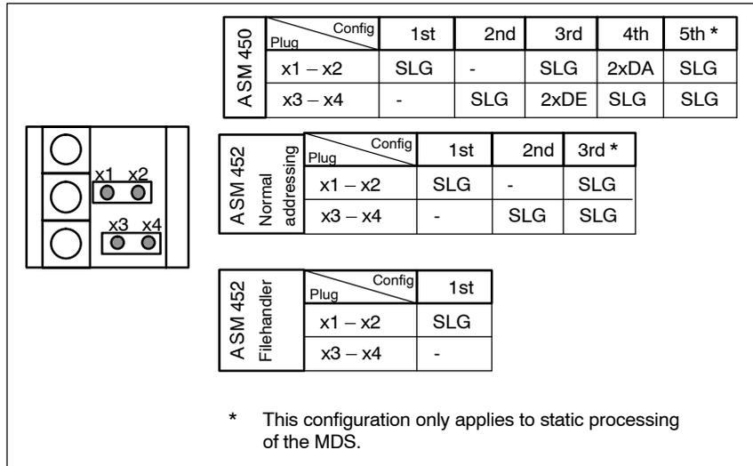
Figure 6-26 SLG and DI/DO configuration for ASM 450/452
