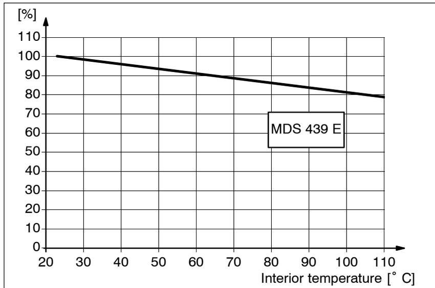
Figure 3-38 Reduction of field length and limit distance
