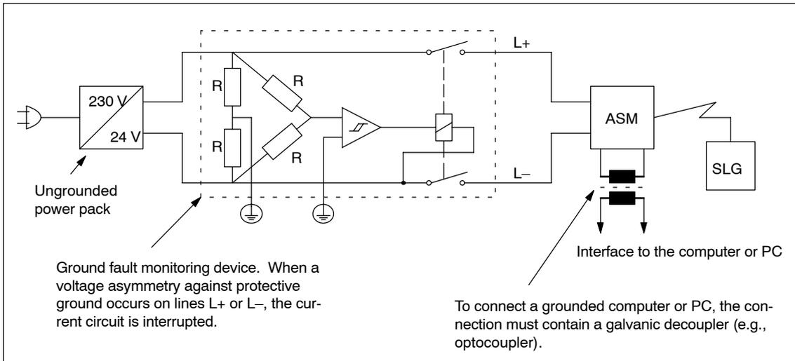
Figure 3-48 Circuit diagram of the principle of grounding fault monitoring
