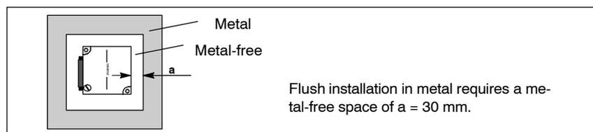
Figure 6-50 Flush installation of SIM in metal
