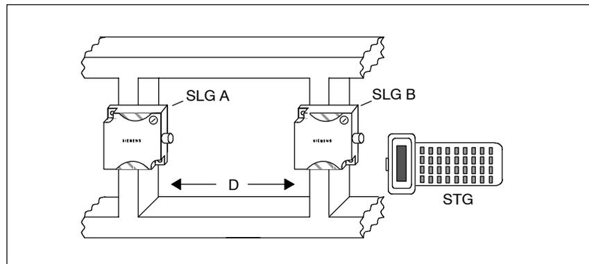
Only SLG A is active. In the vicinity of SLG B, the field is measured on the metal carrier. When an interference field appears on the display, the following measures can be used to correct the situation.
