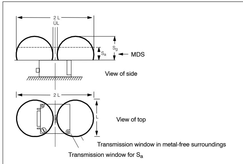
Figure 6-51 Transmission window of SIM
