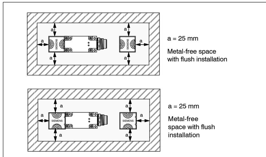
Figure 5-14 Metal-free space for SLG 41/SLG 41-S
