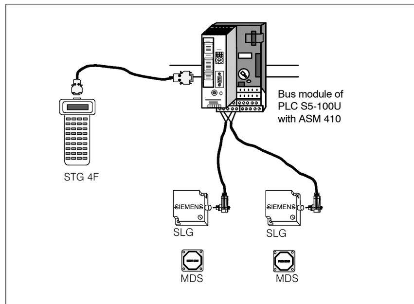
Figure 6-17 Configurator for the ASM 410 in SIMATIC S5
