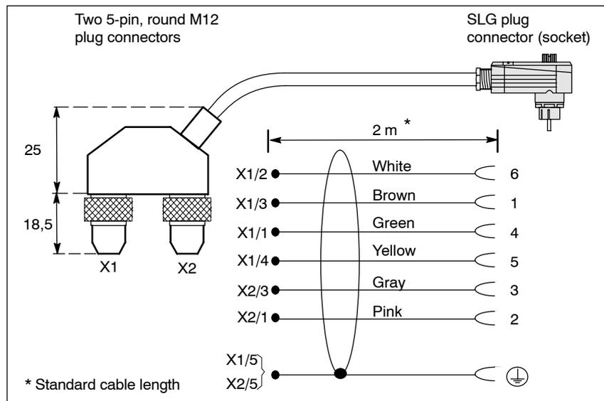
Figure 6-24 Connection cable, ASM 450/452/473 ↔ SLG (6GT2 091-1CH20)
