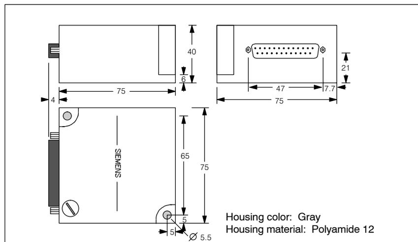
Figure 6-52 Dimensions of SIM serial interface module
