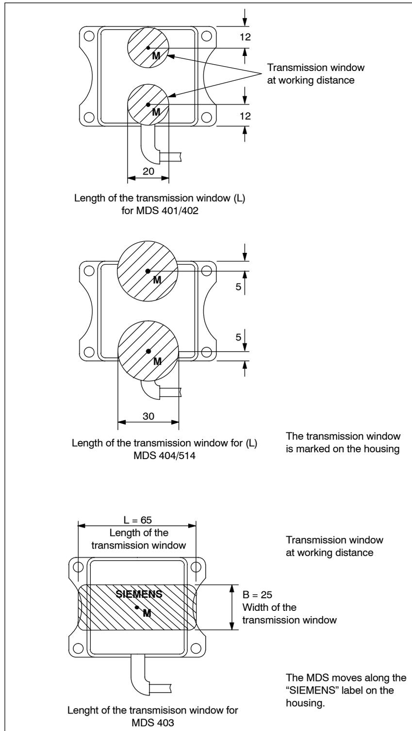
Figure 5-19 Transmission window of SLG 41C/41CC
