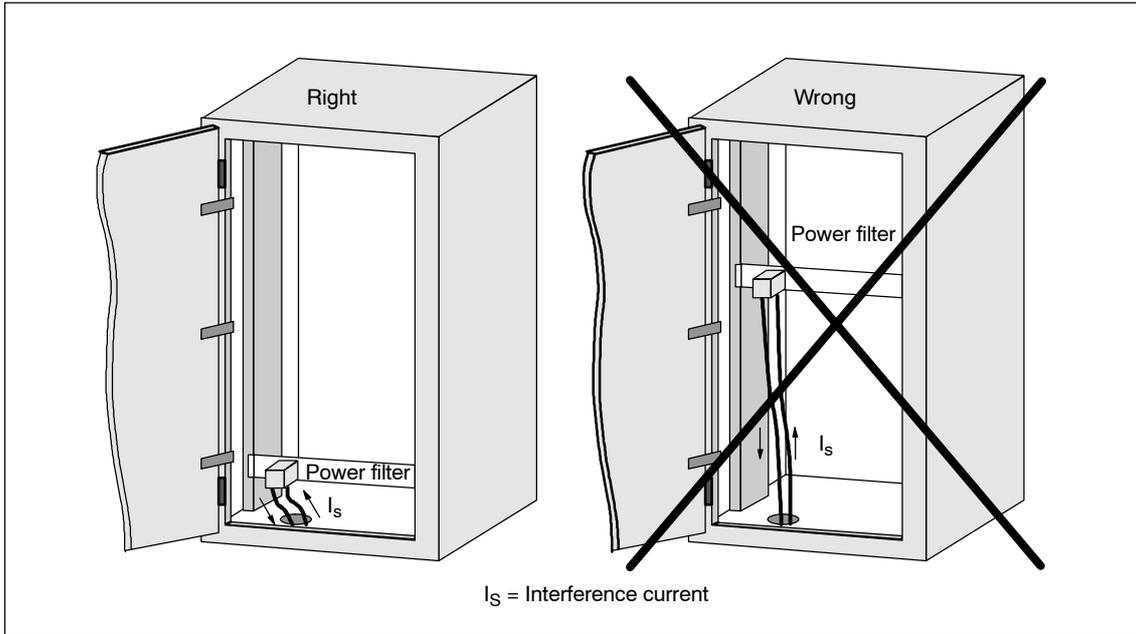
Figure 3-45 Filtering the supply voltage
