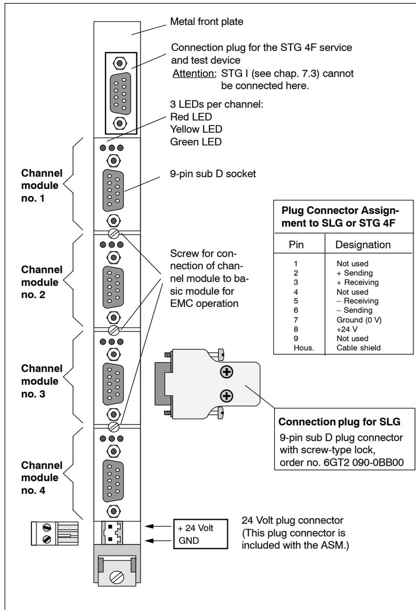
Figure 6-2 Plug connectors and their assignment for ASM 400/401
