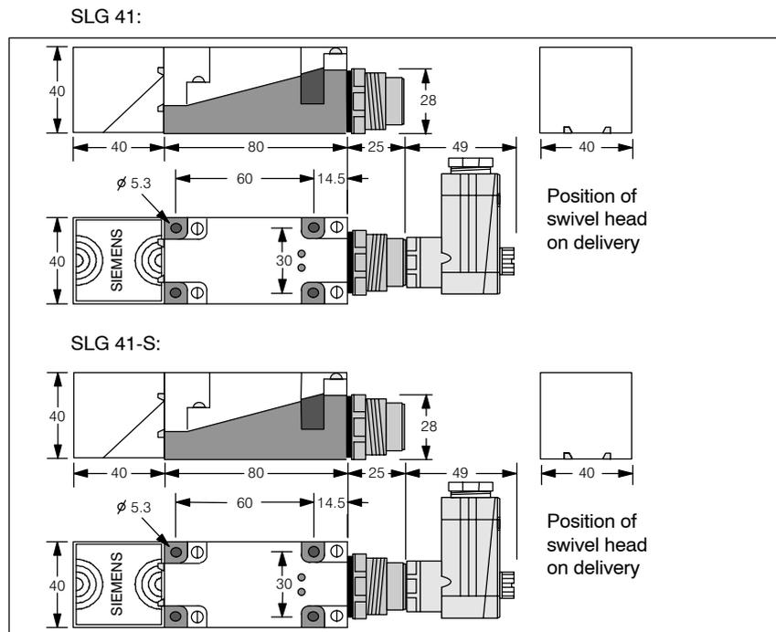
Figure 5-16 Dimensional diagram of SLG 41/SLG 41-S
