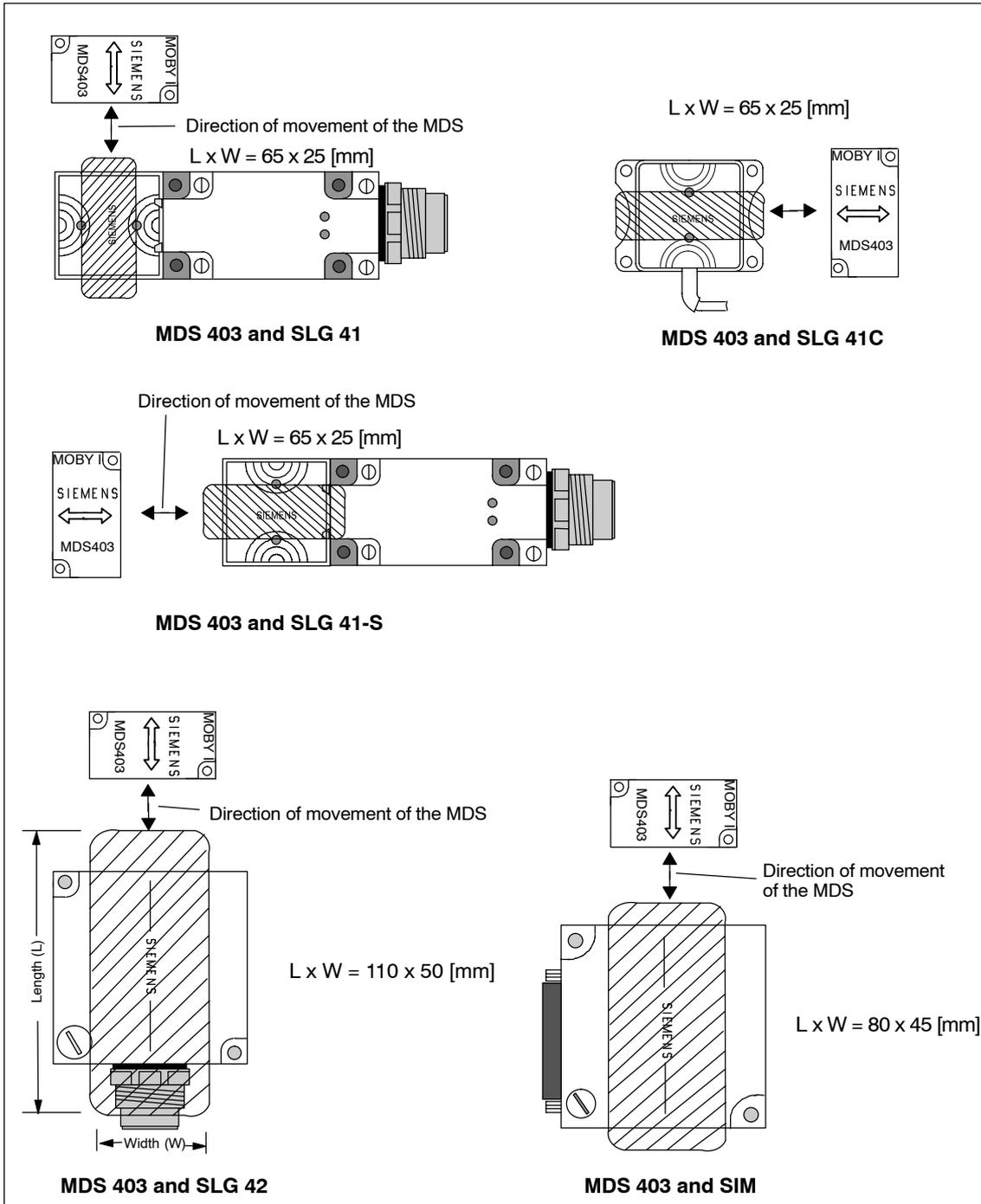
Figure 4-10 Transmission window of the MDS 403
