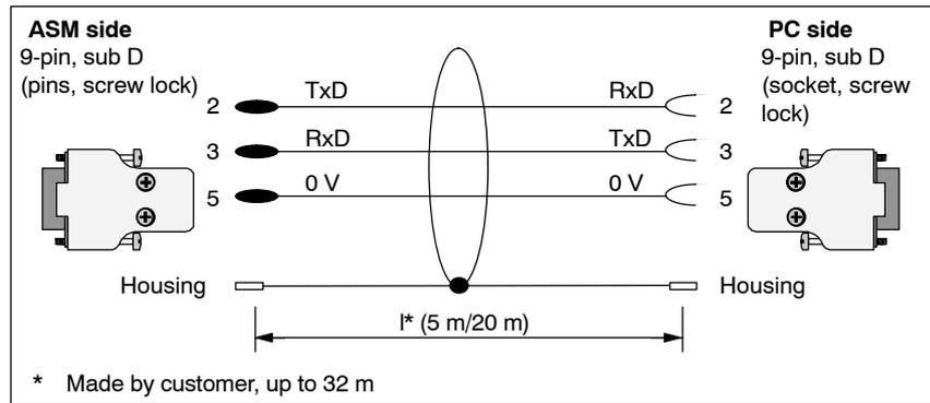
Figure 3-63 Connection cable RS 232 PC ↔ ASM 424
