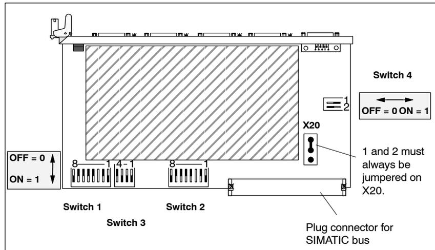
Figure 6-3 Switches and plug-in jumpers for ASM 400/401
