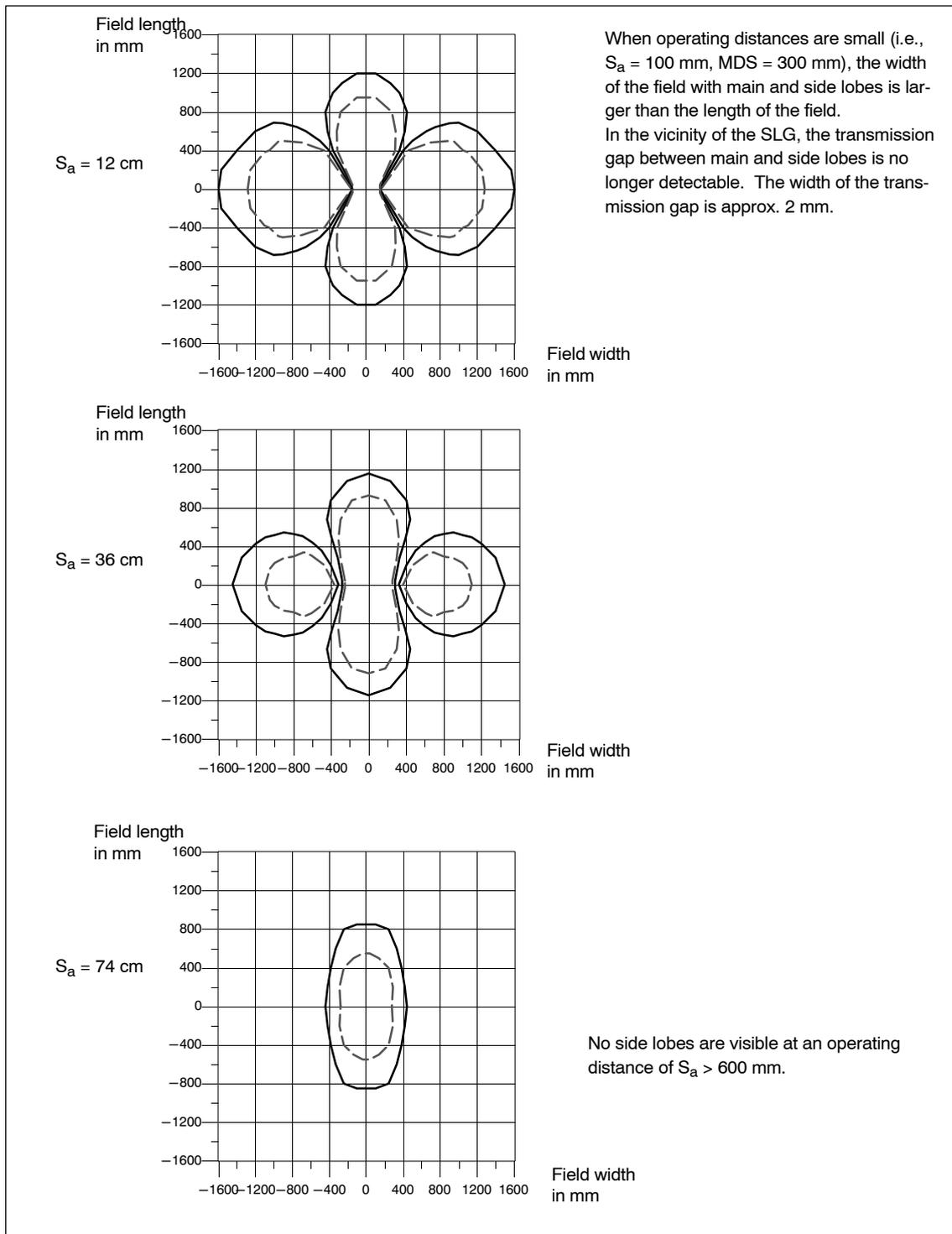
Figure 3-27 Main and side lobes with different operating distances
