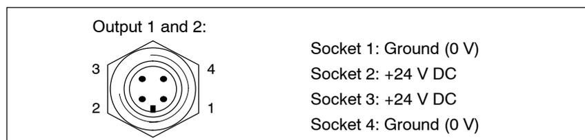
Figure 7-2 Connection assignment of 24 V output
