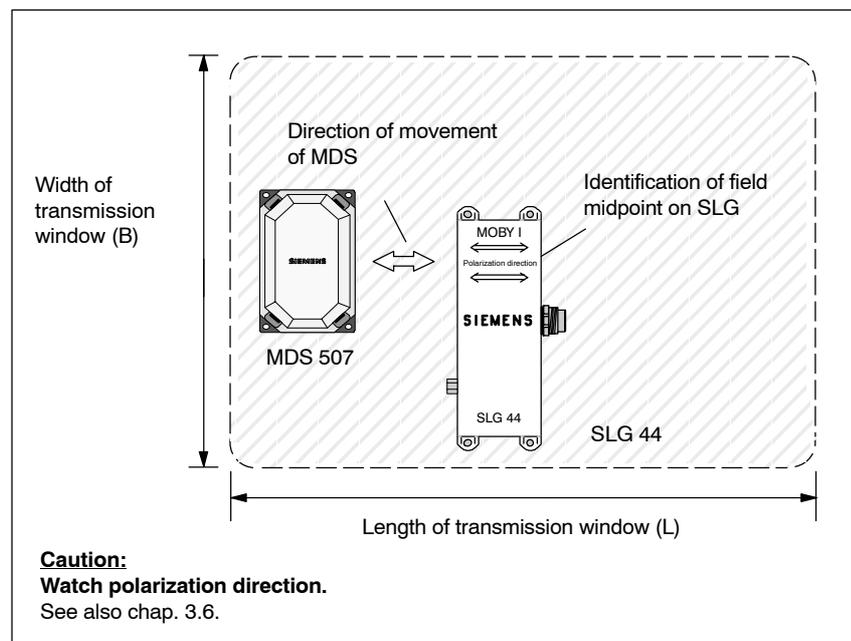
Figure 5-34 Transmission window of SLG 44
