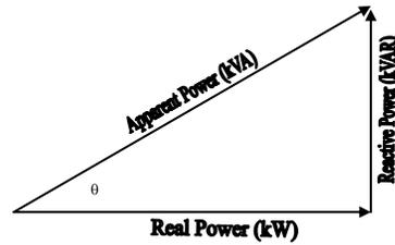
$$3\text{-phase apparent power (kVA)} = \frac{\text{Volts} \times \text{Amps} \times 1.73}{1000}$$
