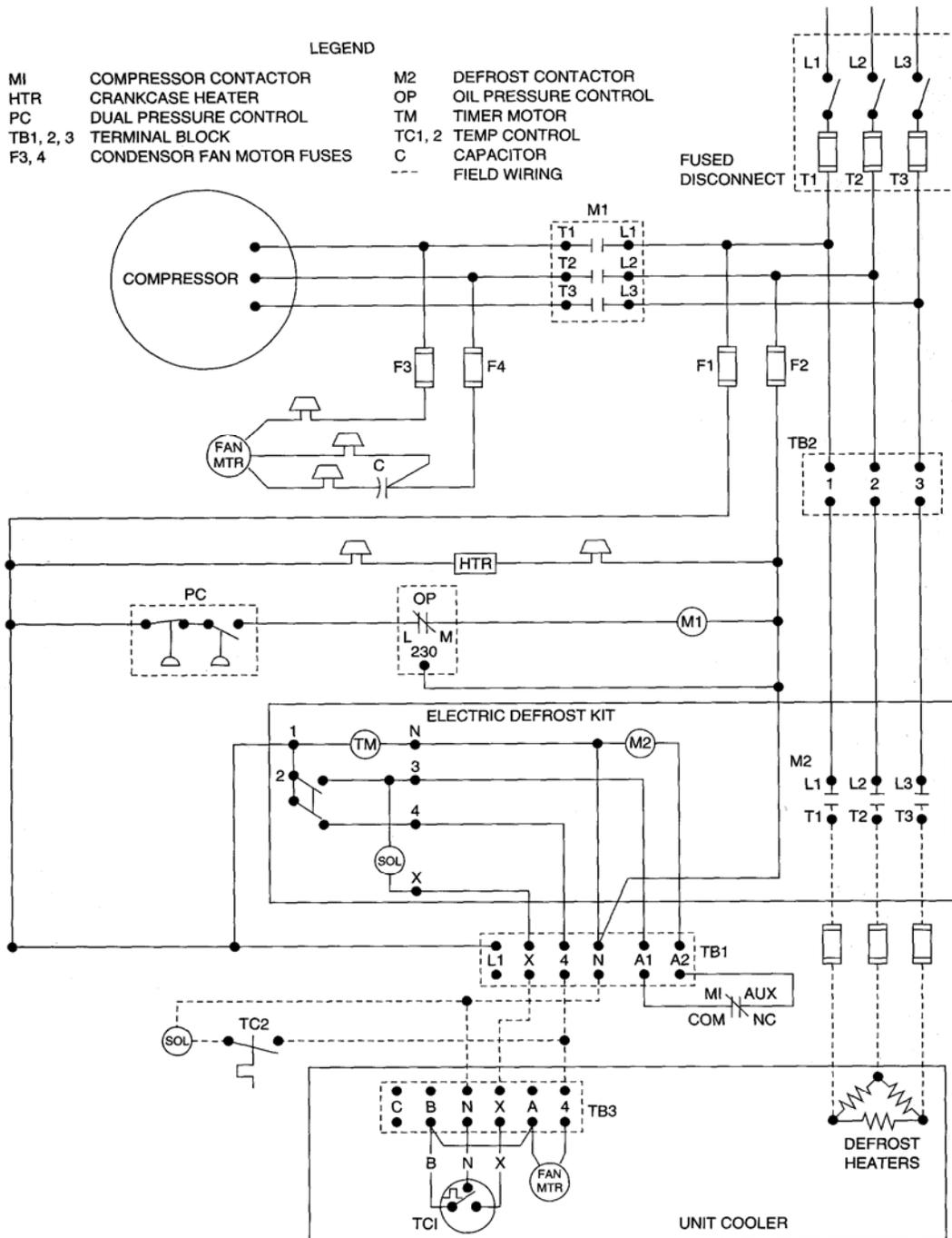
134. The compressor on a walk-in freezer has just restarted after a defrost cycle but the technician notices that the evaporator fans are not operating. What would the first component that the technician would focus on in this situation?
